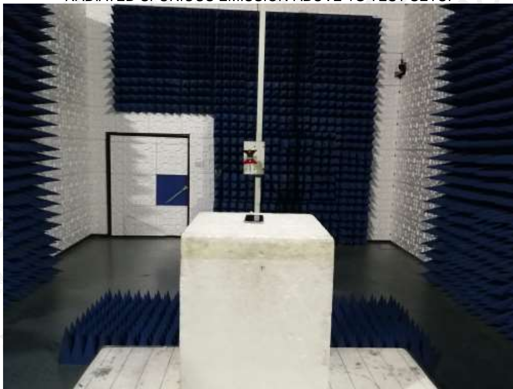
RADIATED SPURIOUS EMISSION-ABOVE 1G TEST SETUP
