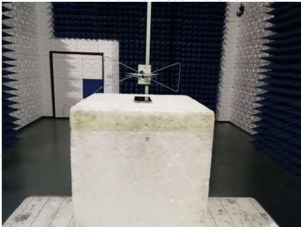
RADIATED SPURIOUS EMISSION-ABOVE 1G TEST SETUP
