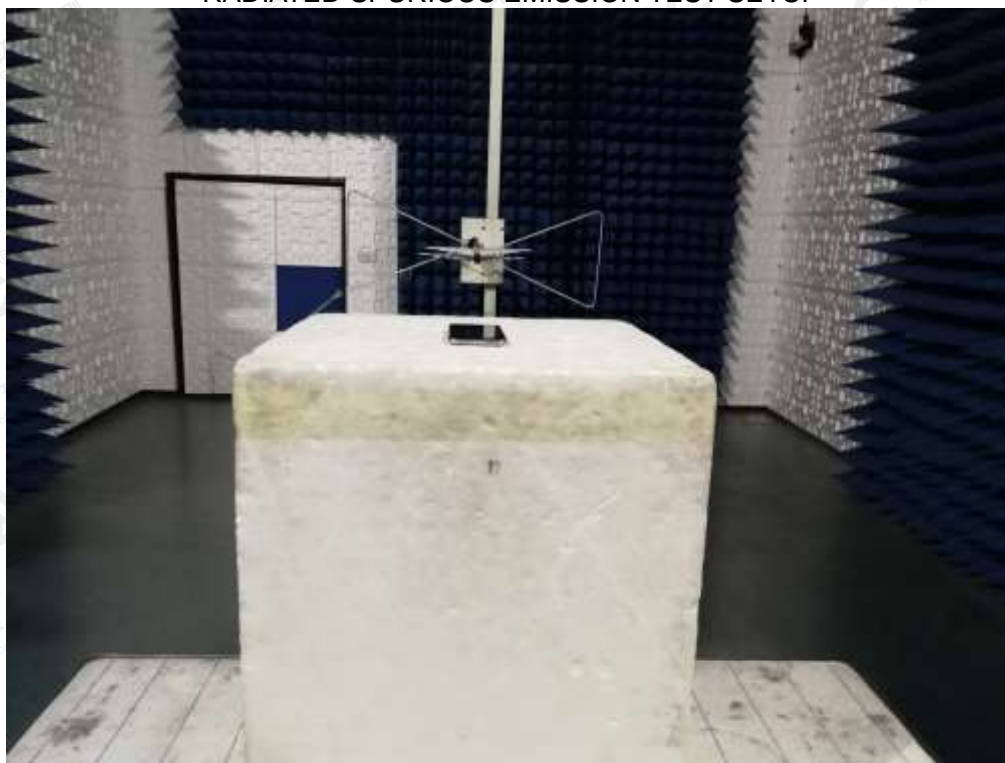
RADIATED SPURIOUS EMISSION-ABOVE 1G TEST SETUP
