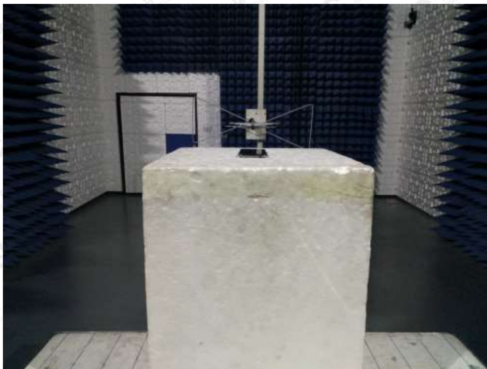
RADIATED SPURIOUS EMISSION-ABOVE 1G TEST SETUP
