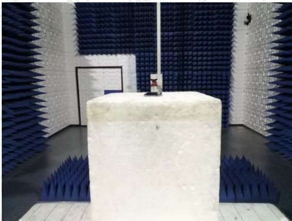
RADIATED SPURIOUS EMISSION-ABOVE 1G TEST SETUP
