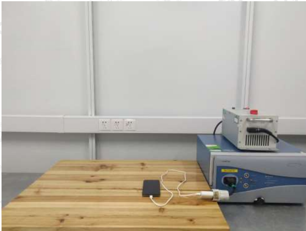
EFT SURGE and DIPS IMMUNITY TEST SETUP
