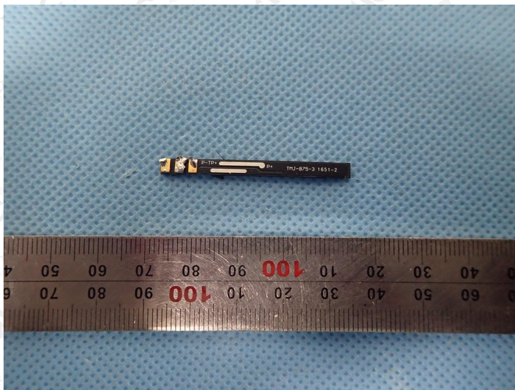
Fig.13 – bottom circuit of battery
