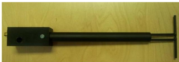
Figure 1 – MVG COMOSAR Validation Dipole
