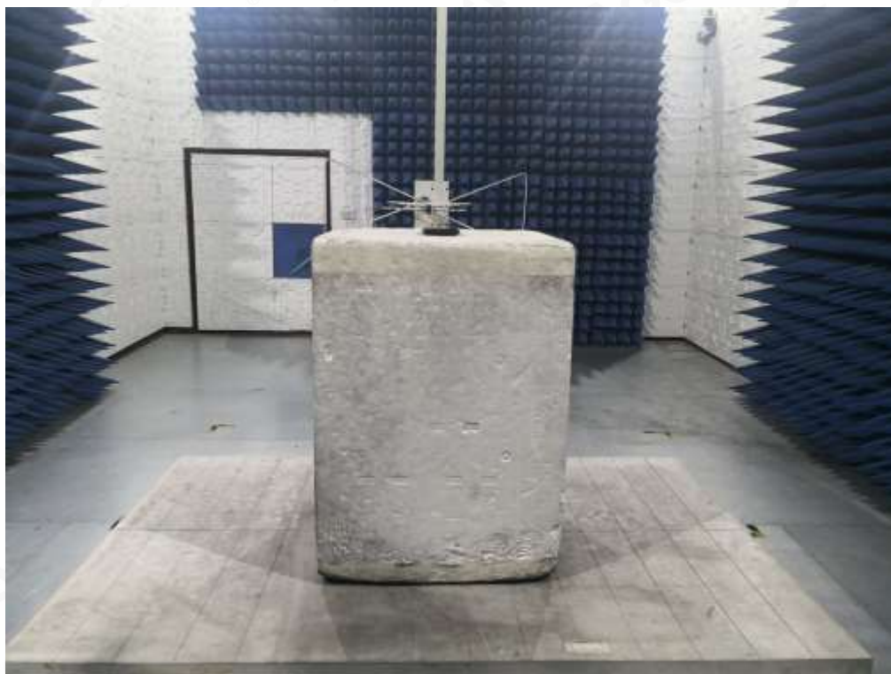
RADIATED SPURIOUS EMISSION ABOVE 1G TEST SETUP
