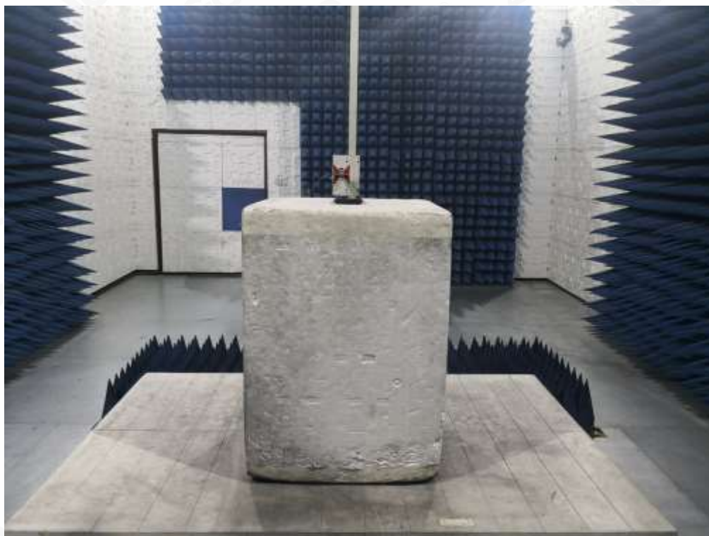
RADIATED SPURIOUS EMISSION ABOVE 1G TEST SETUP
