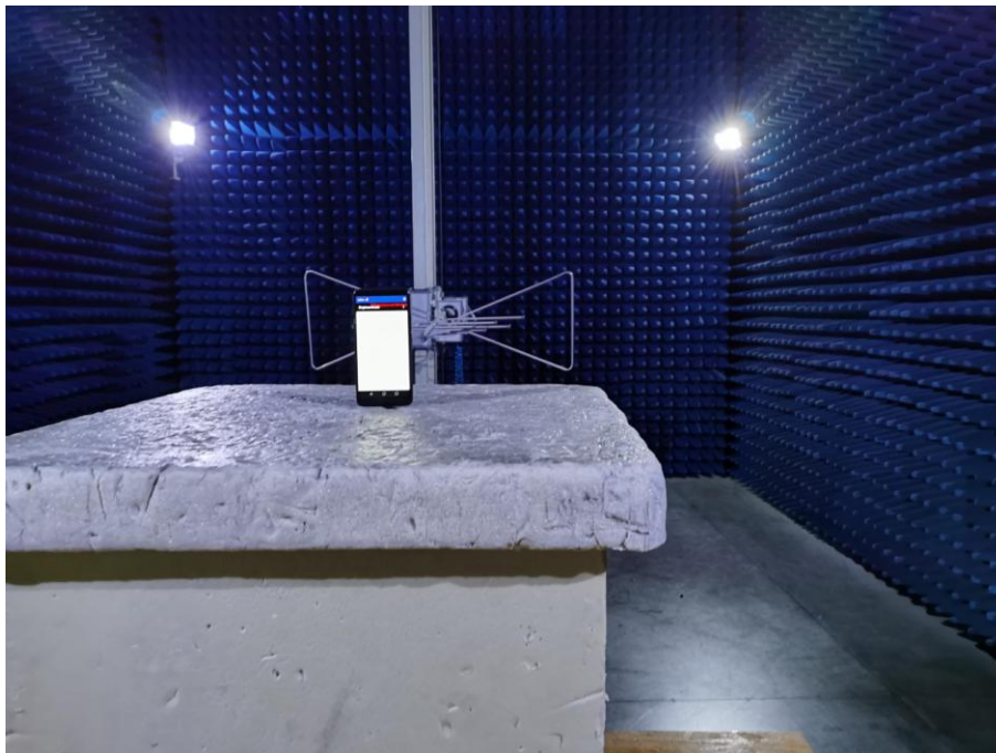
Radiated Spurious Emissions Test View (Below 1GHz)
