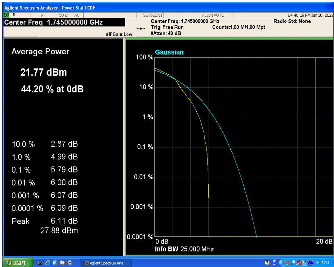
Band66 16QAM BW=10MHz Channel=132322 RB Size=1 Position=#0
