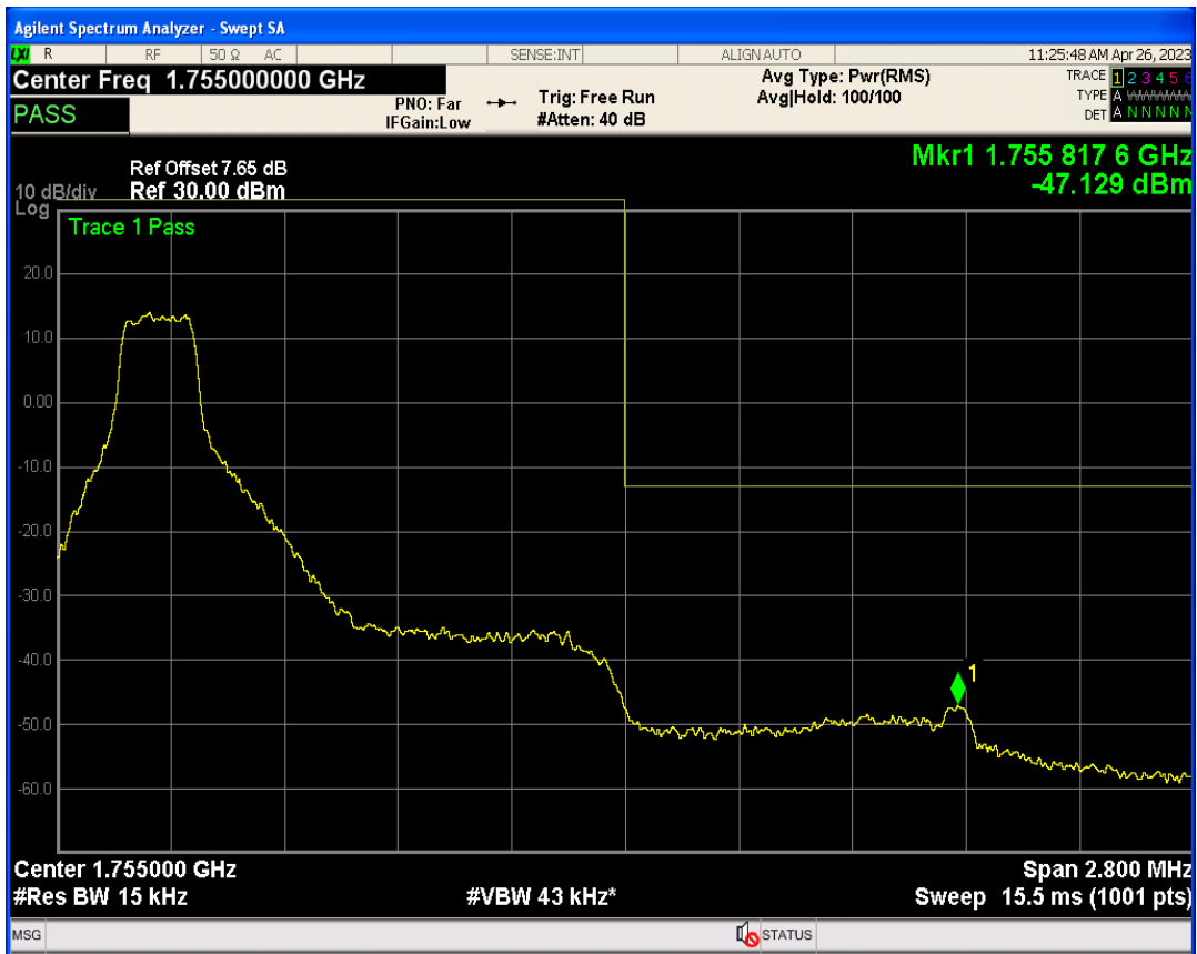
Band4 QPSK BW=1.4MHz Channel=20393 RB Size=1 Position=#Max
