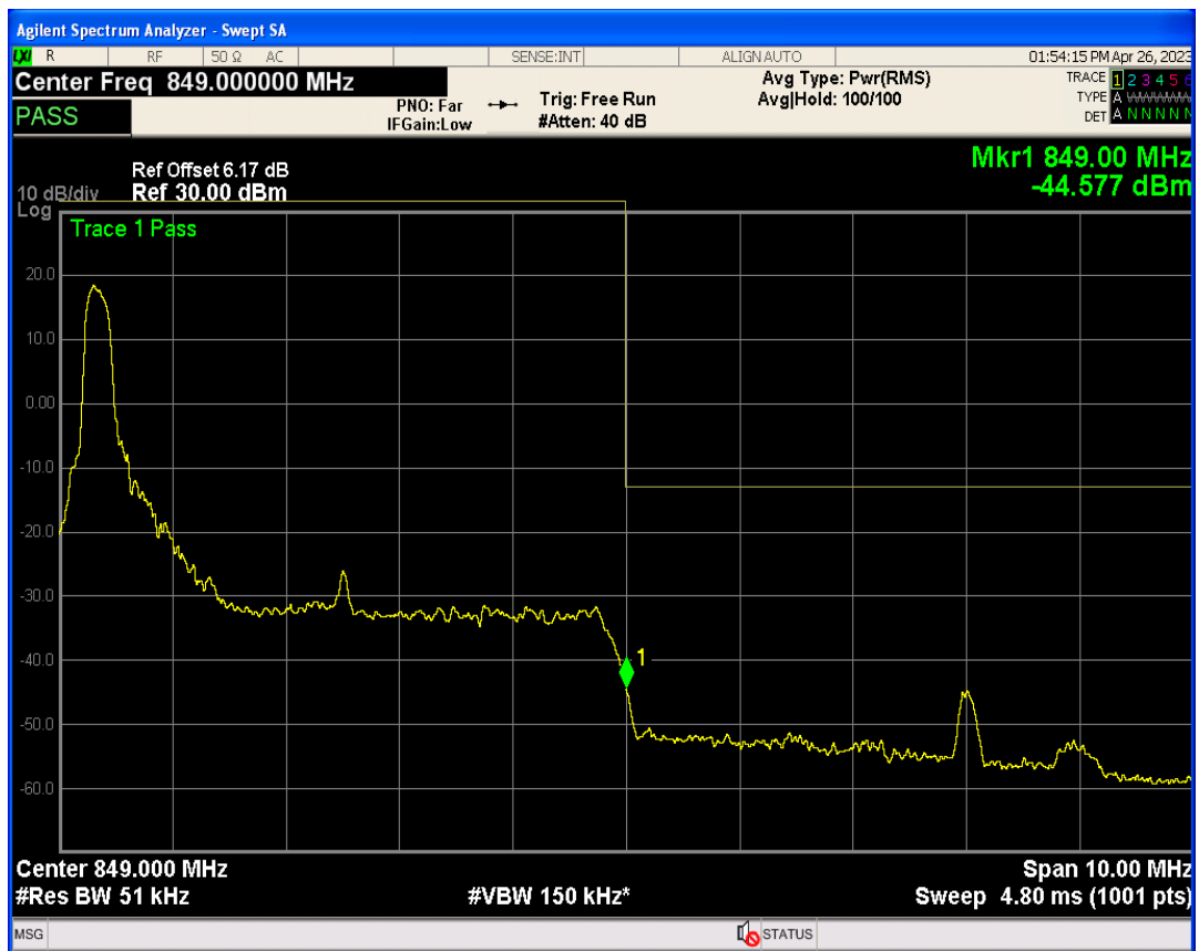
Band5 16QAM BW=5MHz Channel=20625 RB Size=25 Position=#0
