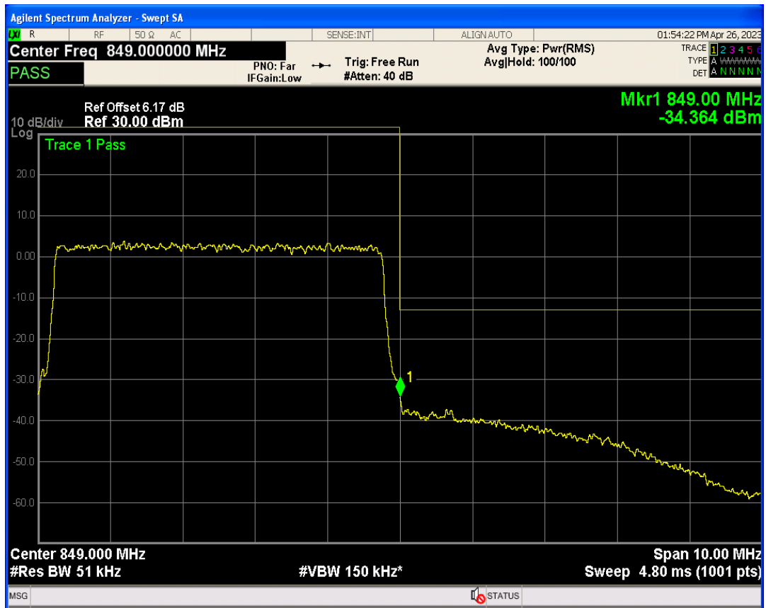
Band5 16QAM BW=5MHz Channel=20625 RB Size=1 Position=#Max
