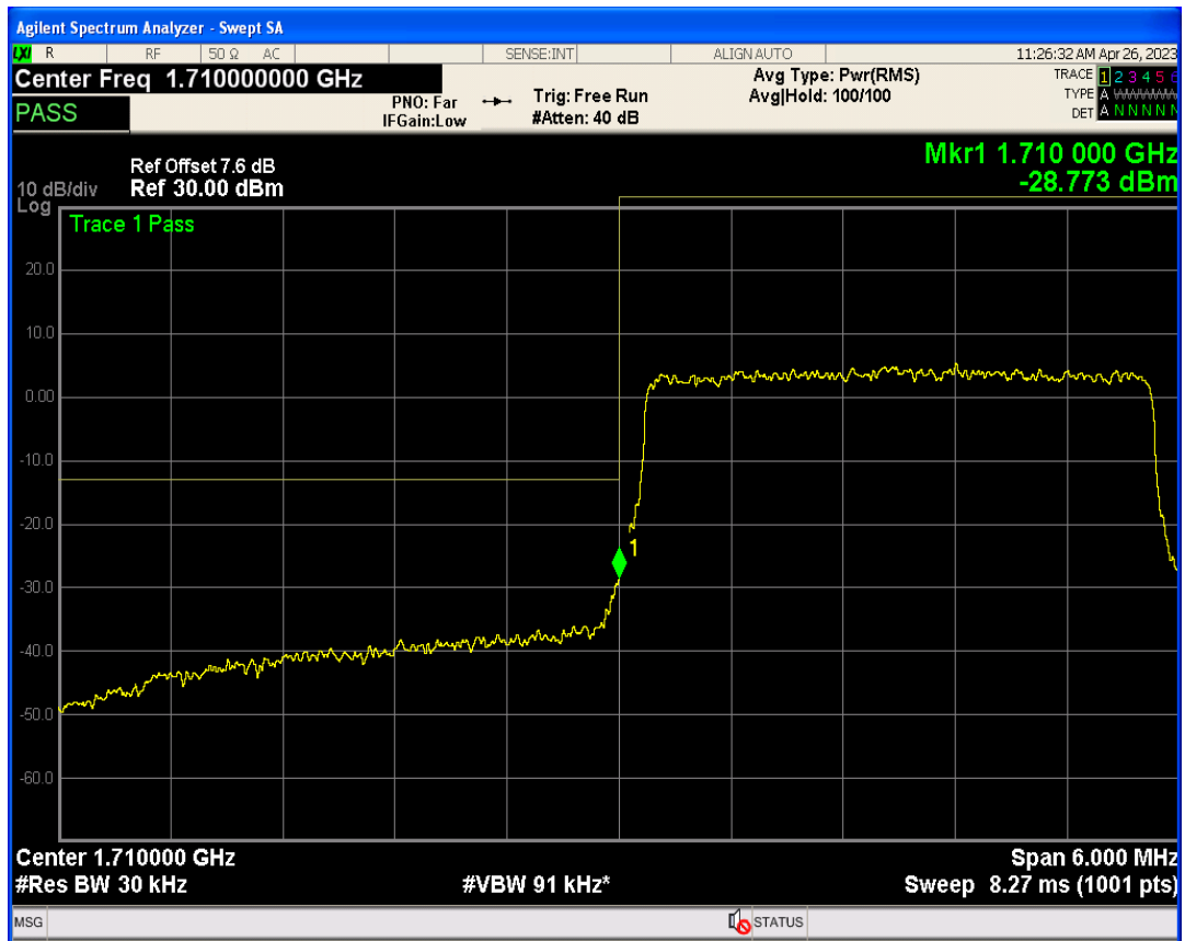
Band4 16QAM BW=3MHz Channel=19965 RB Size=1 Position=#0
