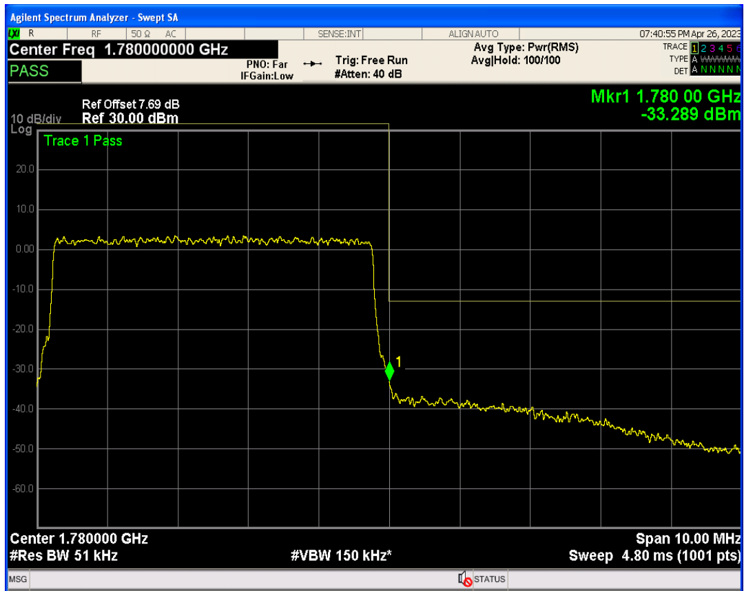
Band66 QPSK BW=10MHz Channel=132022 RB Size=50 Position=#0
