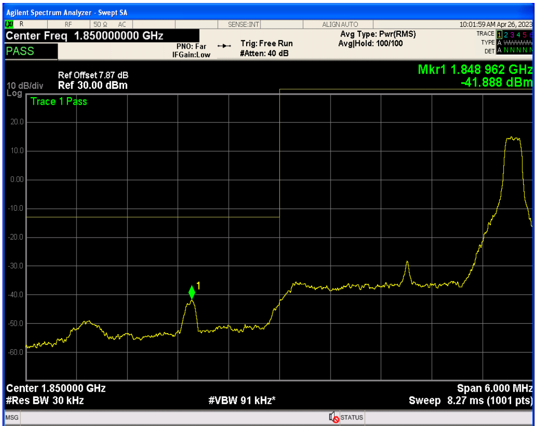
Band2 16QAM BW=3MHz Channel=18615 RB Size=15 Position=#0
