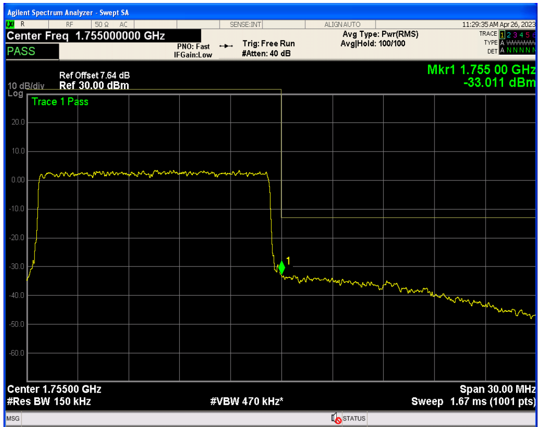
Band4 QPSK BW=20MHz Channel=20050 RB Size=1 Position=#Max
