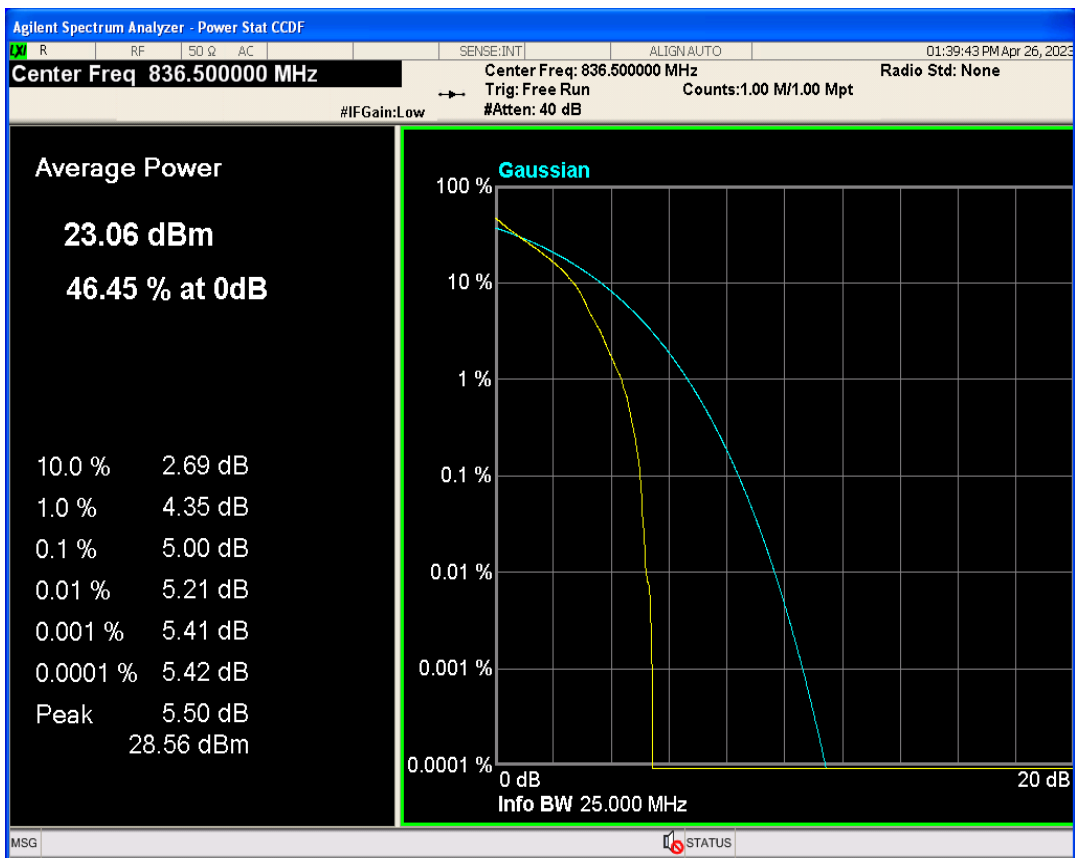
Band5 QPSK BW=5MHz Channel=20525 RB Size=1 Position=#0
