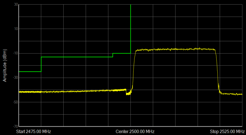
Band7 16QAM BW=20MHz Channel=20850 RB Size=100 Position=#0
