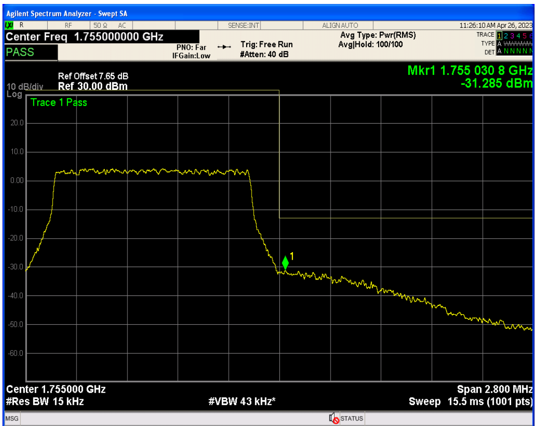
Band4 QPSK BW=3MHz Channel=19965 RB Size=1 Position=#Max
