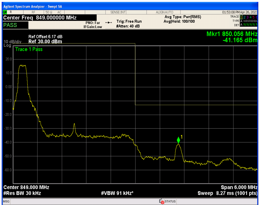
Band5 16QAM BW=3MHz Channel=20415 RB Size=15 Position=#0
