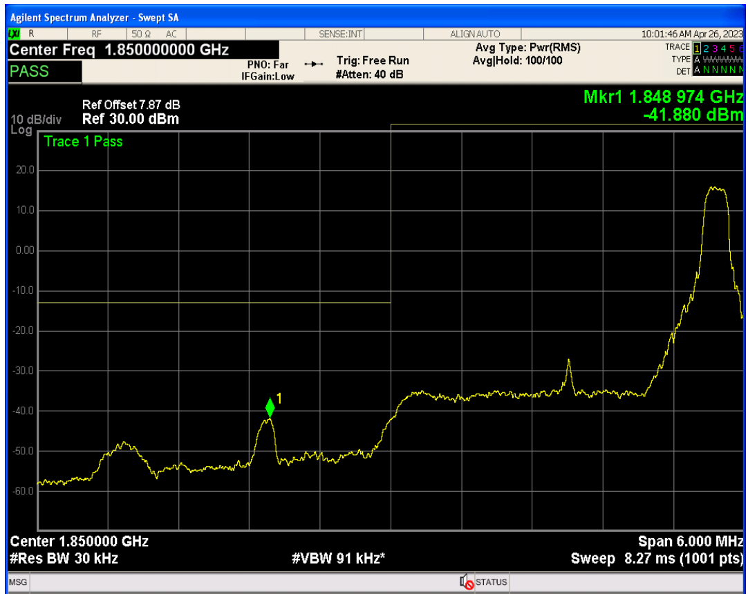
Band2 QPSK BW=3MHz Channel=18615 RB Size=1 Position=#0
