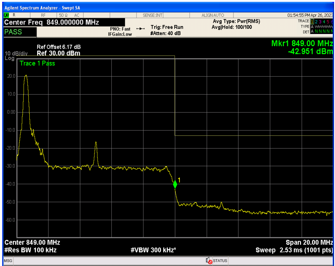
Band5 QPSK BW=10MHz Channel=20600 RB Size=1 Position=#Max
