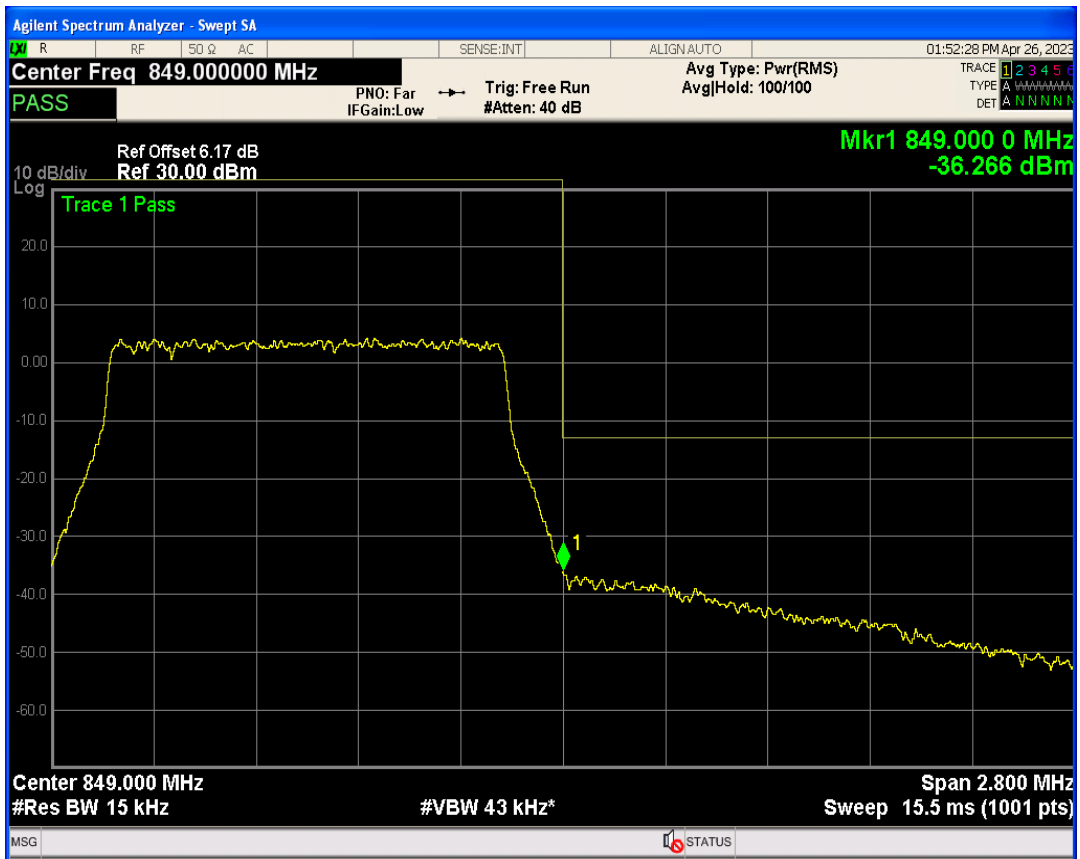
Band5 16QAM BW=1.4MHz Channel=20643 RB Size=1 Position=#Max
