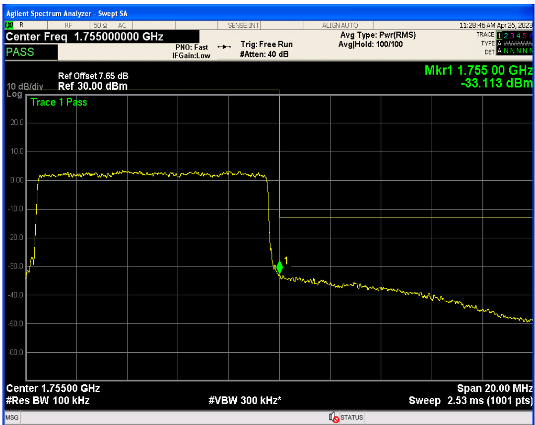
Band4 QPSK BW=15MHz Channel=20025 RB Size=1 Position=#Max
