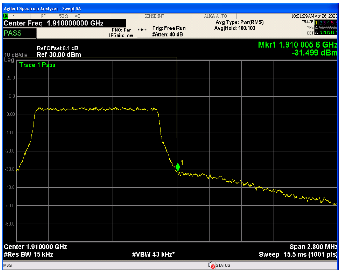
Band2 QPSK BW=3MHz Channel=18615 RB Size=1 Position=#Max
