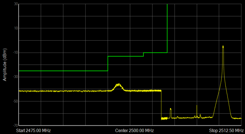
Band7 16QAM BW=10MHz Channel=20800 RB Size=1 Position=#Max
