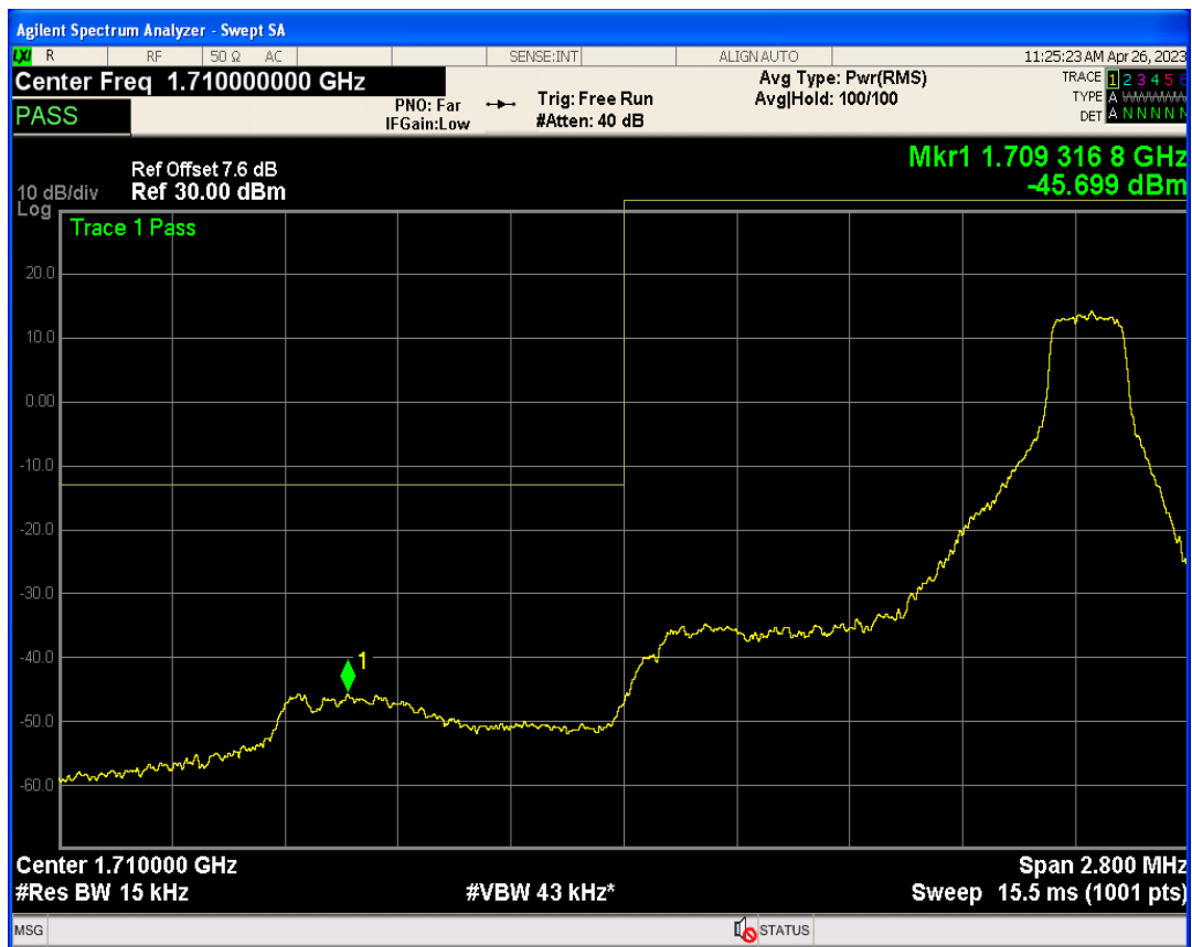
Band4 QPSK BW=1.4MHz Channel=19957 RB Size=6 Position=#0
