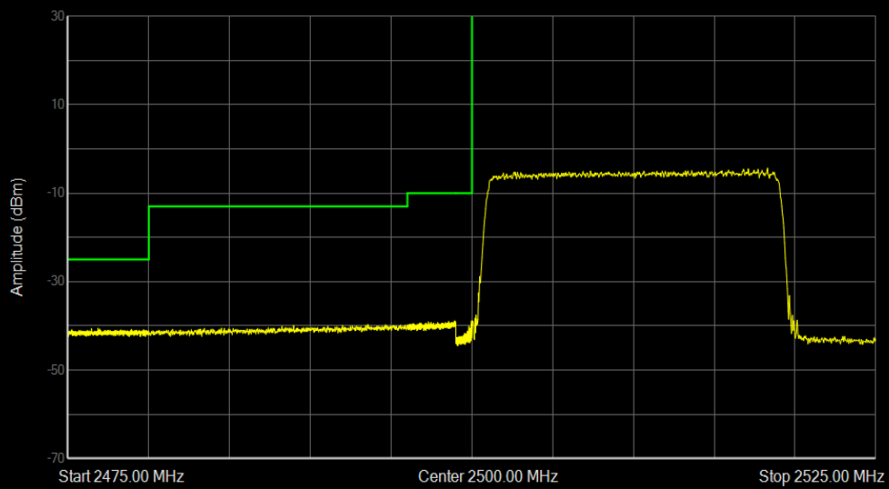
Band7 QPSK BW=20MHz Channel=20850 RB Size=100 Position=#0
