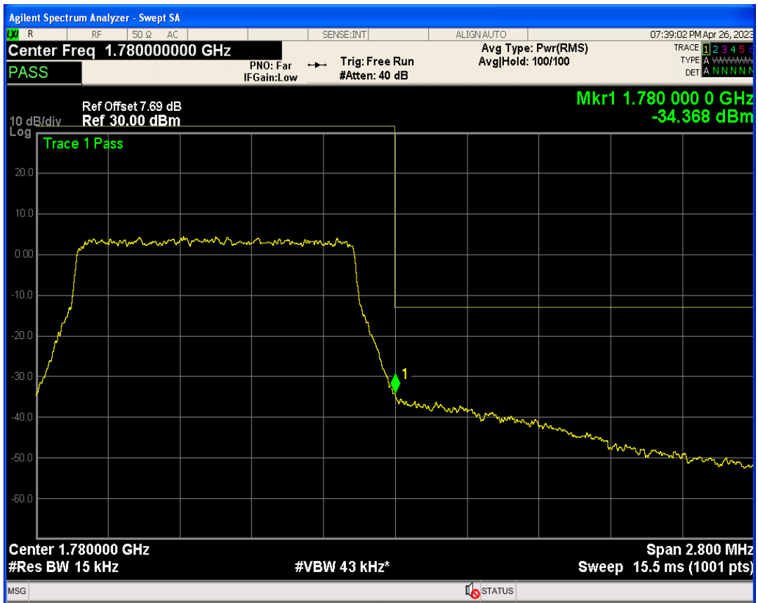
Band66 16QAM BW=1.4MHz Channel=132665 RB Size=1 Position=#Max
