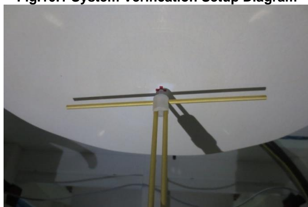
Fig.10.2 Photo of Dipole setup
