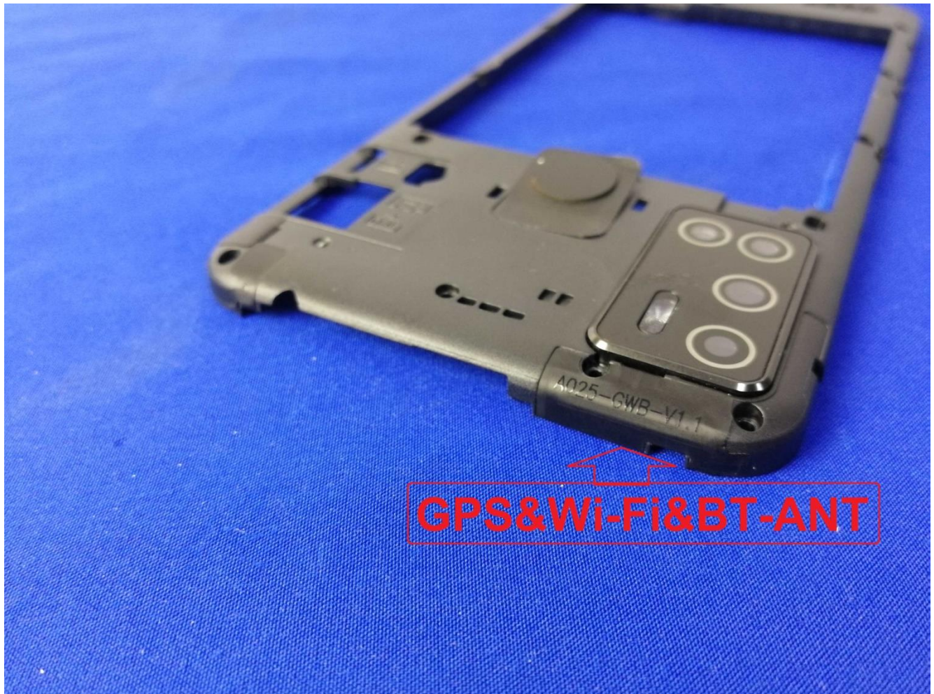
Fig.14.1 EUT Antenna Locations
