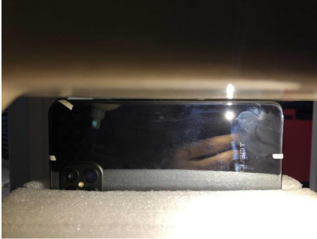
Extremity – Left (Test distance: 5mm, Thickness of DUT: 9mm)
