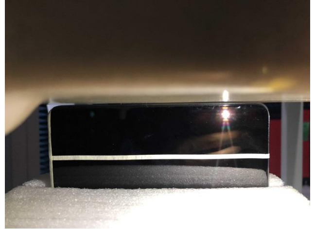
Extremity – Right (Test distance: 5mm, Thickness of DUT: 9mm)
