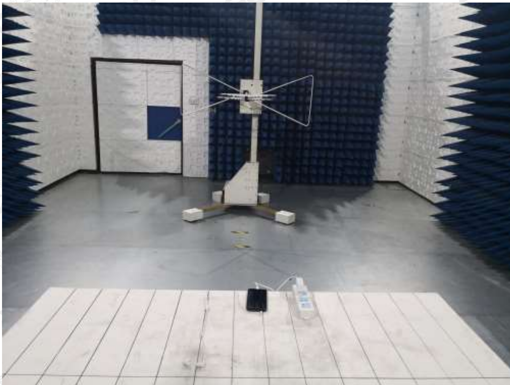
EN 55032 RADIATED EMISSION TEST SETUP
