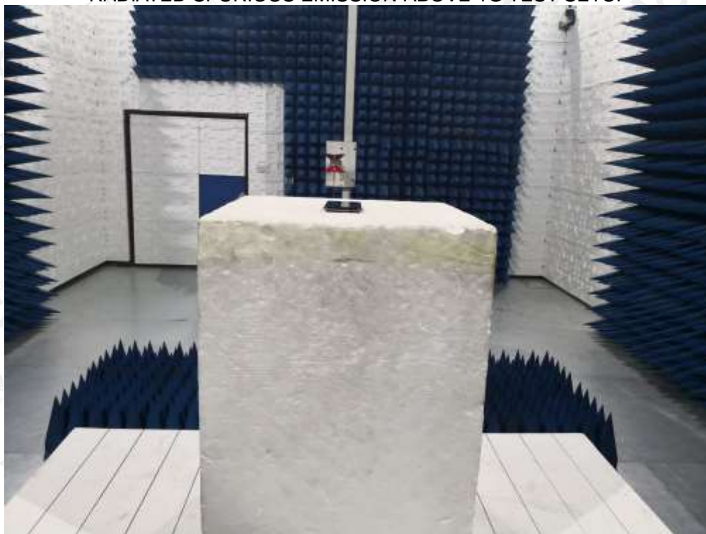
RADIATED SPURIOUS EMISSION-ABOVE 1G TEST SETUP
