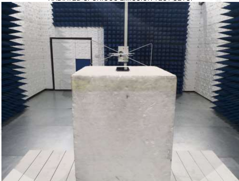
RADIATED SPURIOUS EMISSION-ABOVE 1G TEST SETUP
