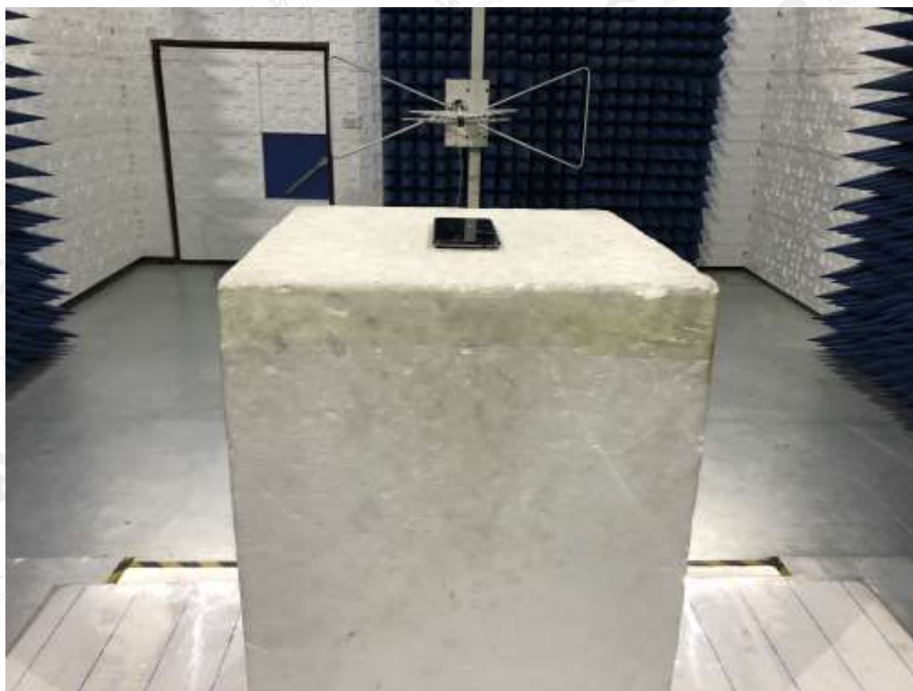
RADIATED SPURIOUS EMISSION-ABOVE 1G TEST SETUP
