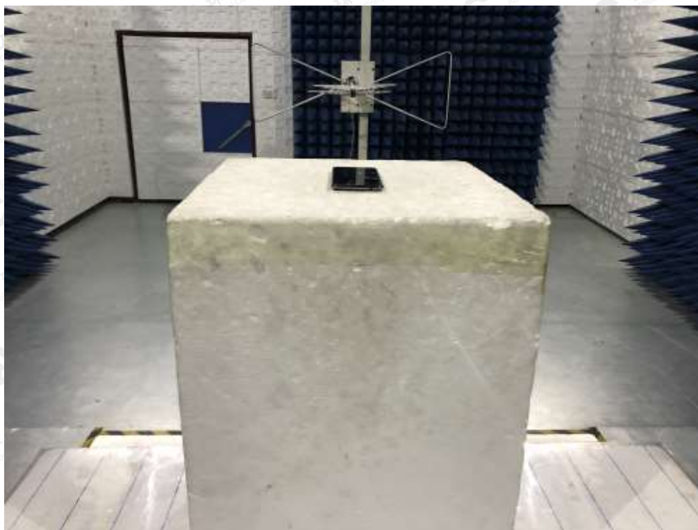
RADIATED SPURIOUS EMISSION-ABOVE 1G TEST SETUP
