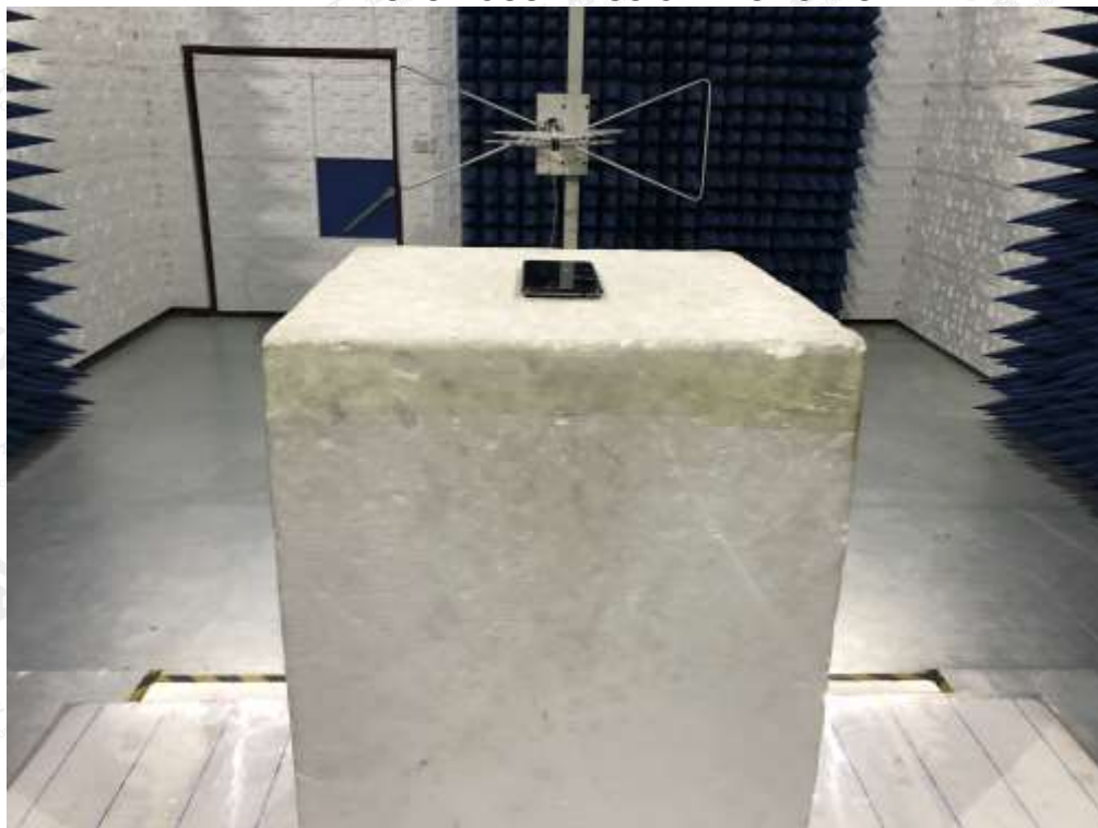
RADIATED SPURIOUS EMISSION-ABOVE 1G TEST SETUP
