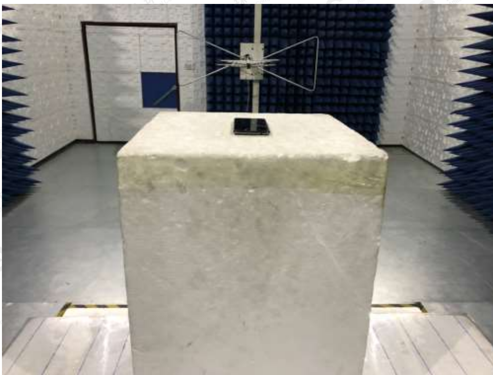
RADIATED SPURIOUS EMISSION-ABOVE 1G TEST SETUP
