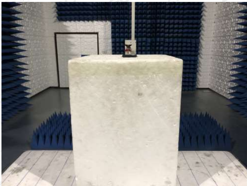
RADIATED SPURIOUS EMISSION-ABOVE 1G TEST SETUP
