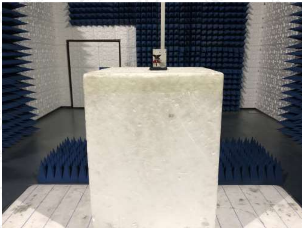
RADIATED SPURIOUS EMISSION-ABOVE 1G TEST SETUP
