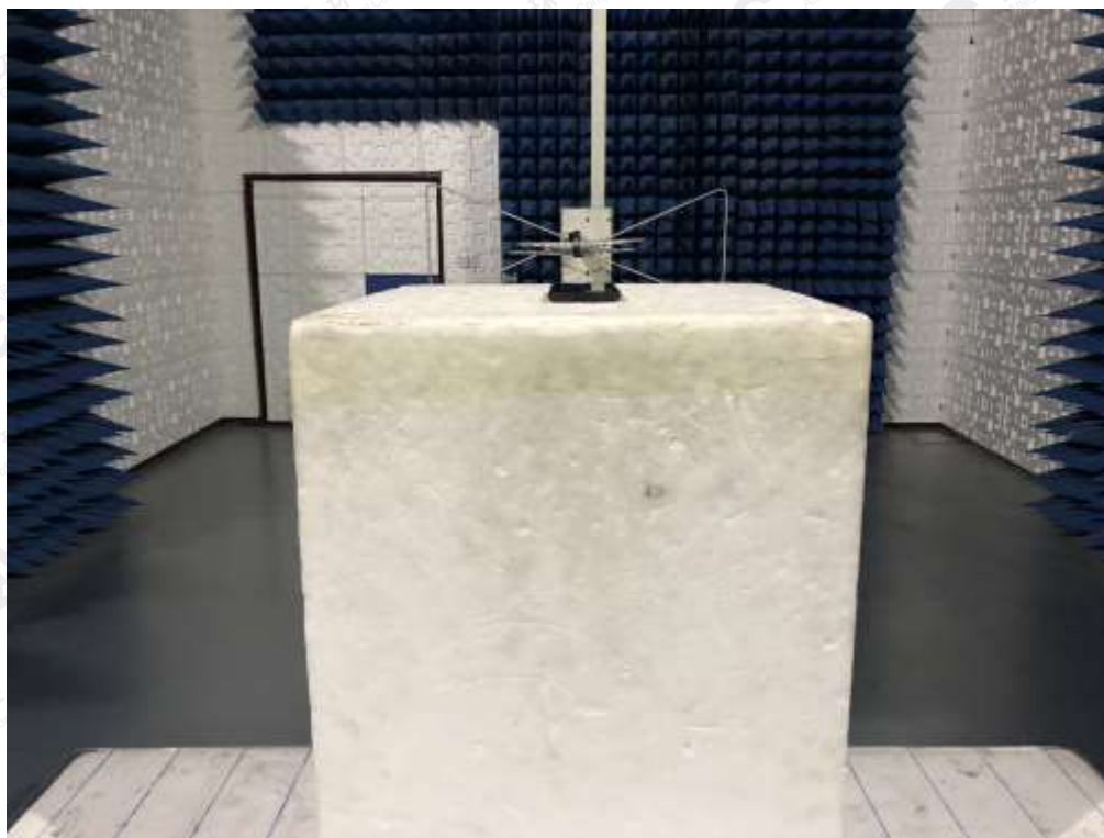
RADIATED SPURIOUS EMISSION-ABOVE 1G TEST SETUP
