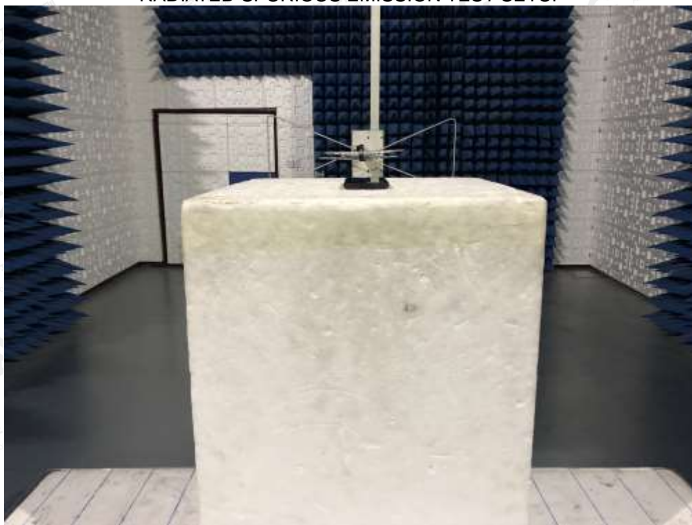
RADIATED SPURIOUS EMISSION-ABOVE 1G TEST SETUP
