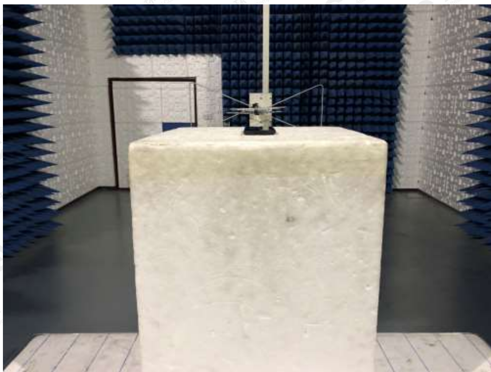
RADIATED SPURIOUS EMISSION-ABOVE 1G TEST SETUP
