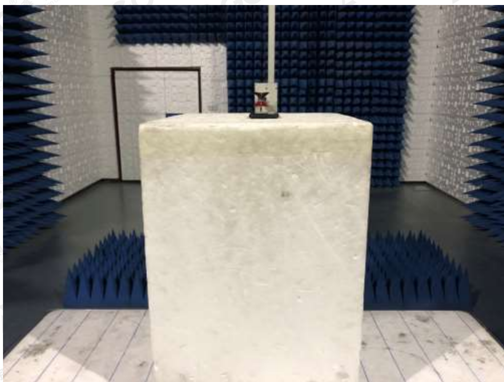
RADIATED SPURIOUS EMISSION-ABOVE 1G TEST SETUP
