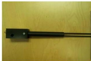
Figure 1 – MVG COMOSAR Validation Dipole
