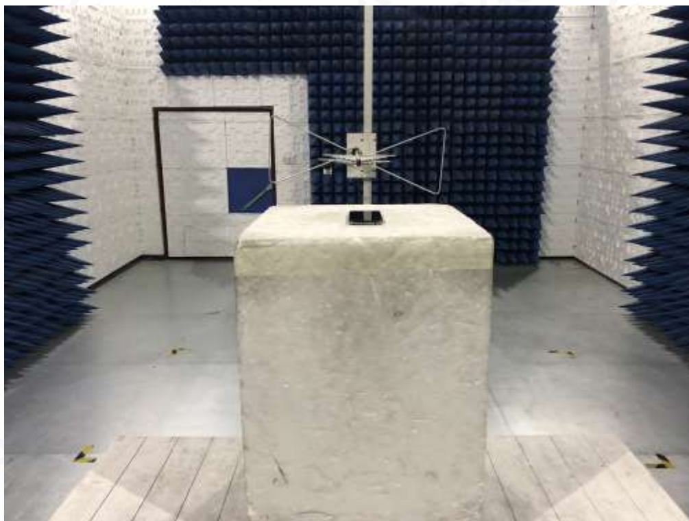
RADIATED SPURIOUS EMISSION ABOVE 1G TEST SETUP
