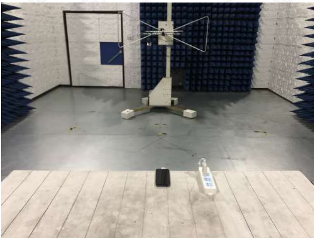
RADIATED EMISSION TEST SETUP
