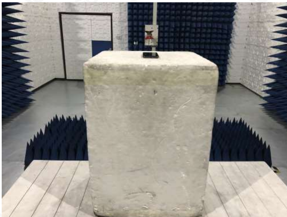
RADIATED SPURIOUS EMISSION-ABOVE 1G TEST SETUP
