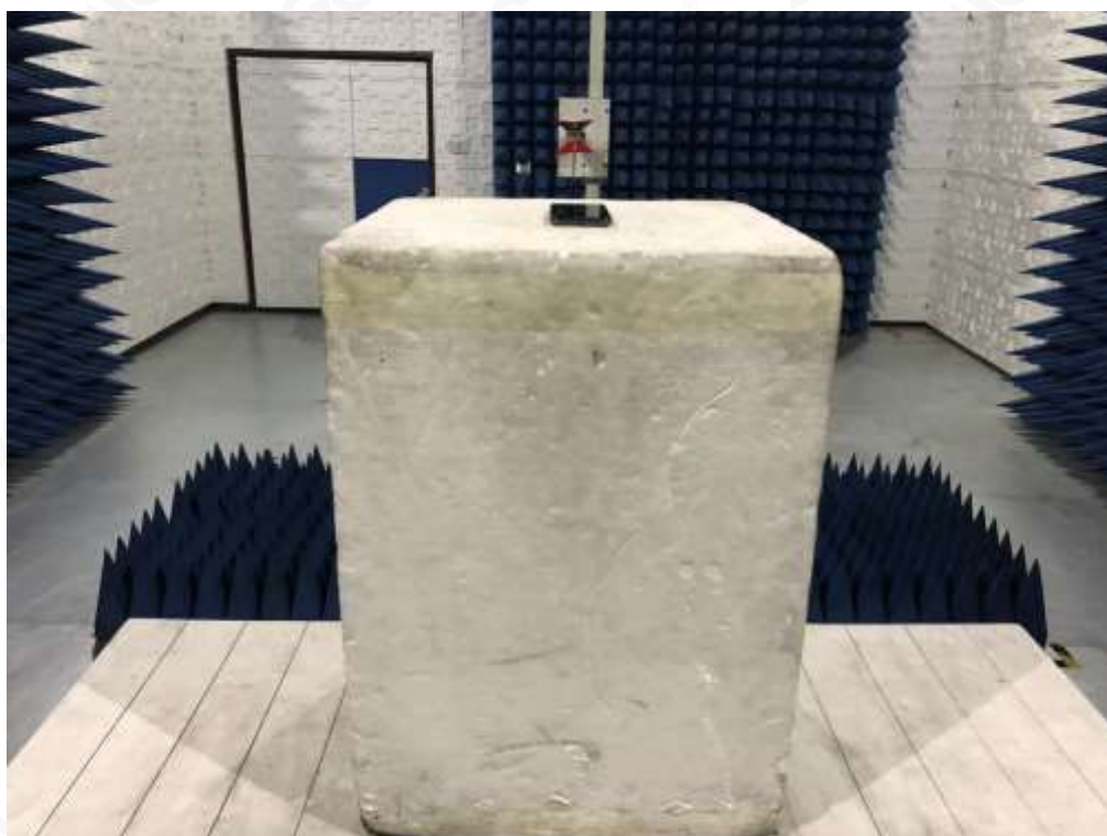
RADIATED SPURIOUS EMISSION-ABOVE 1G TEST SETUP
