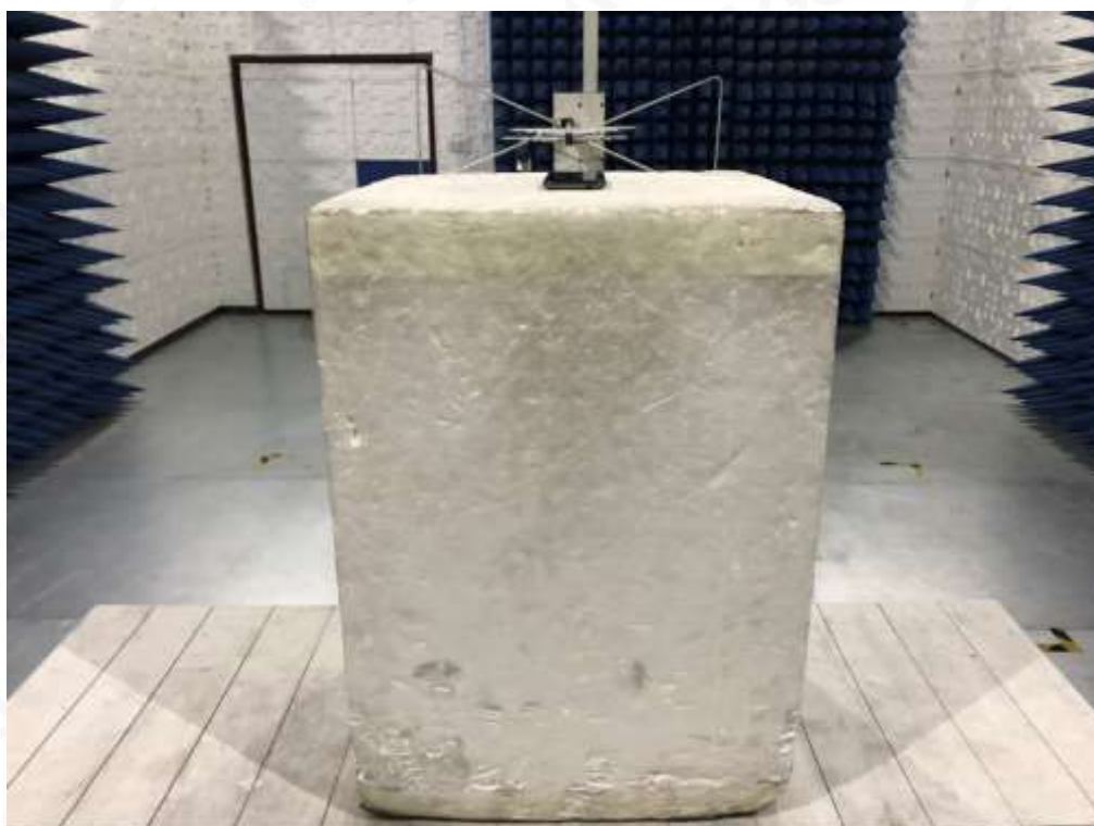
RADIATED SPURIOUS EMISSION-ABOVE 1G TEST SETUP
