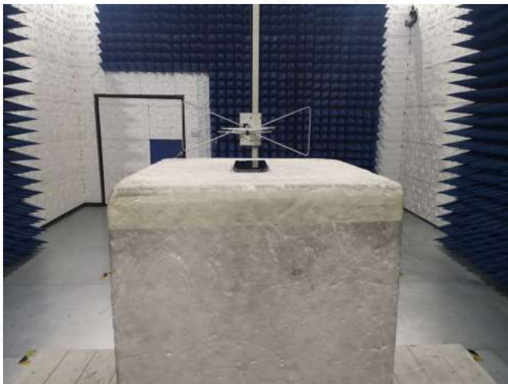
RADIATED SPURIOUS EMISSION-ABOVE 1G TEST SETUP
