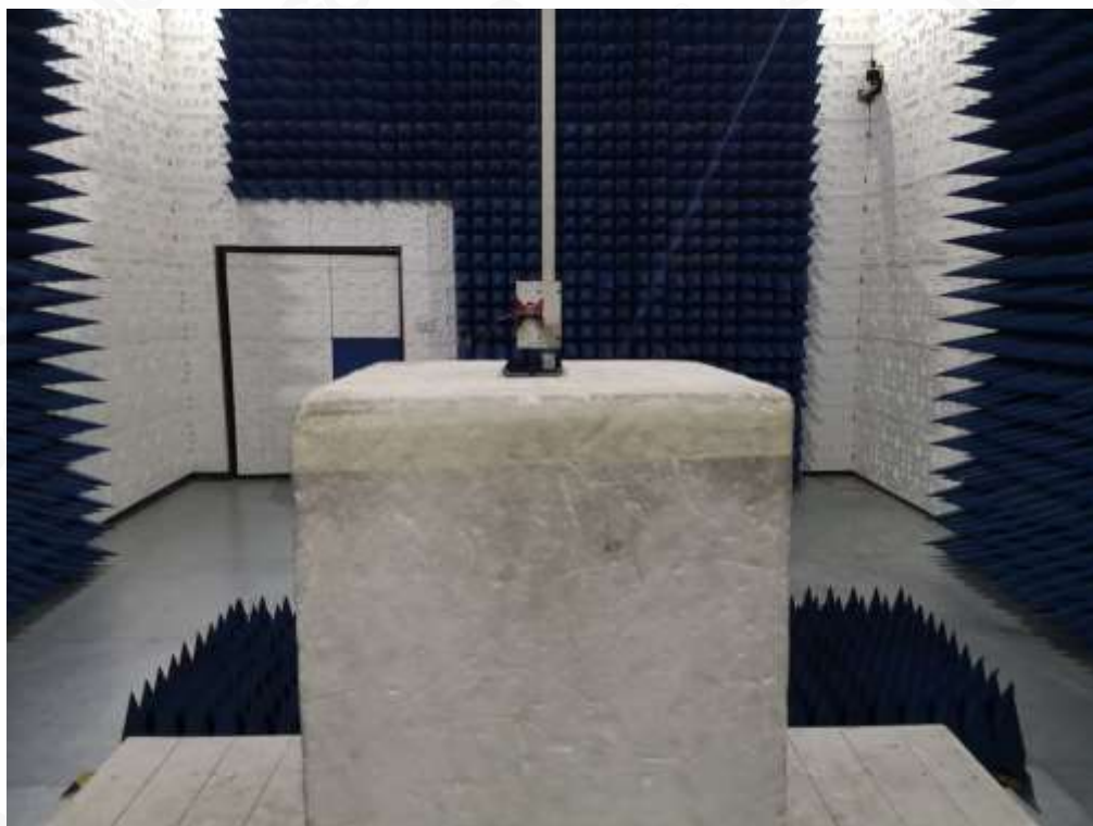
RADIATED SPURIOUS EMISSION-ABOVE 1G TEST SETUP
