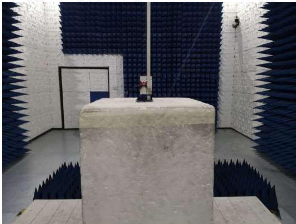
RADIATED SPURIOUS EMISSION-ABOVE 1G TEST SETUP
