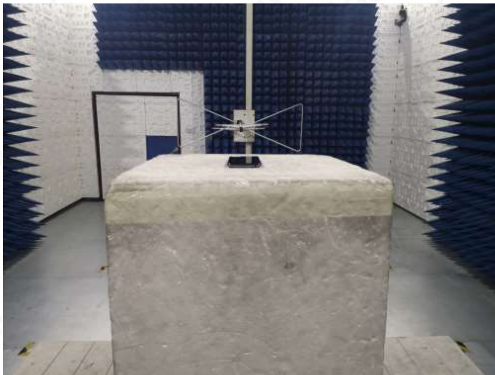
RADIATED SPURIOUS EMISSION-ABOVE 1G TEST SETUP
