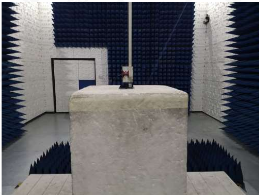
RADIATED SPURIOUS EMISSION-ABOVE 1G TEST SETUP
