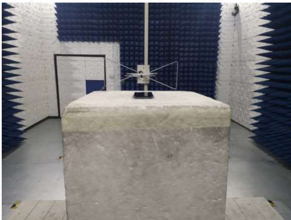
RADIATED SPURIOUS EMISSION-ABOVE 1G TEST SETUP
