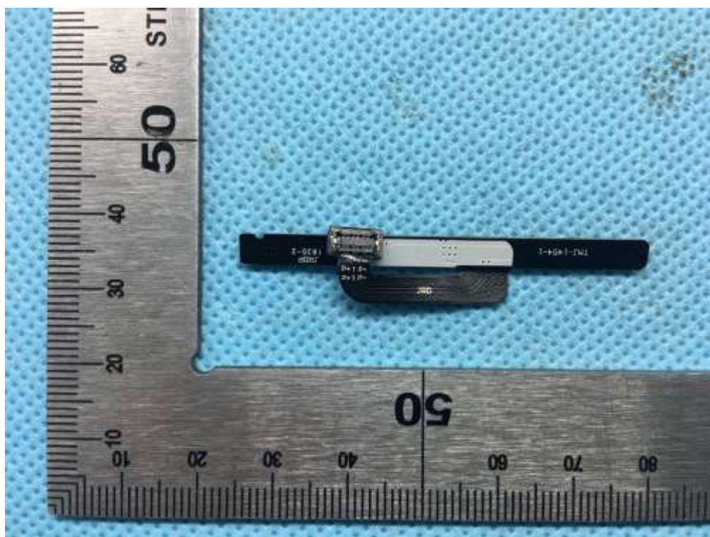
Fig.13 – bottom circuit of battery
