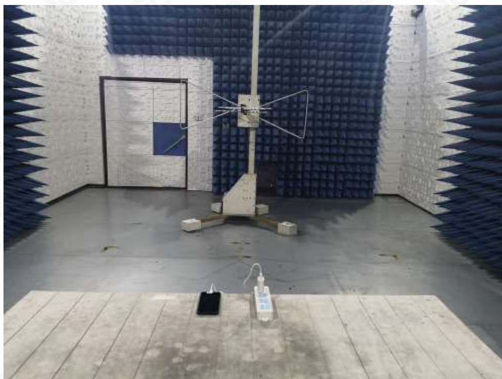
RADIATED EMISSION TEST SETUP
