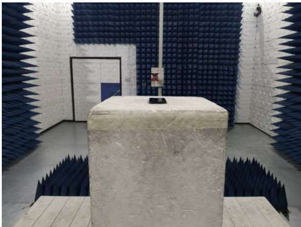
RADIATED SPURIOUS EMISSION-ABOVE 1G TEST SETUP
