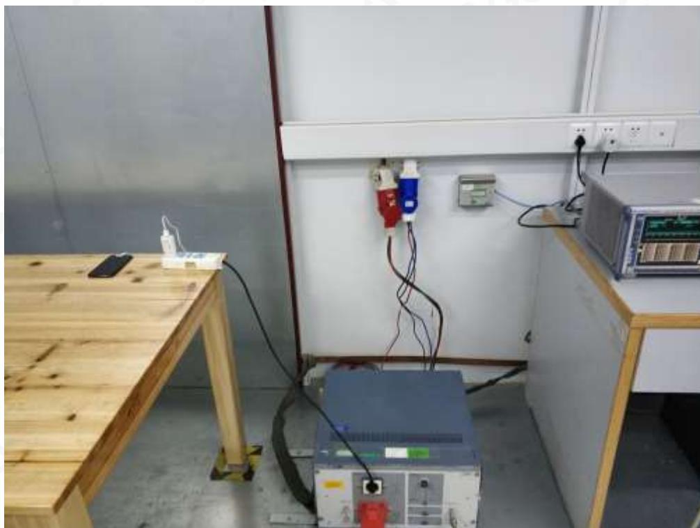
RADIATED EMISSION TEST SETUP
