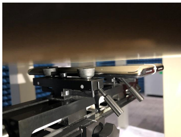
Body worn – Back (Test distance: 5mm, Thickness of DUT: 9mm)
