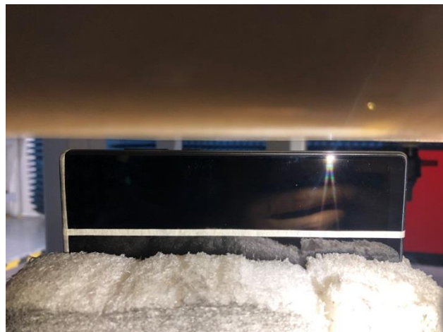
Body worn – Right (Test distance: 5mm, Thickness of DUT: 9mm)
