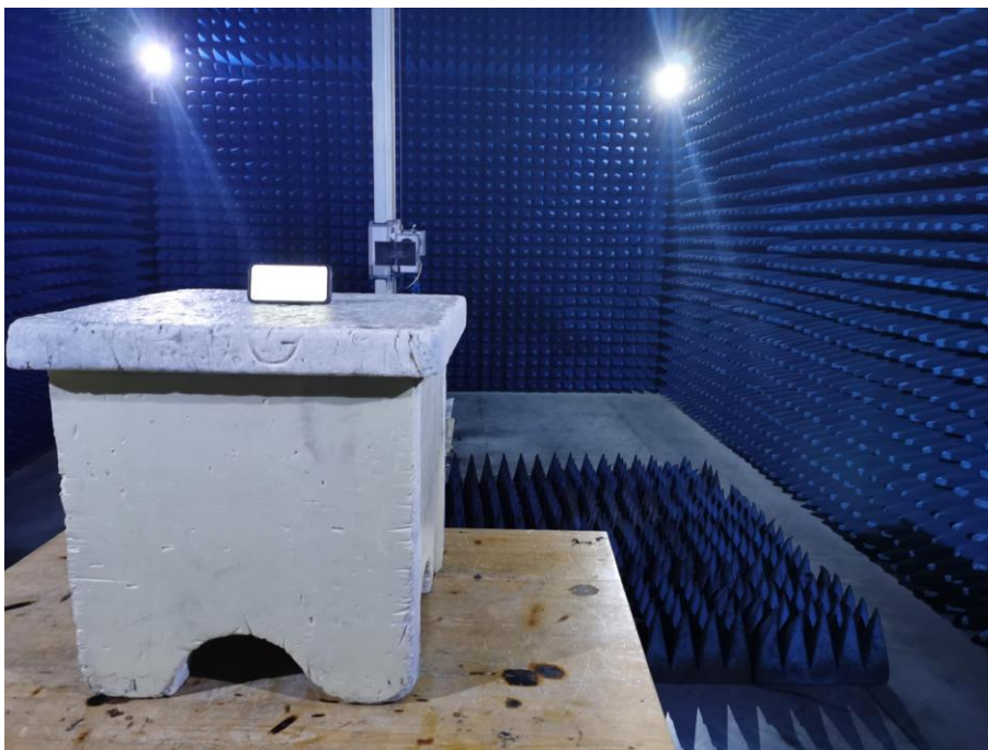
Radiated Spurious Emissions Test View (Above 1GHz)
