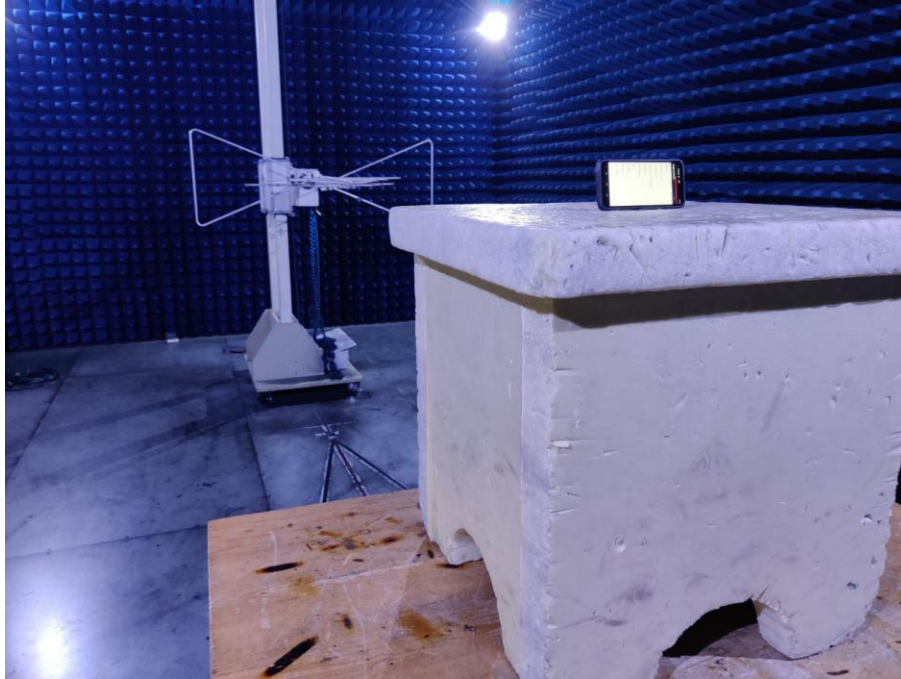
Radiated Spurious Emissions Test View (Below 1GHz)
