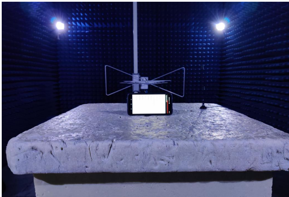
Radiated Spurious Emissions Test View (Above 1GHz)
