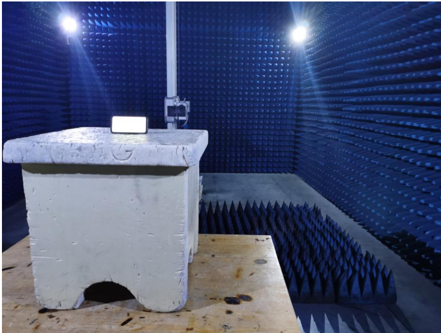
Radiated Spurious Emissions Test View (Above 1GHz)
