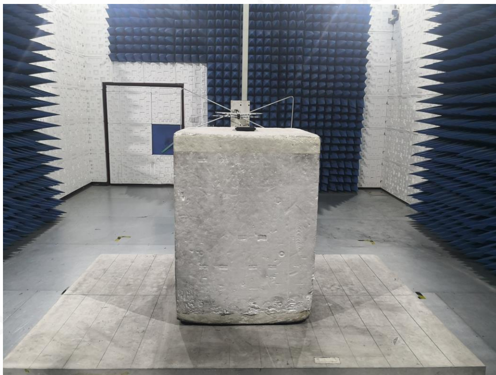
RADIATED SPURIOUS EMISSION ABOVE 1G TEST SETUP
