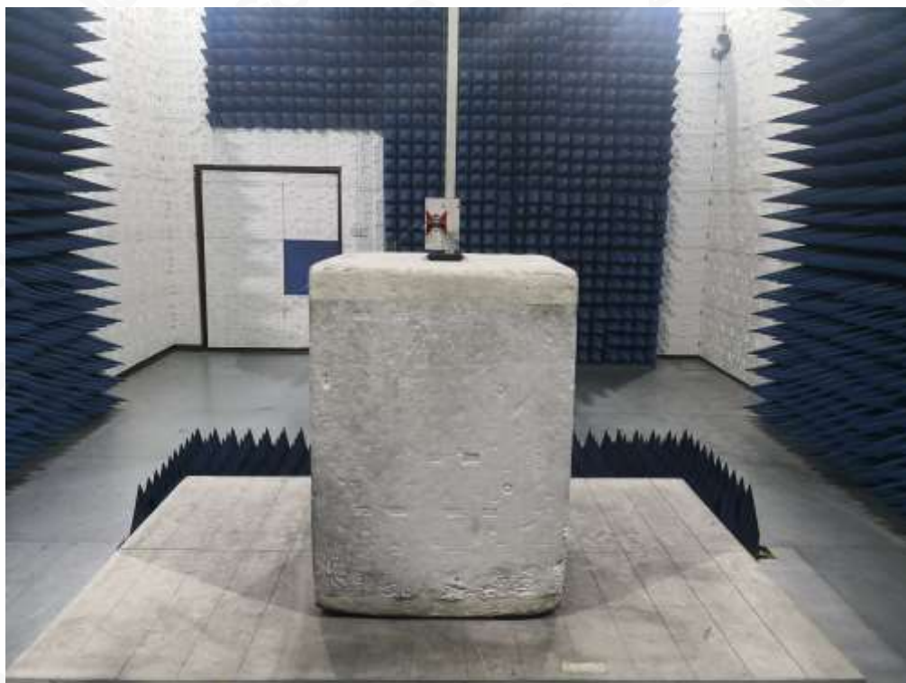
RADIATED SPURIOUS EMISSION ABOVE 1G TEST SETUP
