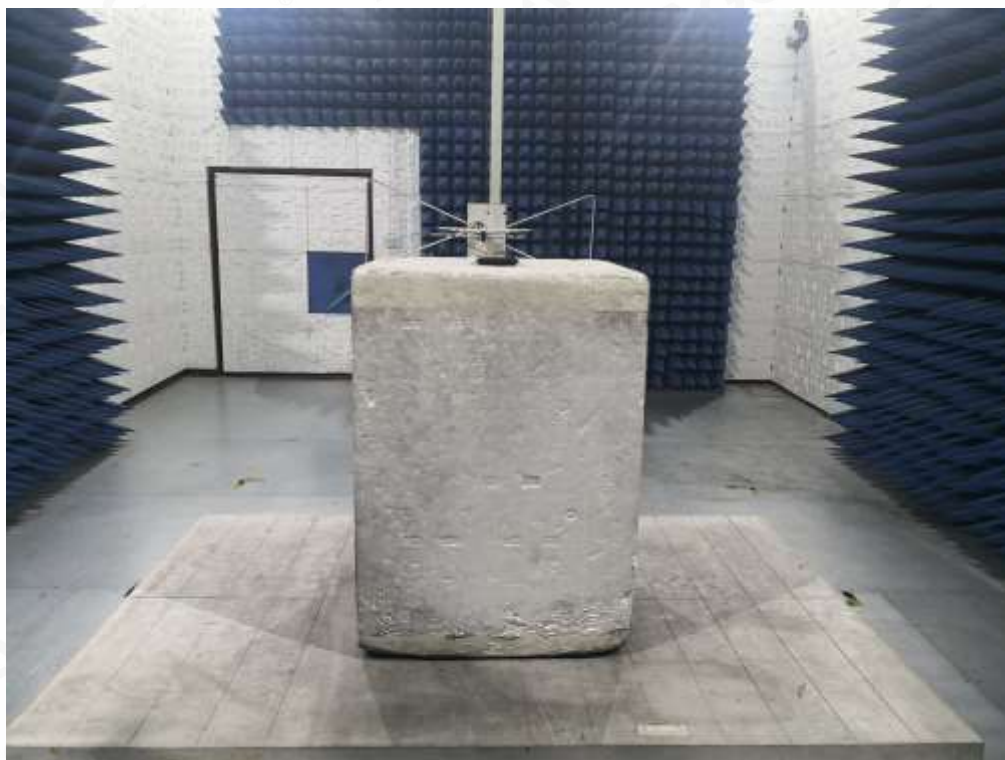
RADIATED SPURIOUS EMISSION ABOVE 1G TEST SETUP
