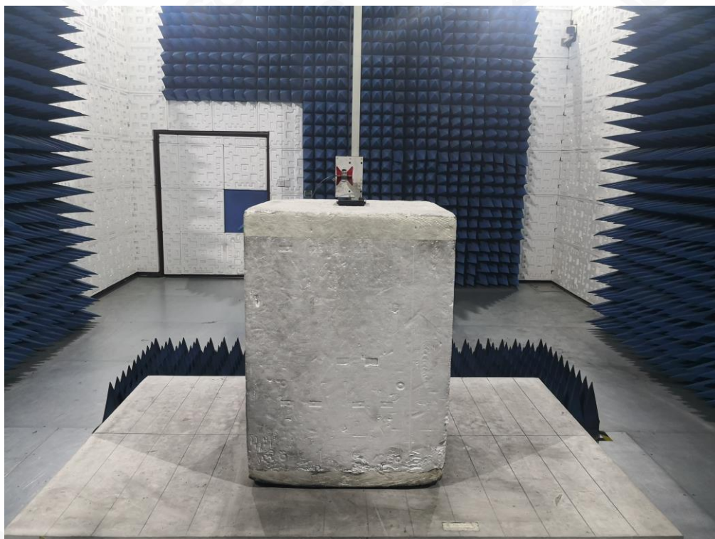
RADIATED SPURIOUS EMISSION ABOVE 1G TEST SETUP
