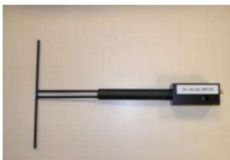
Figure 1 – Satimo COMOSAR Validation Dipole
