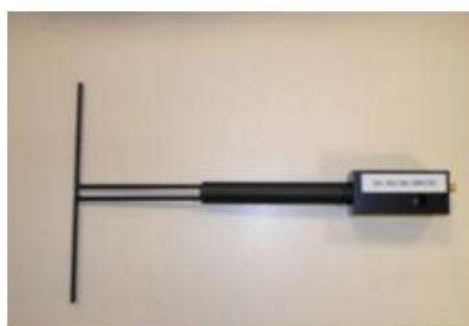
Figure 1 – Satimo COMOSAR Validation Dipole
