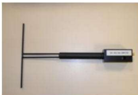
Figure 1 – Satimo COMOSAR Validation Dipole
