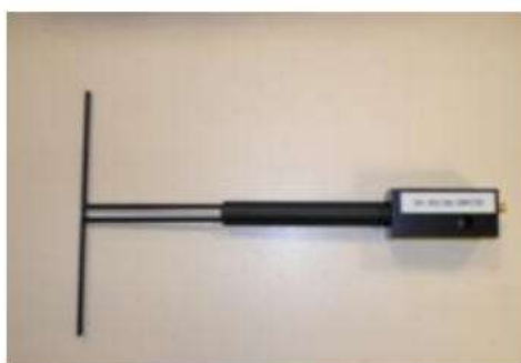
Figure 1 – Satimo COMOSAR Validation Dipole
