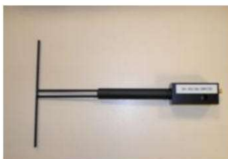
Figure 1 – Satimo COMOSAR Validation Dipole
