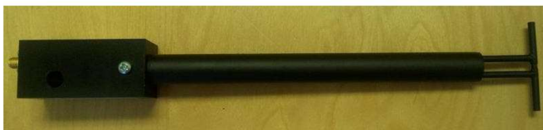
Figure 1 – MVG COMOSAR Validation Dipole
