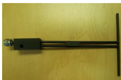
Figure 1 – MVG COMOSAR Validation Dipole
