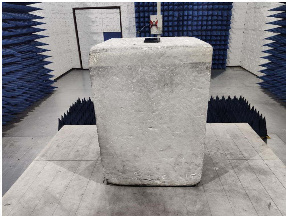
RADIATED SPURIOUS EMISSION ABOVE 1G TEST SETUP
