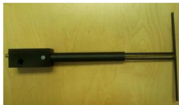
Figure 1 – MVG COMOSAR Validation Dipole
