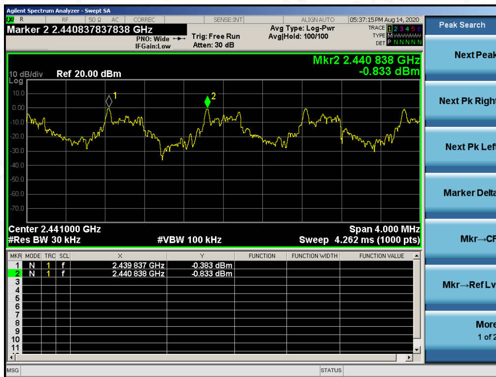
TEST PLOT FOR FREQUENCY SEPARATION
