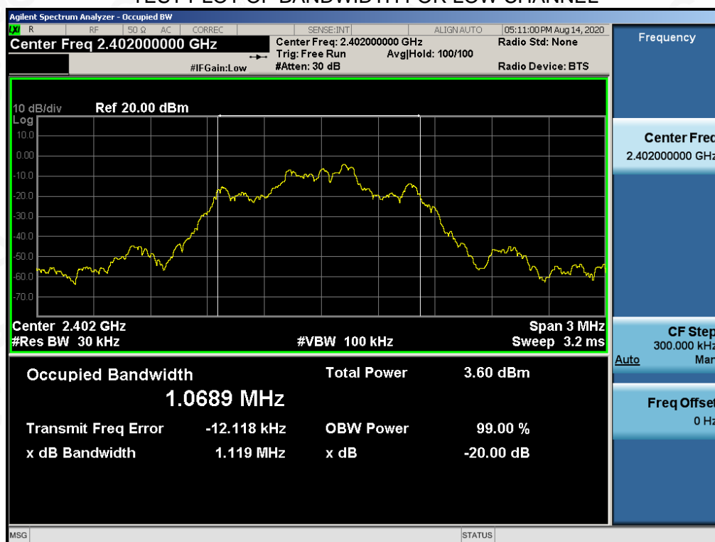
TEST PLOT OF BANDWIDTH FOR LOW CHANNEL
