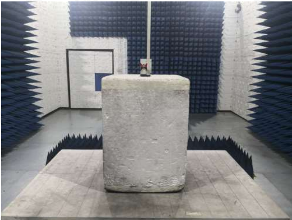
RADIATED SPURIOUS EMISSION ABOVE 1G TEST SETUP
