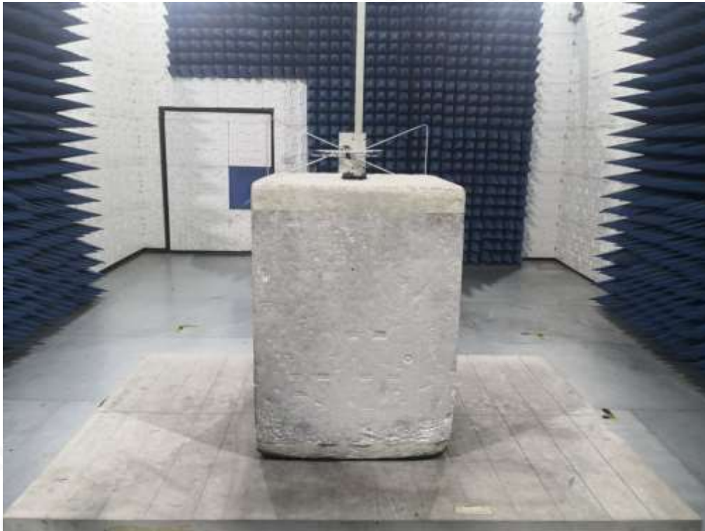
RADIATED SPURIOUS EMISSION ABOVE 1G TEST SETUP
