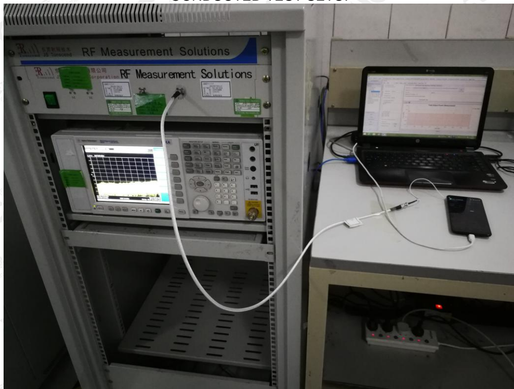
CONDUCTED TEST SETUP
