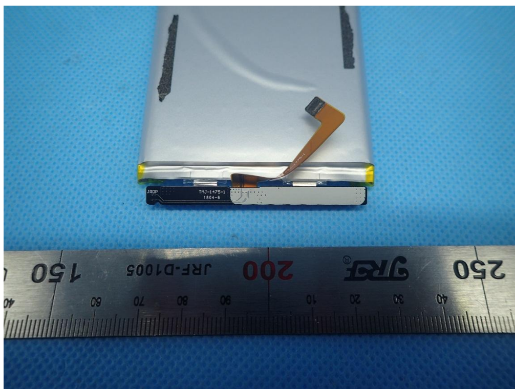
Fig.12 – bottom circuit of battery
