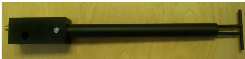
Figure 1 – MVG COMOSAR Validation Dipole
