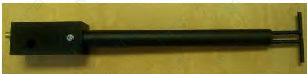
Figure 1 – MVG COMOSAR Validation Dipole
