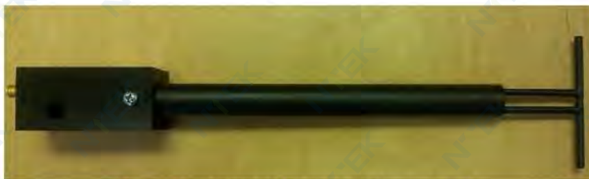
Figure 1 – MVG COMOSAR Validation Dipole
