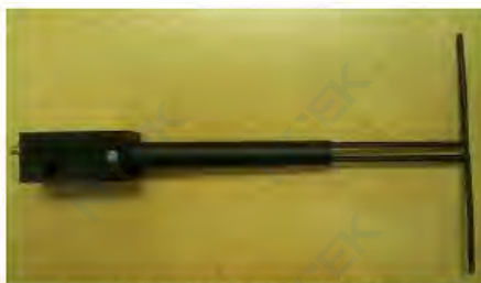
Figure 1 – MVG COMOSAR Validation Dipole
