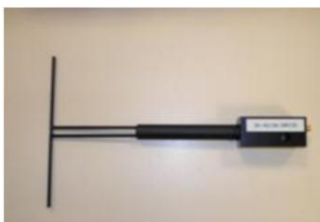
Figure 1 – Satimo COMOSAR Validation Dipole
