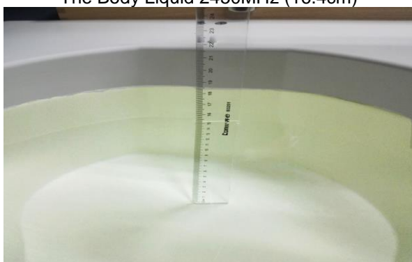
The Body Liquid of 5000-6000MHz (15.2 cm)
