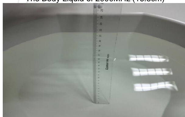
The Body Liquid of 2600MHz (16.6cm)
