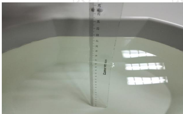
The Body Liquid of 750MHz (16.5cm)
