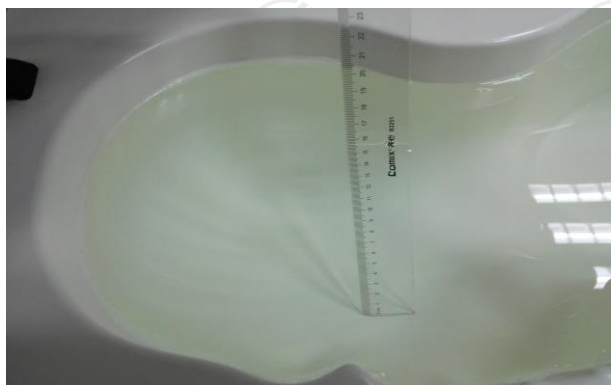
The Head Liquid of 700MHz (15.5cm)
