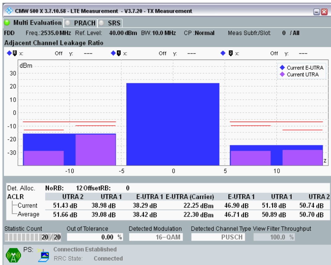
Band7 QAM16 BW=10MHz Channel=21100 RB Size=12 Position=#Max.png
