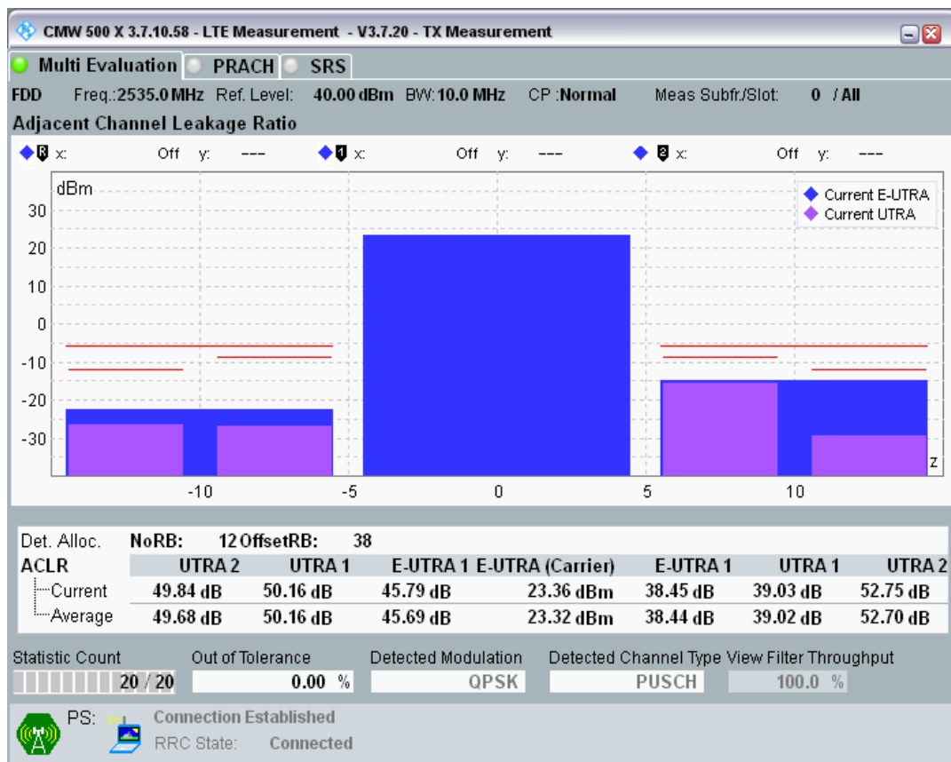
Band7 QPSK BW=10MHz Channel=21100 RB Size=50 Position=#0.png
