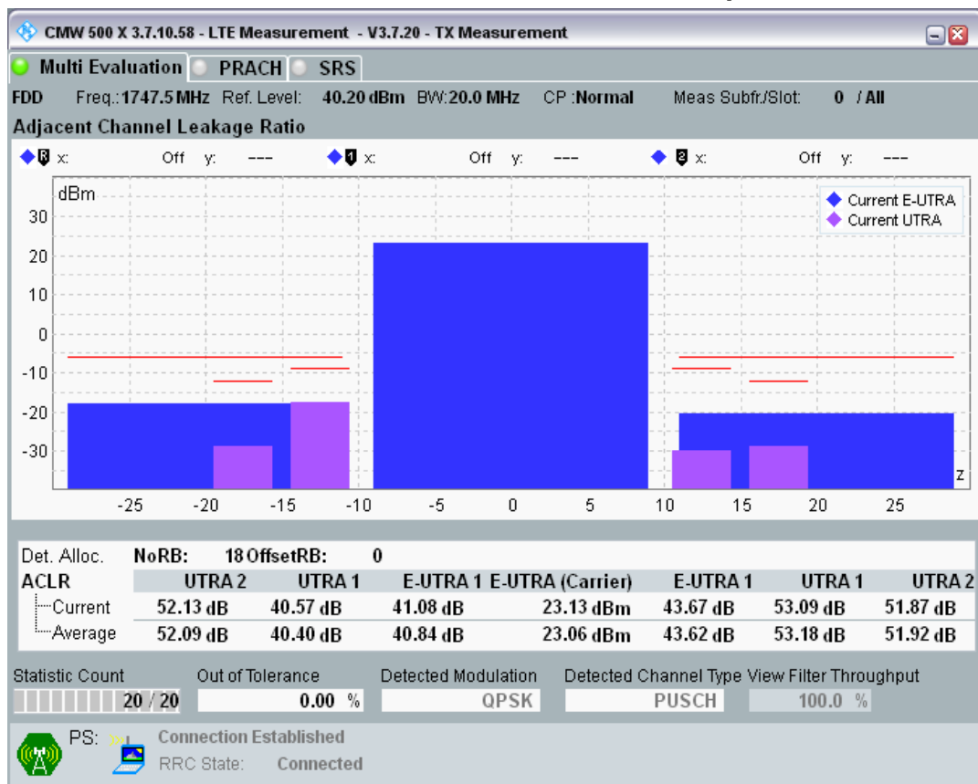
Band3 QPSK BW=20MHz Channel=19575 RB Size=18 Position=#Max.png
