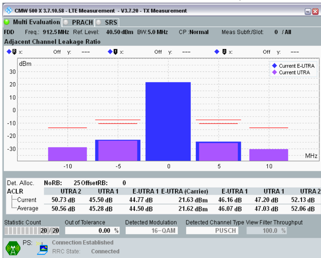
Band8 QAM16 BW=5MHz Channel=21775 RB Size=8 Position=#0.png
