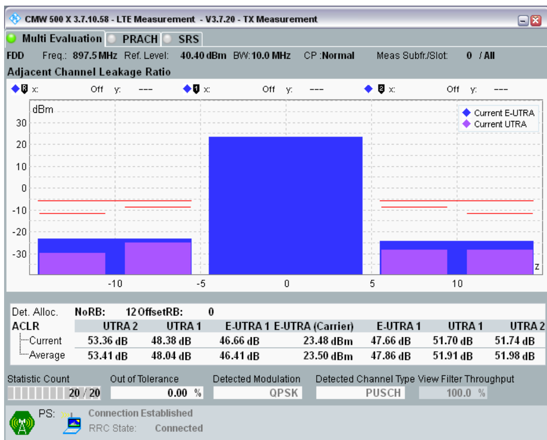
Band8 QPSK BW=10MHz Channel=21625 RB Size=12 Position=#Max.png
