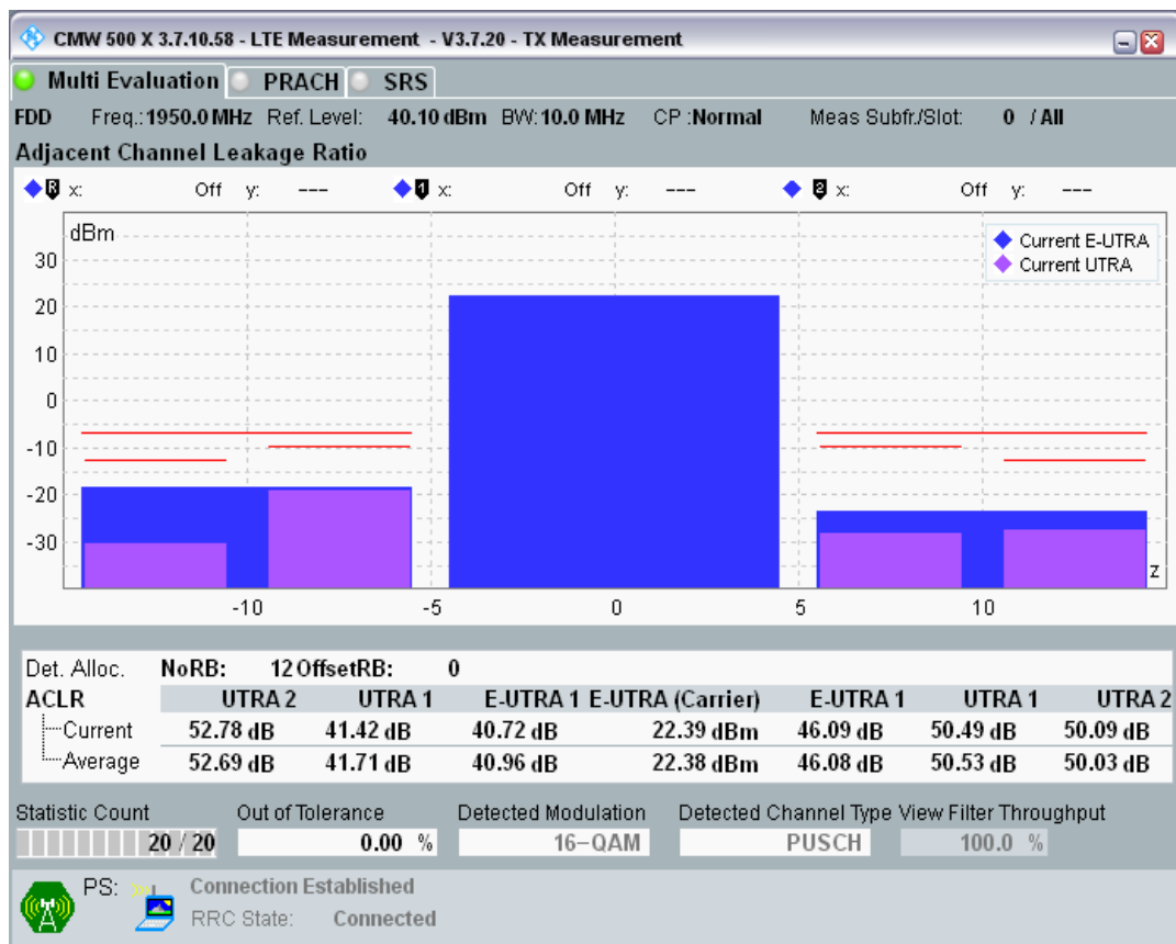
Band1 QAM16 BW=10MHz Channel=18300 RB Size=12 Position=#Max.png
