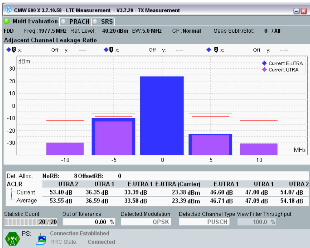
Band1 QPSK BW=5MHz Channel=18575 RB Size=8 Position=#Max.png
