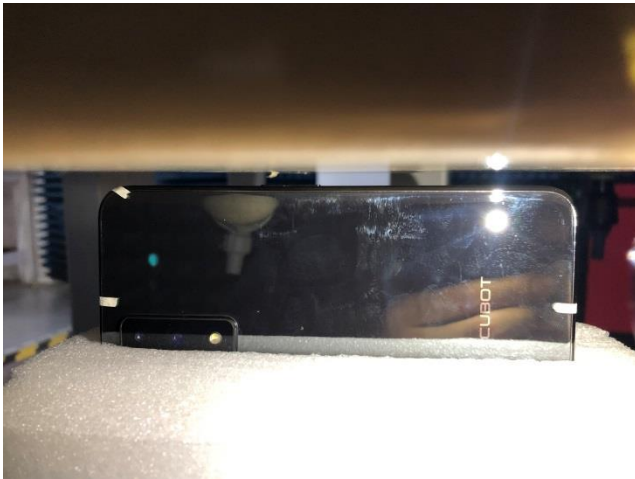
Body worn – Left (Test distance: 5mm, Thickness of DUT: 9mm)
