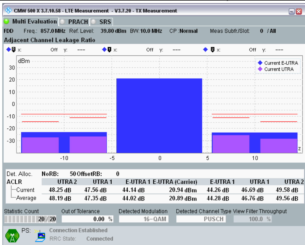
Band20 QAM16 BW=20MHz Channel=24250 RB Size=100 Position=#0.png
