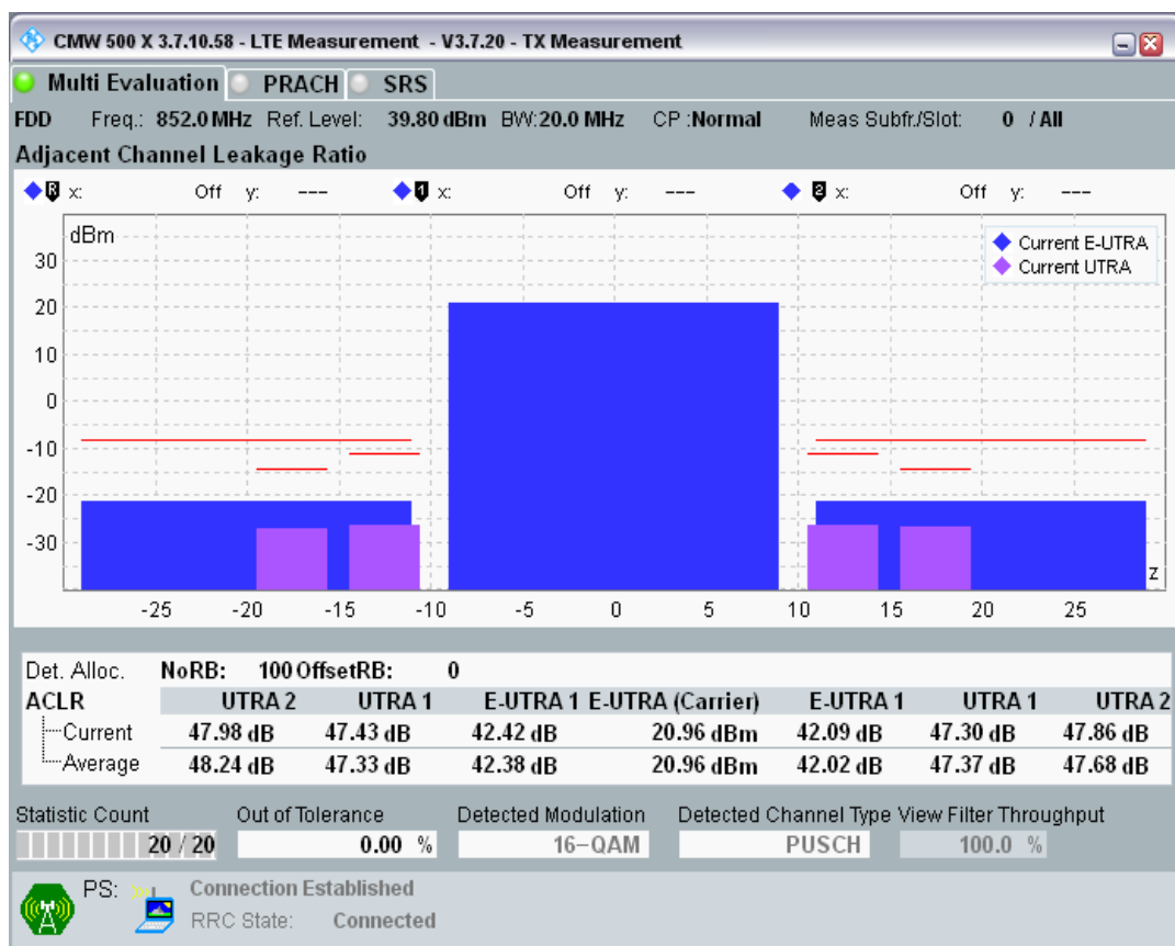
Band20 QAM16 BW=20MHz Channel=24350 RB Size=18 Position=#0.png
