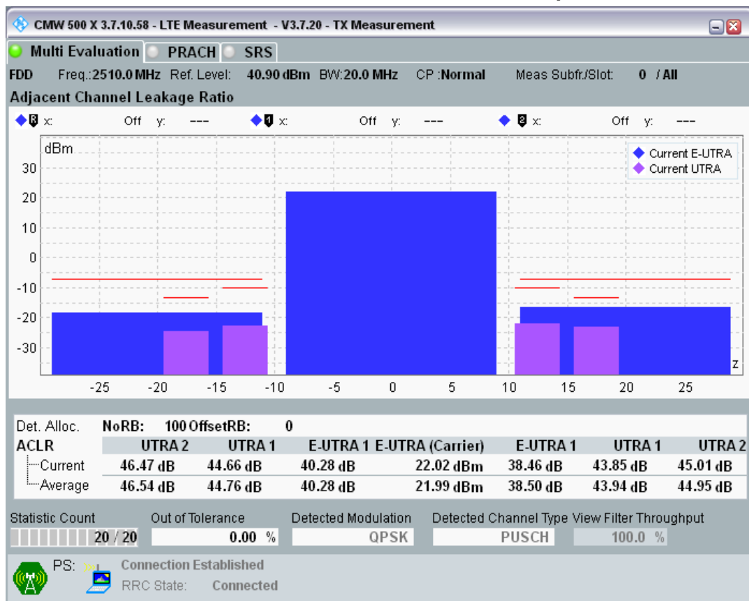
Band7 QPSK BW=20MHz Channel=20850 RB Size=18 Position=#0.png
