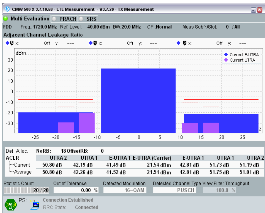
Band3 QAM16 BW=20MHz Channel=19300 RB Size=18 Position=#Max.png
