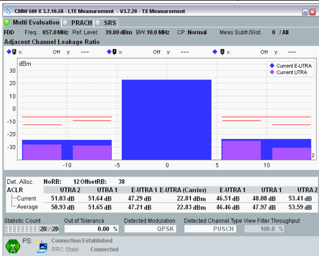
Band20 QPSK BW=10MHz Channel=24400 RB Size=50 Position=#0.png
