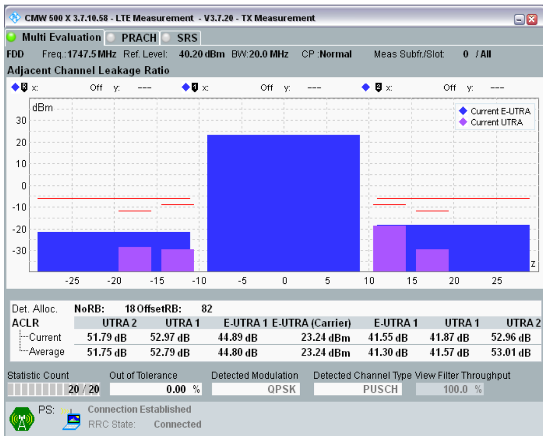
Band3 QPSK BW=20MHz Channel=19850 RB Size=100 Position=#0.png
