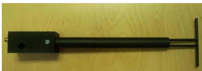
Figure 1 – MVG COMOSAR Validation Dipole
