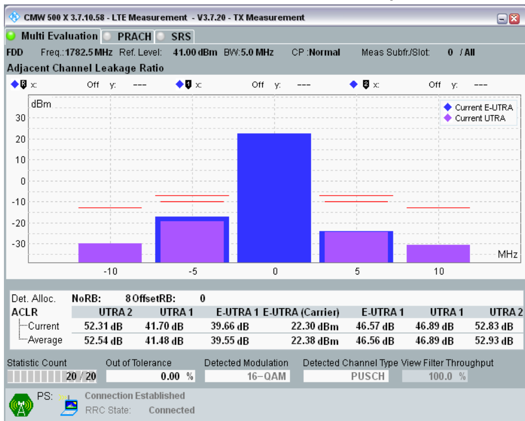
Band3 QAM16 BW=5MHz Channel=19925 RB Size=8 Position=#Max.png
