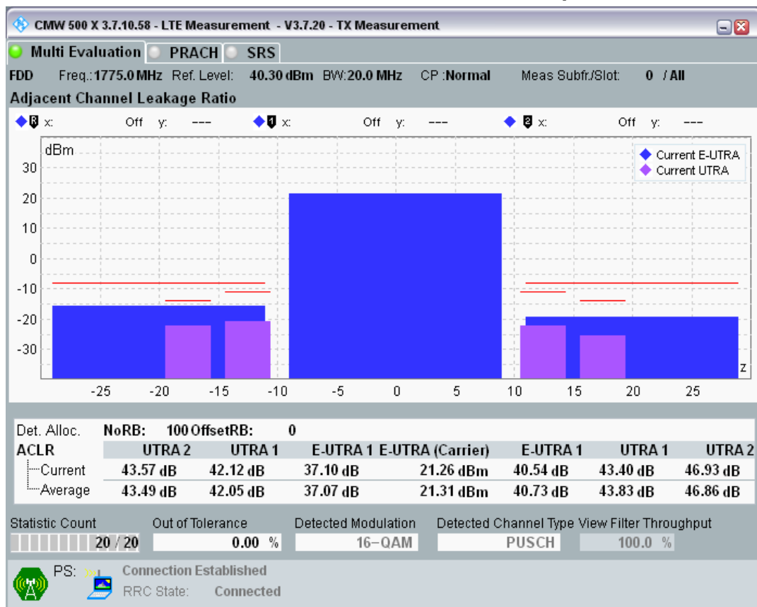
Band3 QAM16 BW=20MHz Channel=19850 RB Size=18 Position=#0.png
