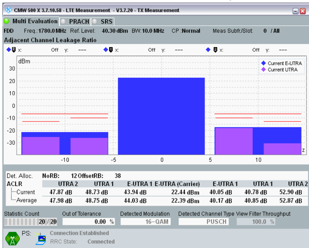
Band3 QAM16 BW=10MHz Channel=19900 RB Size=50 Position=#0.png
