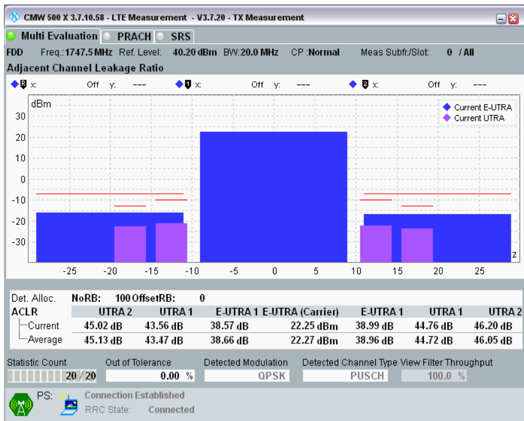
Band3 QPSK BW=20MHz Channel=19575 RB Size=18 Position=#0.png
