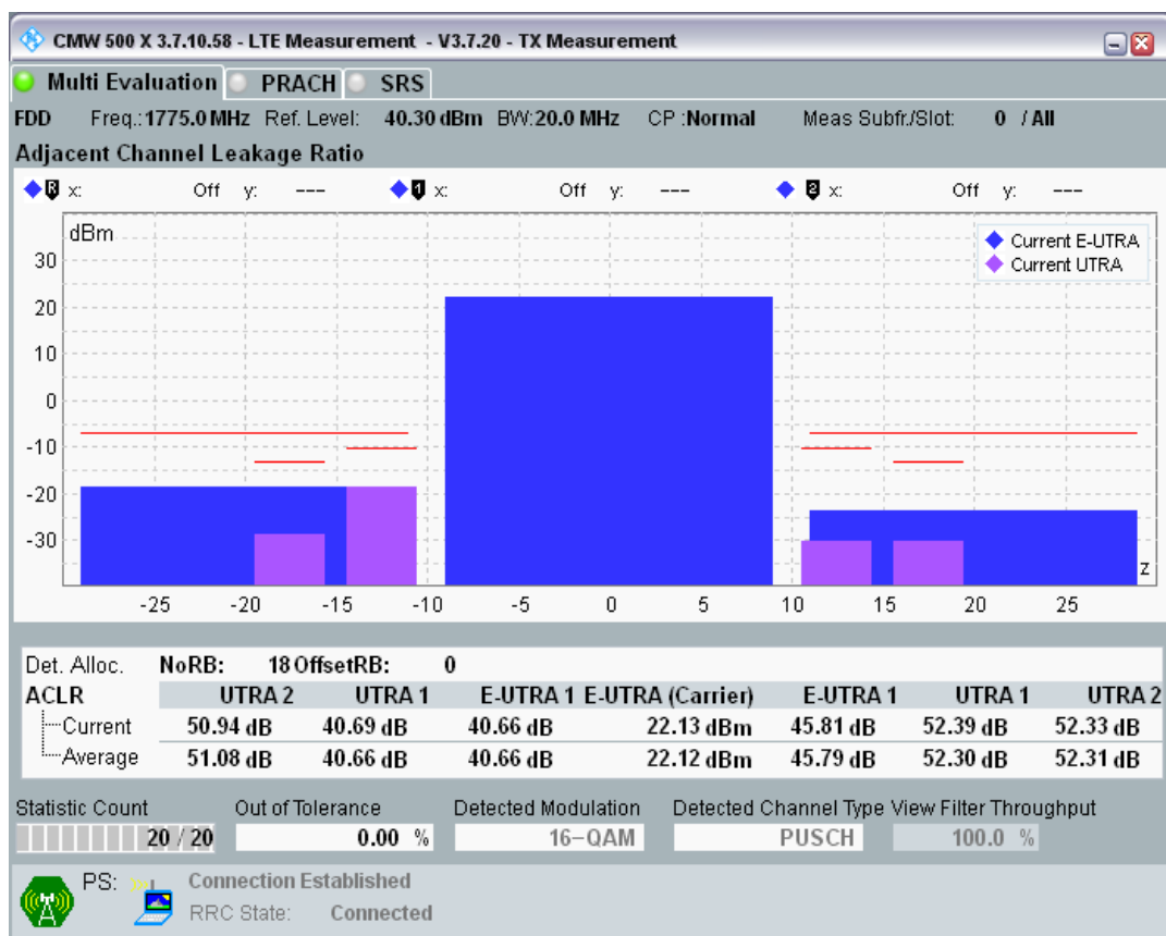
Band3 QAM16 BW=20MHz Channel=19850 RB Size=18 Position=#Max.png
