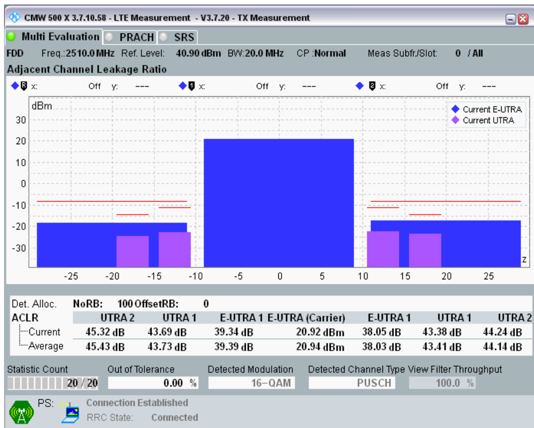
Band7 QAM16 BW=20MHz Channel=20850 RB Size=18 Position=#0.png
