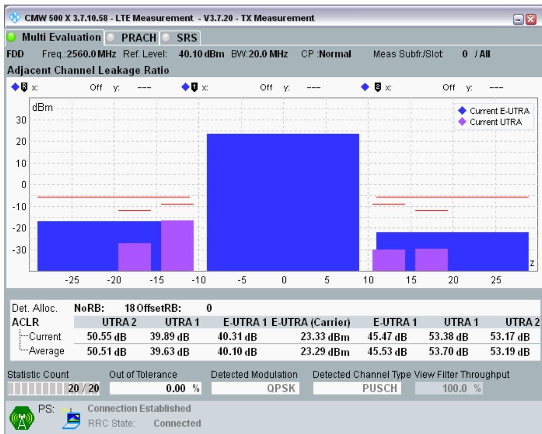
Band7 QPSK BW=20MHz Channel=21350 RB Size=18 Position=#Max.png
