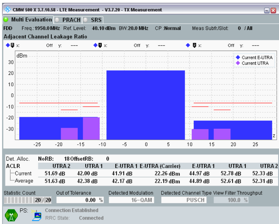
Band1 QAM16 BW=20MHz Channel=18300 RB Size=18 Position=#Max.png
