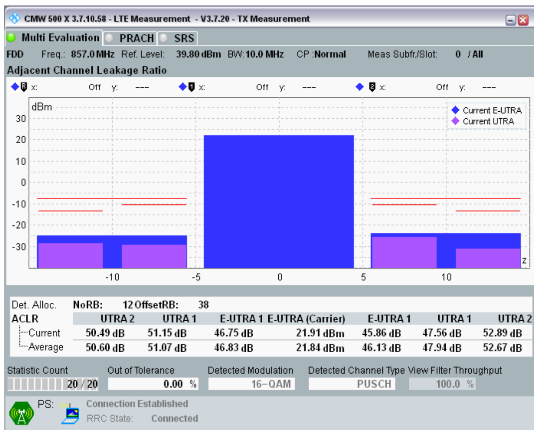
Band20 QAM16 BW=10MHz Channel=24400 RB Size=50 Position=#0.png
