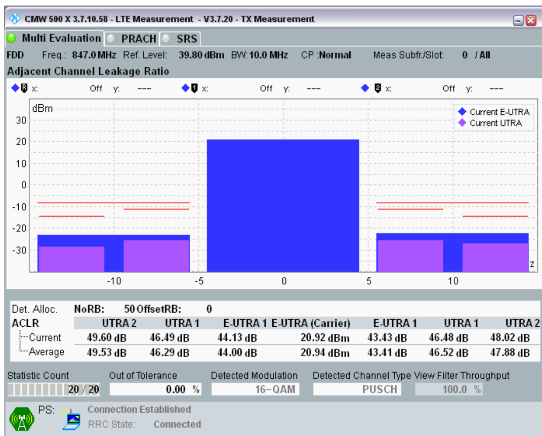
Band20 QAM16 BW=10MHz Channel=24400 RB Size=12 Position=#0.png
