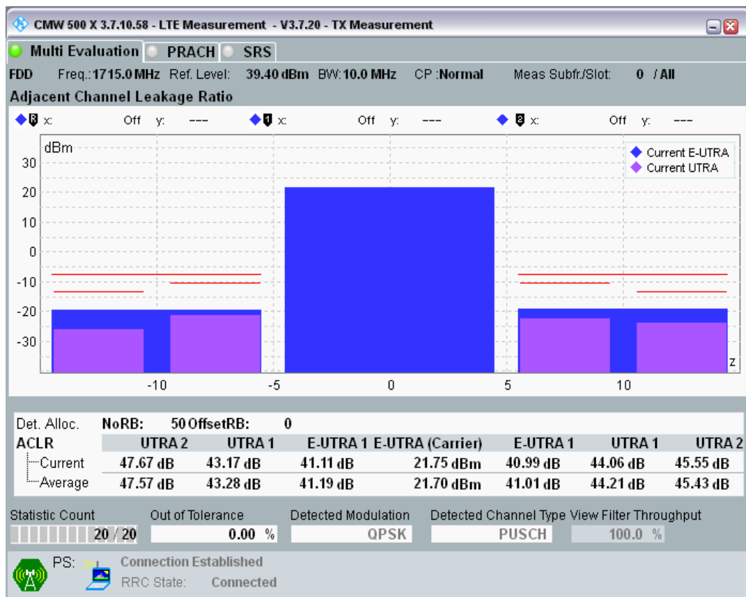
Band3 QPSK BW=10MHz Channel=19575 RB Size=12 Position=#0.png
