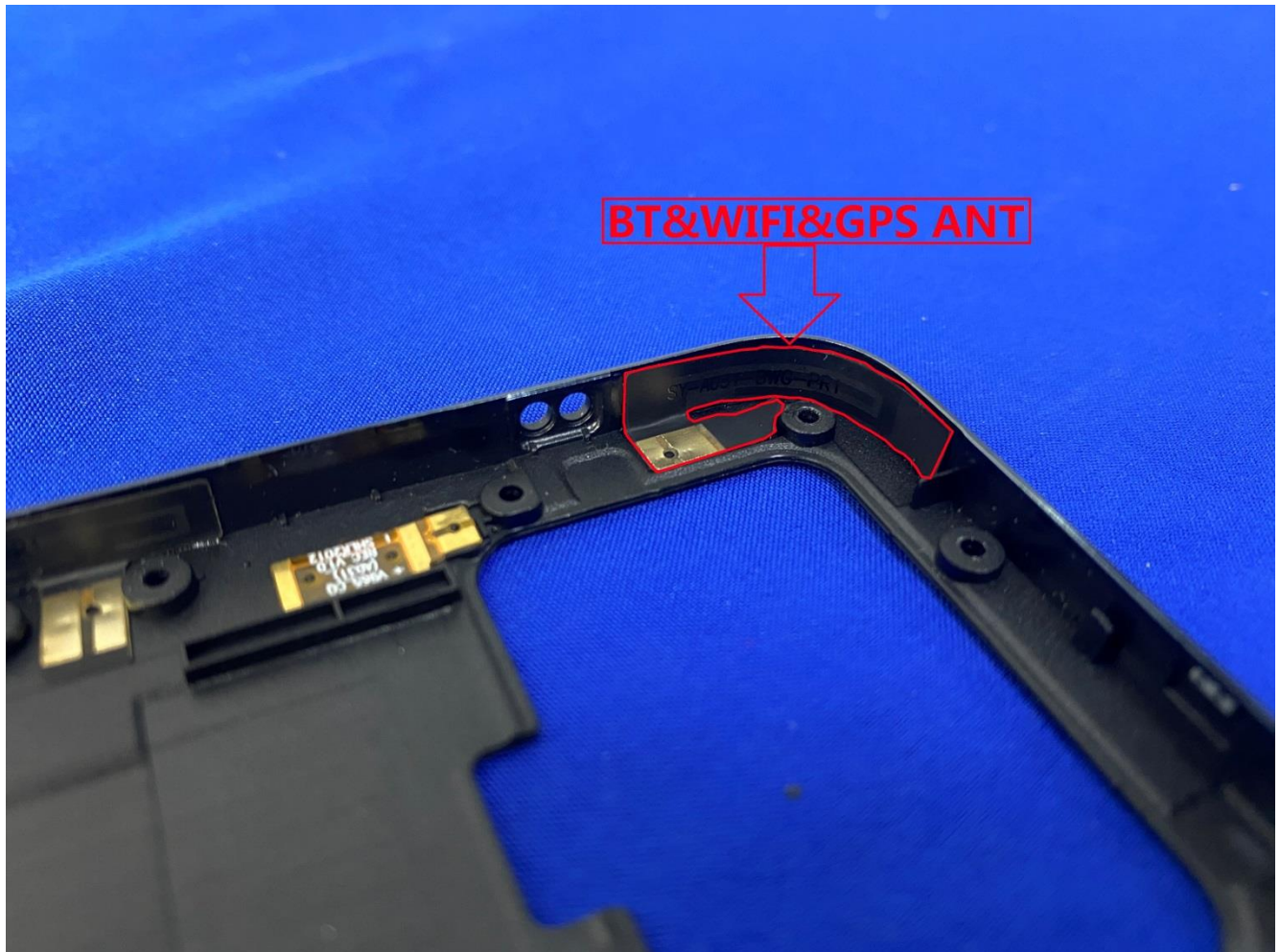
Fig.14.1 EUT Antenna Locations
