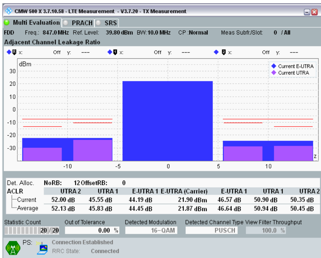
Band20 QAM16 BW=10MHz Channel=24300 RB Size=12 Position=#Max.png
