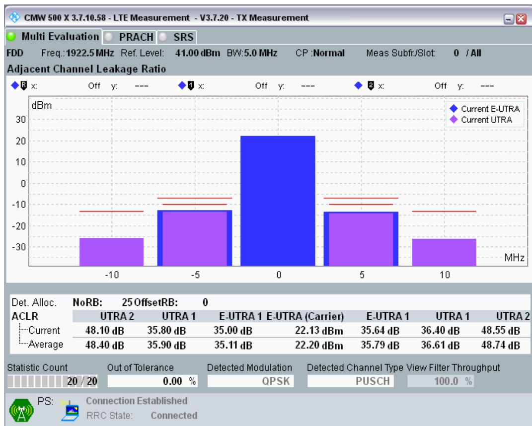
Band1 QPSK BW=5MHz Channel=18025 RB Size=8 Position=#0.png
