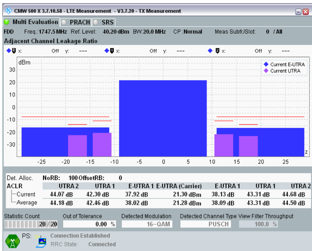
Band3 QAM16 BW=20MHz Channel=19575 RB Size=18 Position=#0.png
