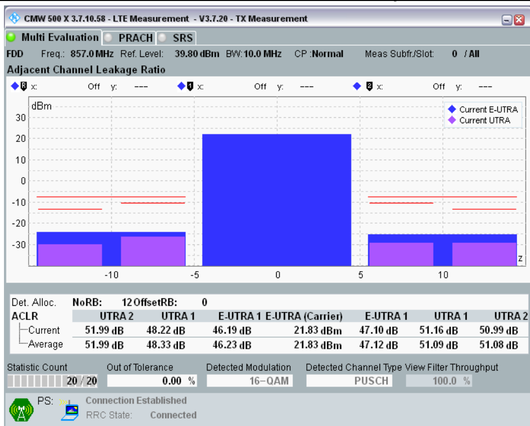
Band20 QAM16 BW=10MHz Channel=24400 RB Size=12 Position=#Max.png
