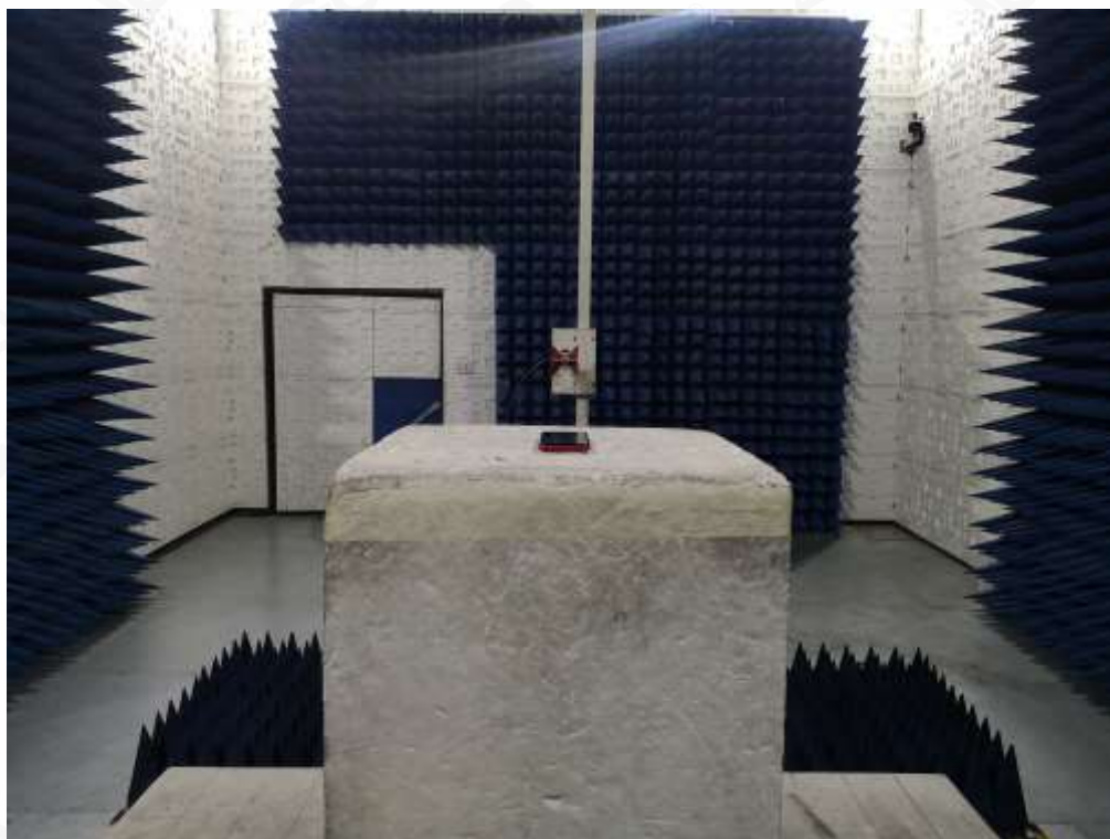
RADIATED SPURIOUS EMISSION ABOVE 1G TEST SETUP
