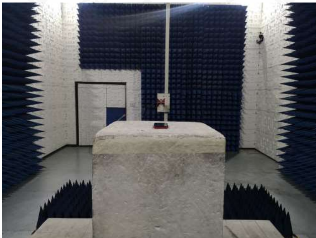
RADIATED SPURIOUS EMISSION ABOVE 1G TEST SETUP
