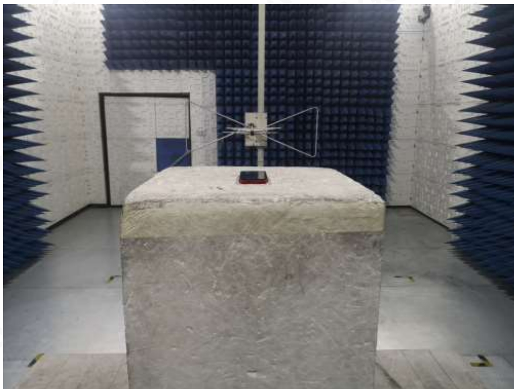
RADIATED SPURIOUS EMISSION ABOVE 1G TEST SETUP
