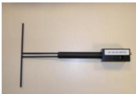
Figure 1 – Satimo COMOSAR Validation Dipole
