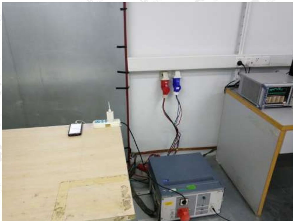
EN 55032 RADIATED EMISSION TEST SETUP
