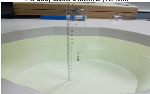
The Body Liquid of 1800MHz (16.3cm)
