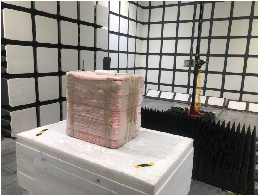
Radiated Spurious Emissions Test View (Above 1GHz)
