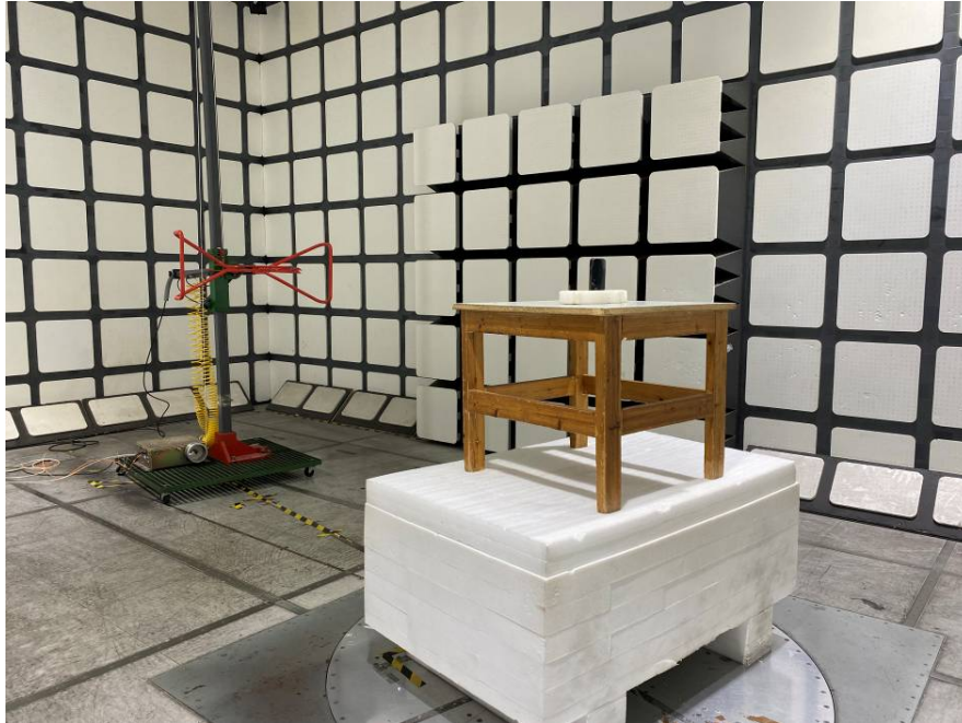
Radiated Spurious Emissions Test View (Above 1GHz)
