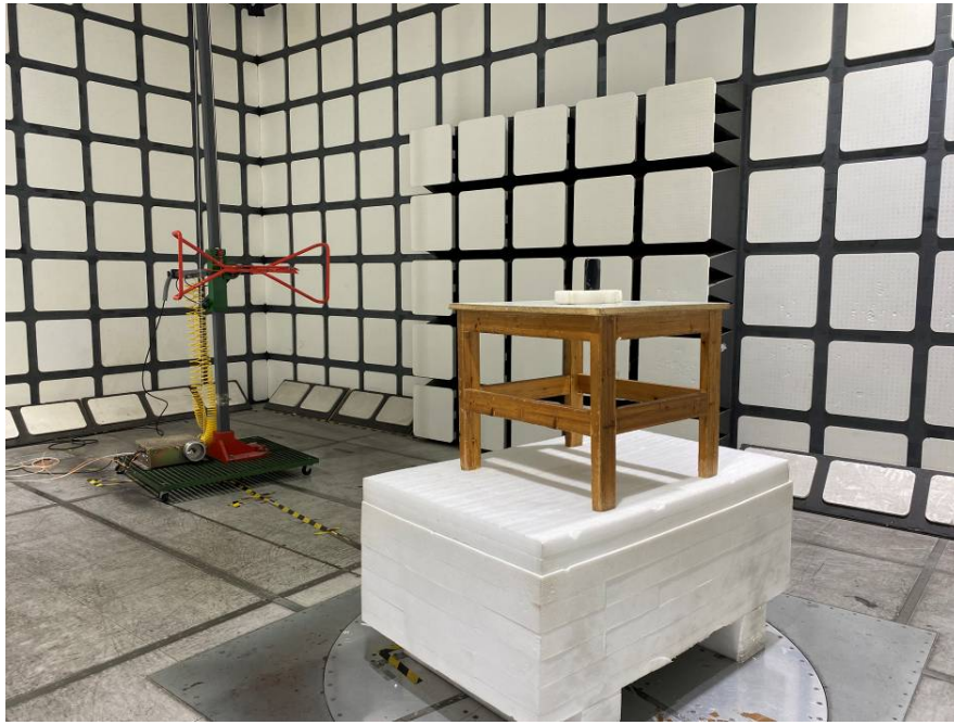
Radiated Spurious Emissions Test View (Above 1GHz)
