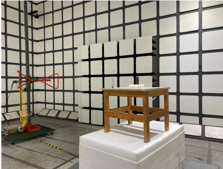
Radiated Spurious Emissions Test View (Above 1GHz)
