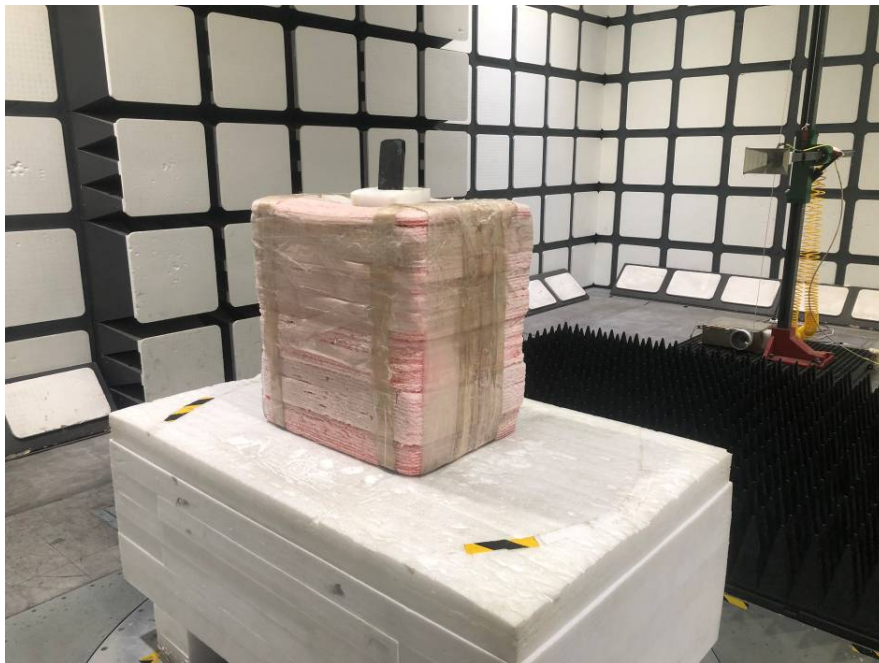
Radiated Spurious Emissions Test View (Above 1GHz)
