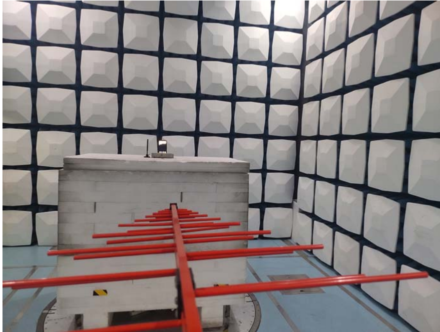
Radiated Spurious Emissions Test View (Above 1GHz)
