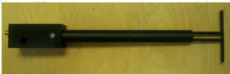
Figure 1 – MVG COMOSAR Validation Dipole
