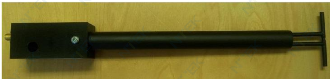
Figure 1 – MVG COMOSAR Validation Dipole
