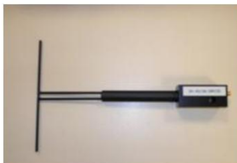
Figure 1 – Satimo COMOSAR Validation Dipole
