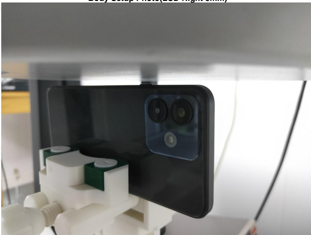
Body Setup Photo(LCD Right 5mm)
