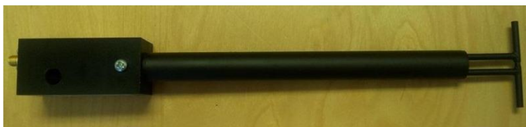
Figure 1 – MVG COMOSAR Validation Dipole
