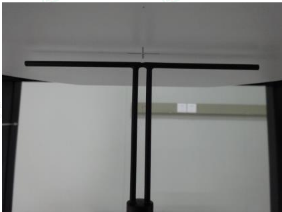
Photo of Dipole Setup
