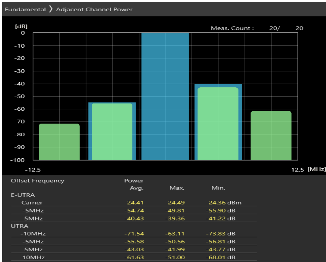
Band20 QPSK BW=5MHz Channel=24175 RB Size=25 Position=#0
