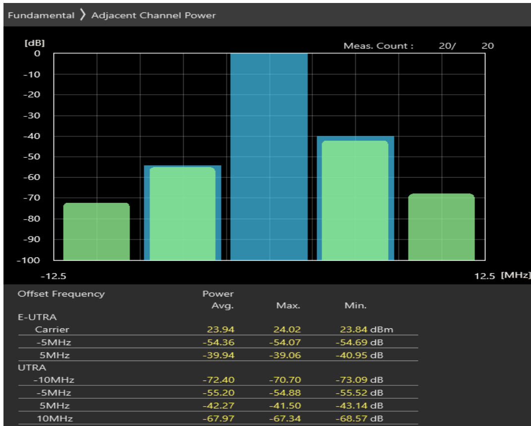
Band8 QPSK BW=5MHz Channel=21625 RB Size=25 Position=#0
