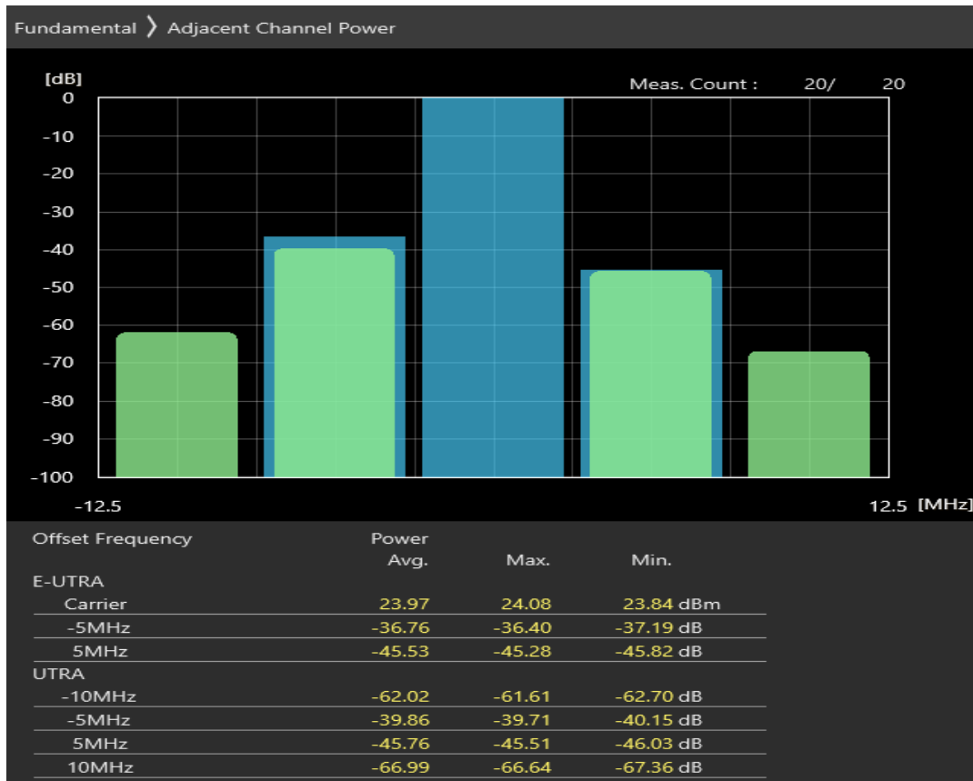
Band7 QAM16 BW=5MHz Channel=21100 RB Size=8 Position=#Max
