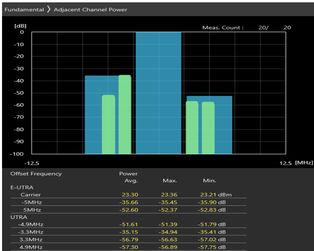
Band38 QPSK BW=5MHz Channel=38000 RB Size=8 Position=#Max
