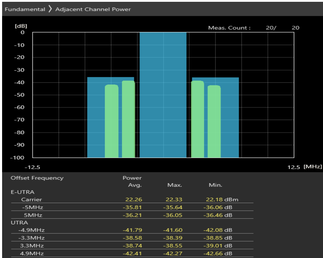
Band38 QAM16 BW=5MHz Channel=38000 RB Size=8 Position=#0
