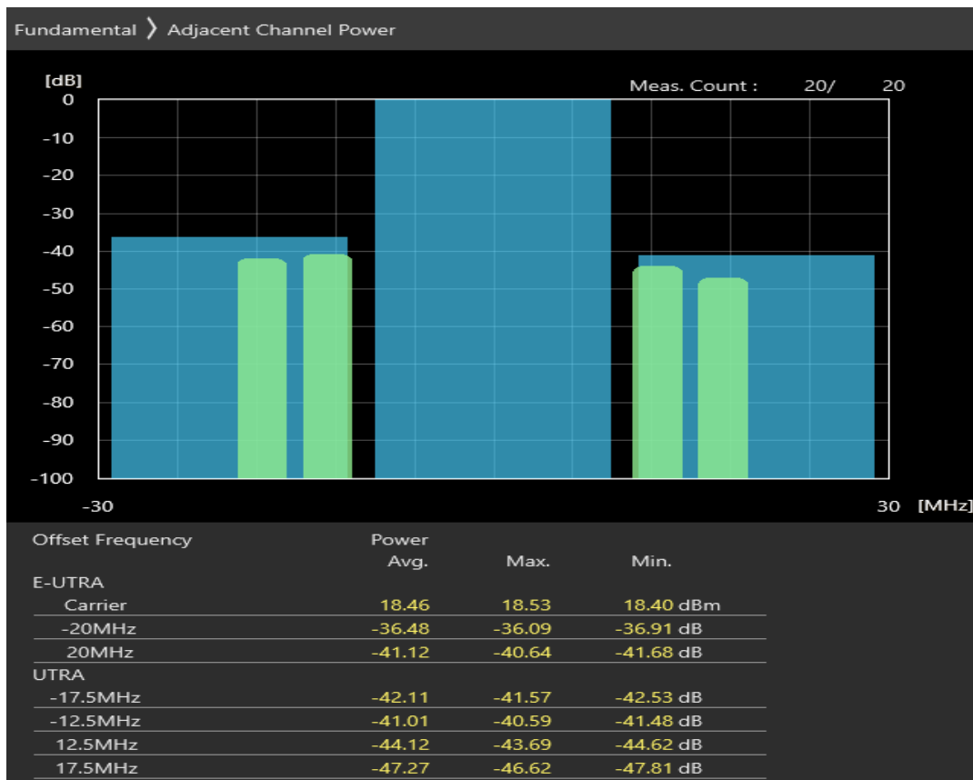
Band1 QAM16 BW=20MHz Channel=18300 RB Size=18 Position=#0
