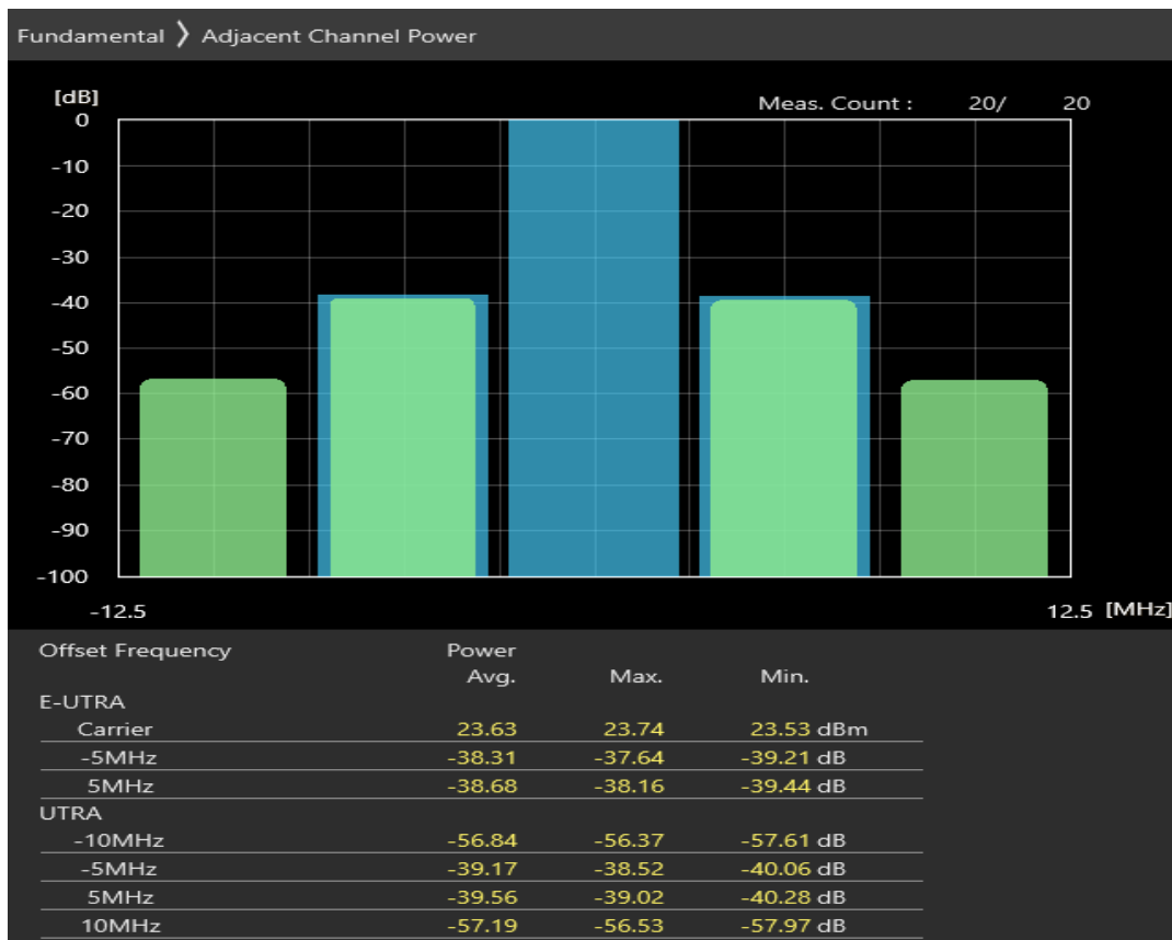
Band20 QAM16 BW=5MHz Channel=24300 RB Size=8 Position=#0
