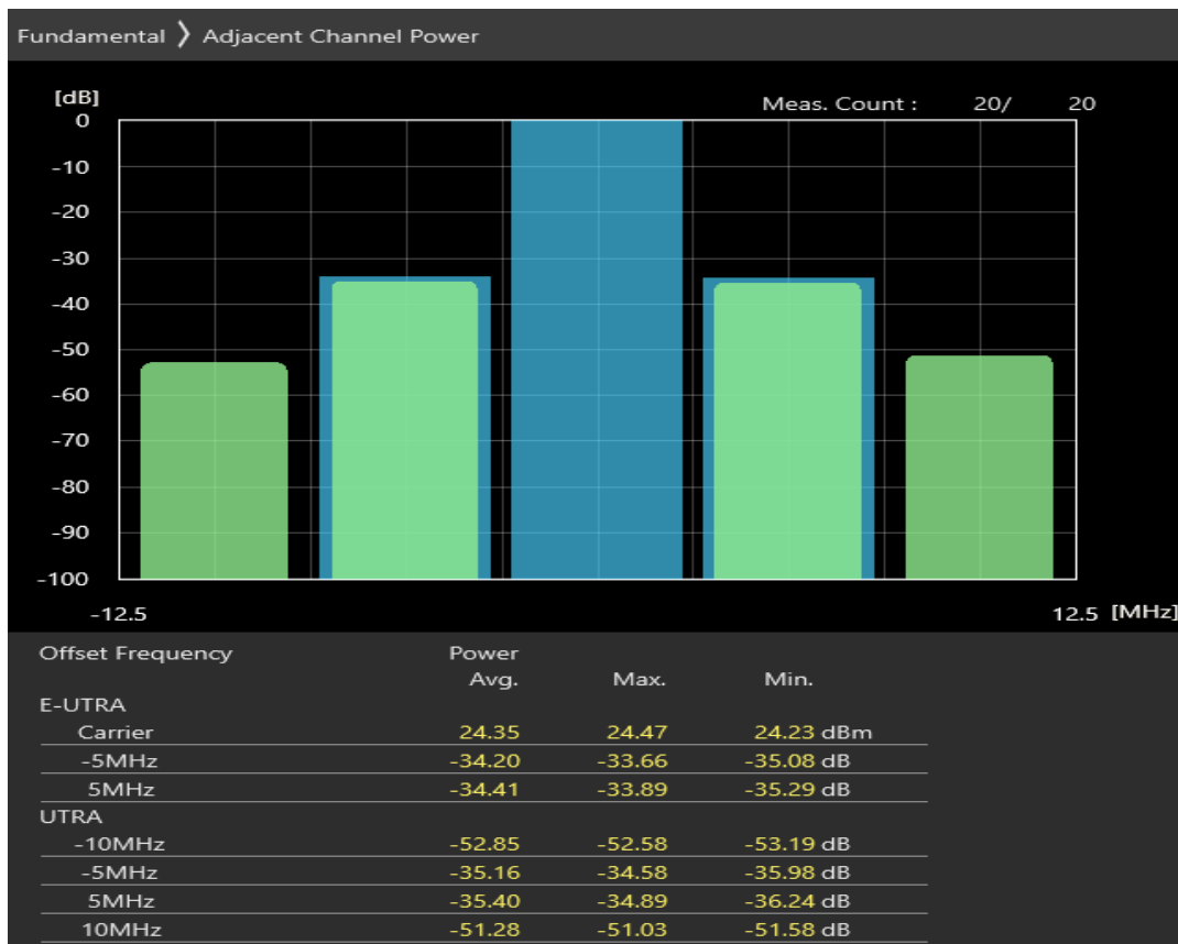
Band7 QAM16 BW=5MHz Channel=20775 RB Size=8 Position=#0
