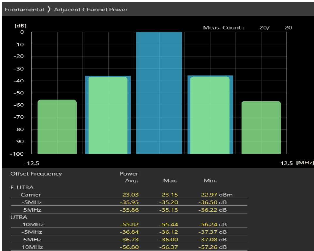
Band3 QAM16 BW=5MHz Channel=19575 RB Size=8 Position=#0
