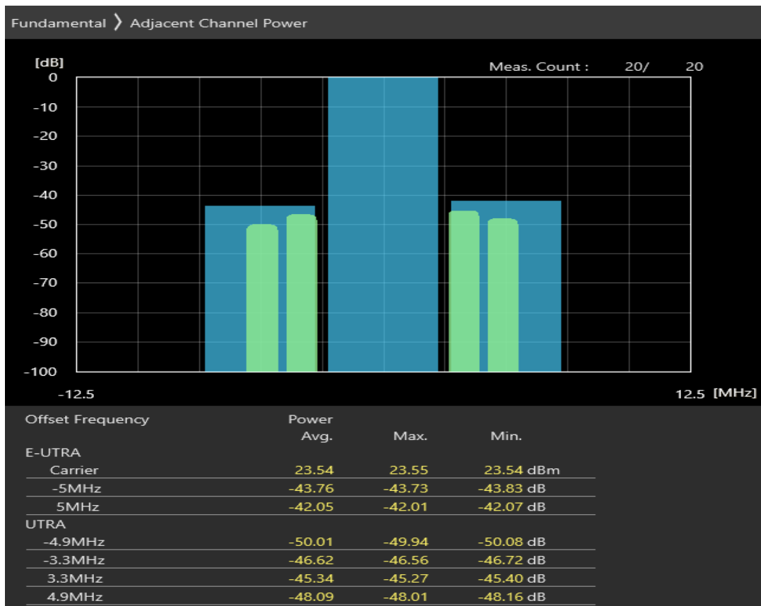
Band40 QAM16 BW=5MHz Channel=38675 RB Size=8 Position=#0
