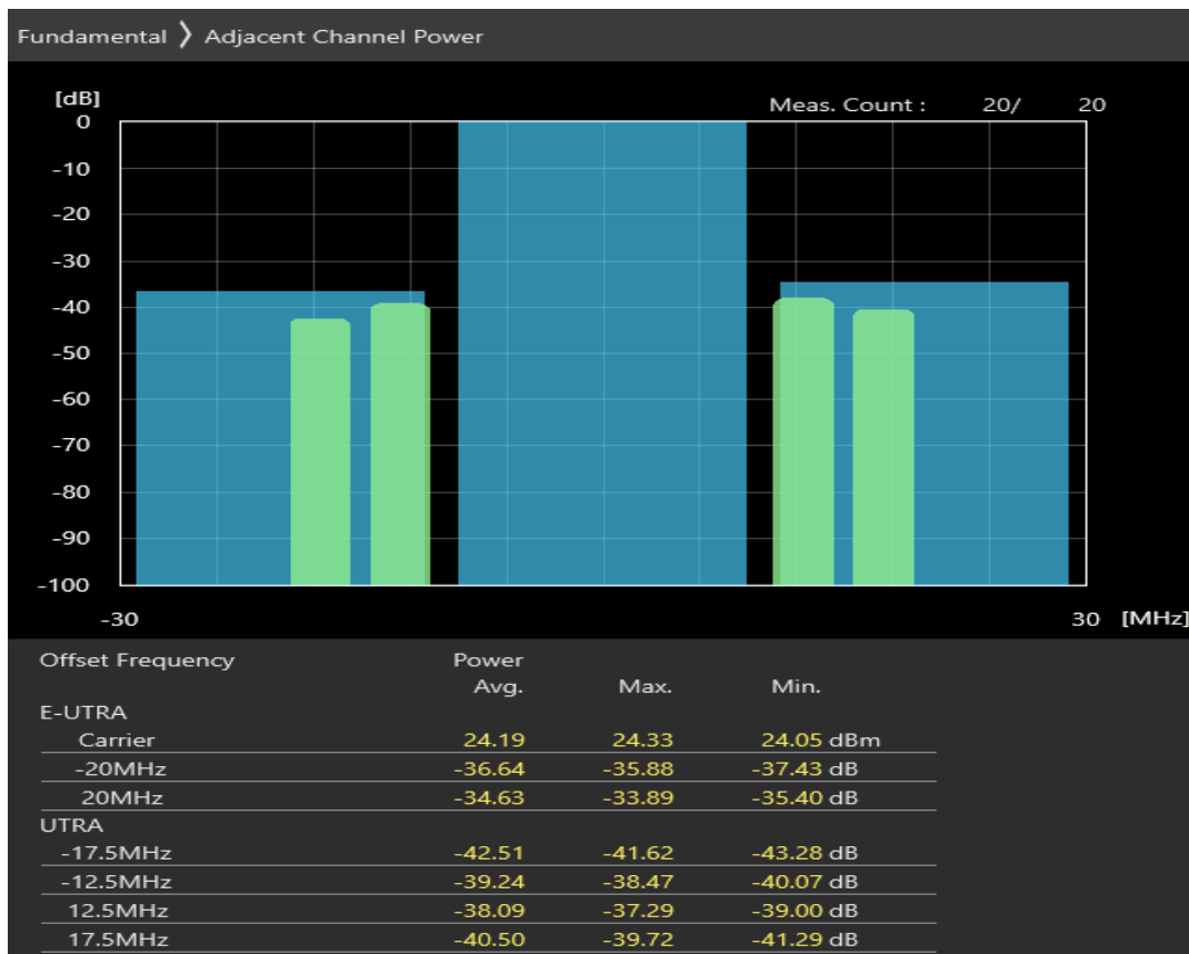
Band7 QAM16 BW=20MHz Channel=20850 RB Size=18 Position=#0
