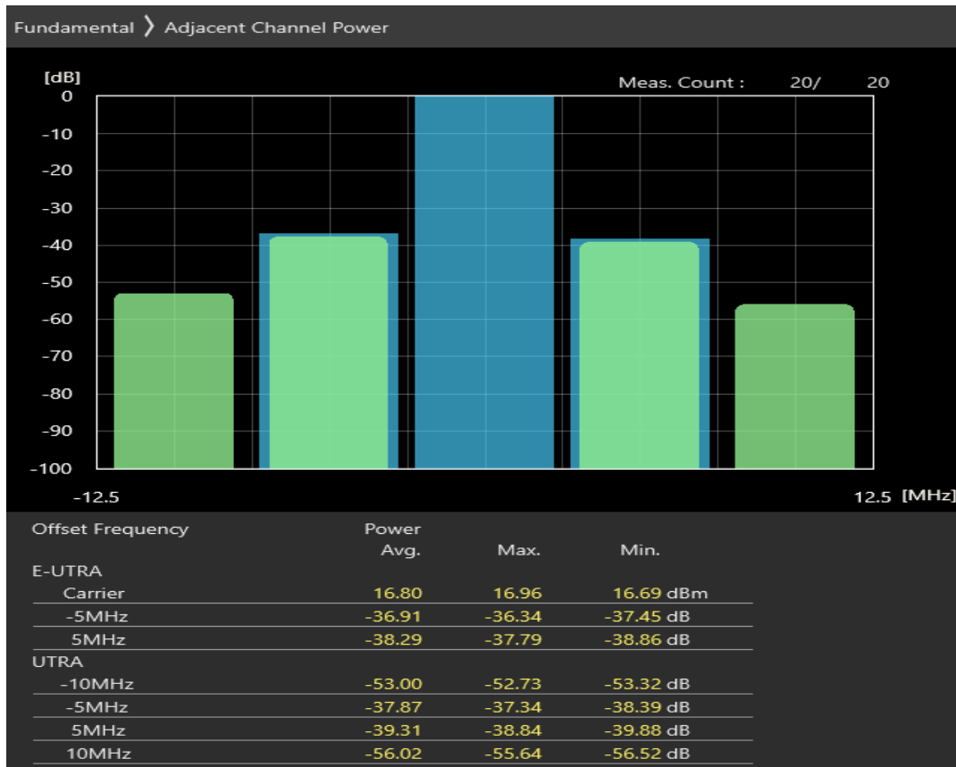
Band1 QPSK BW=10MHz Channel=18050 RB Size=12 Position=#0
