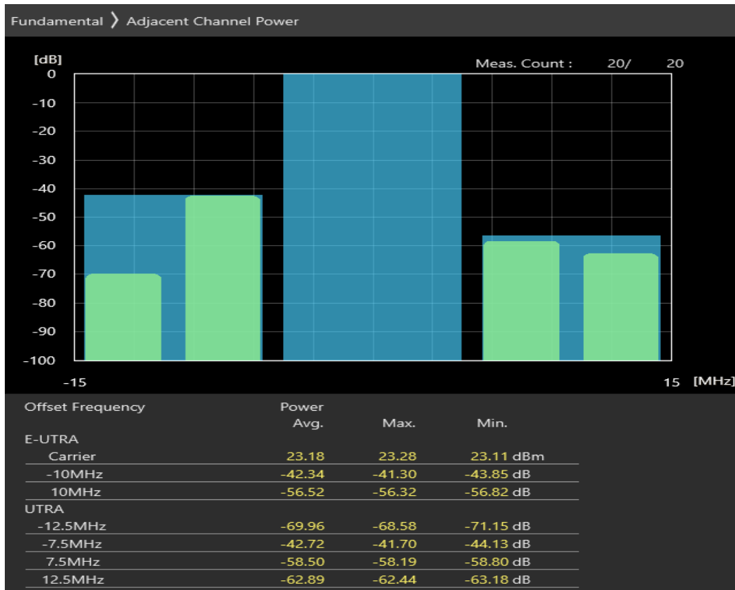
Band8 QAM16 BW=10MHz Channel=21500 RB Size=12 Position=#Max
