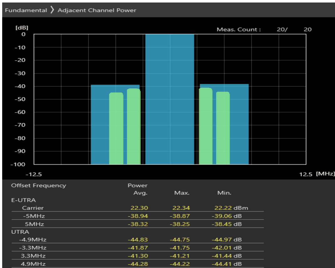
Band38 QAM16 BW=5MHz Channel=37775 RB Size=8 Position=#0
