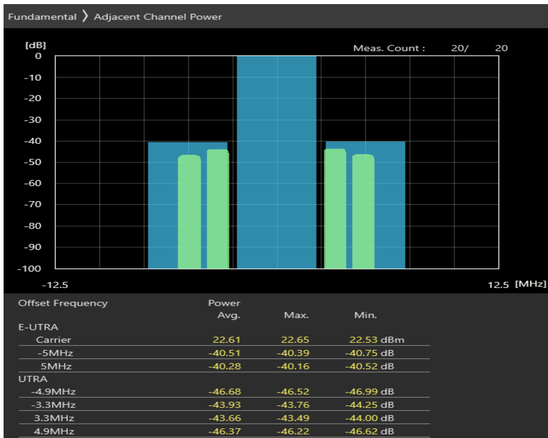
Band38 QAM16 BW=5MHz Channel=38225 RB Size=8 Position=#0
