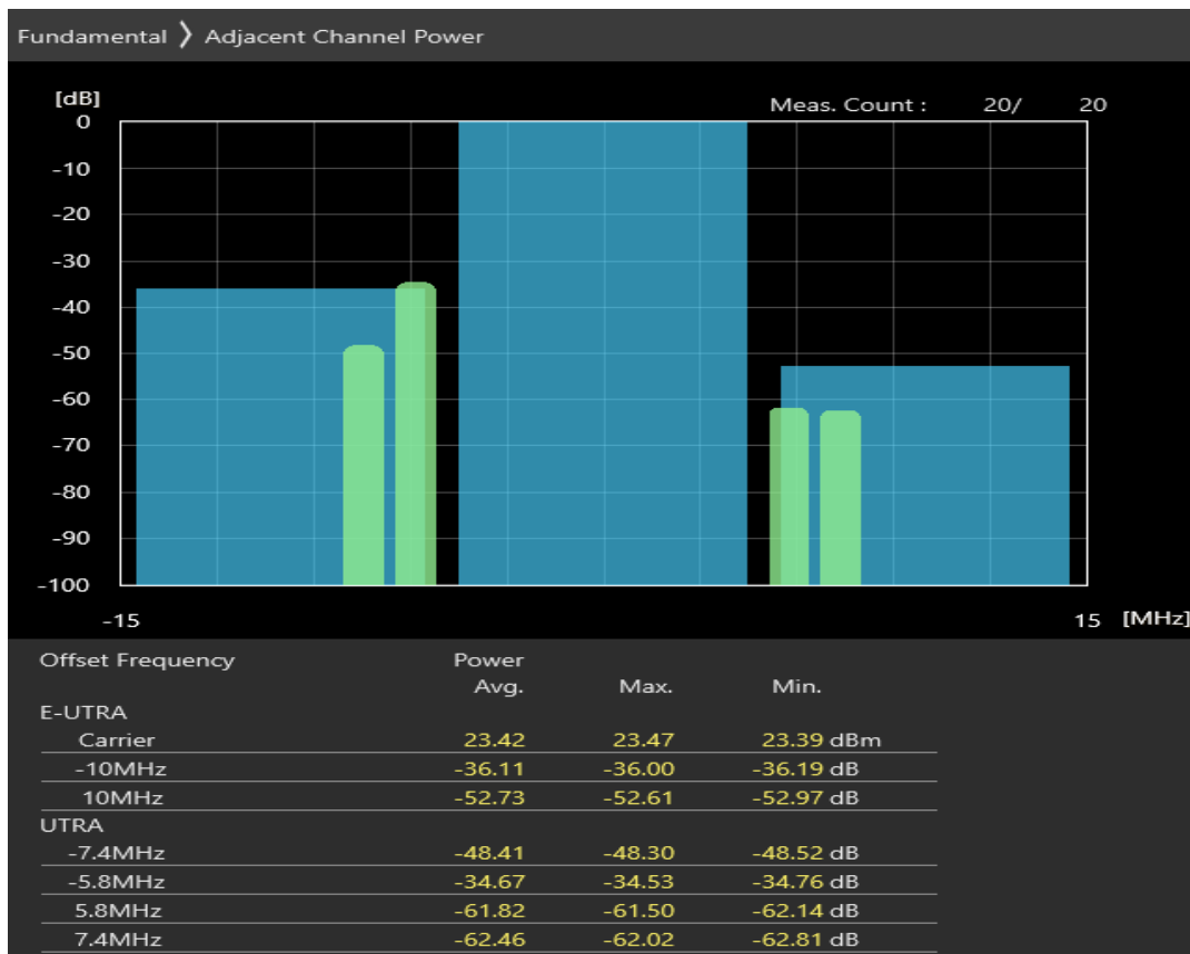
Band38 QPSK BW=10MHz Channel=38000 RB Size=12 Position=#Max
