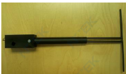
Figure 1 – MVG COMOSAR Validation Dipole
