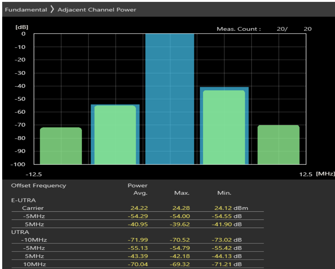
Band20 QPSK BW=5MHz Channel=24425 RB Size=25 Position=#0
