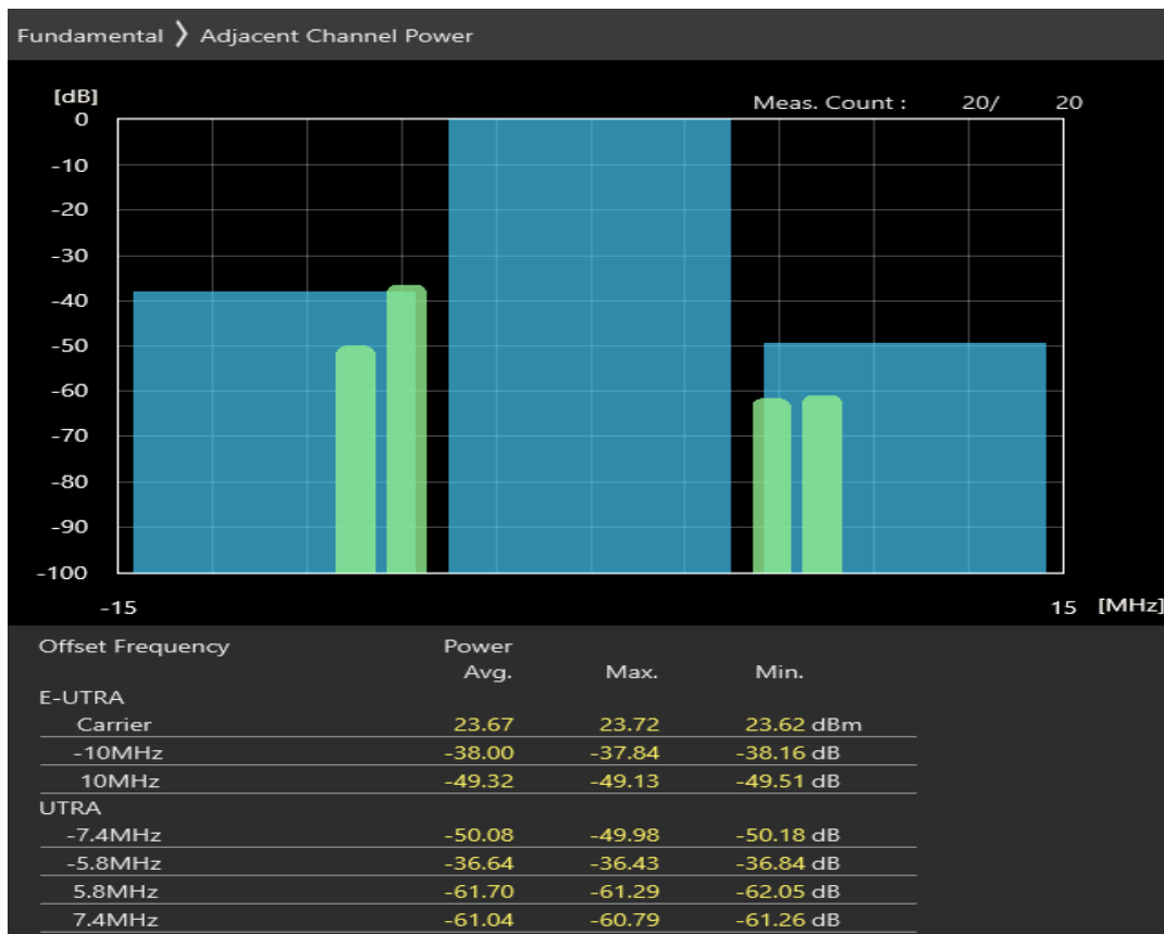
Band38 QPSK BW=10MHz Channel=38200 RB Size=12 Position=#Max
