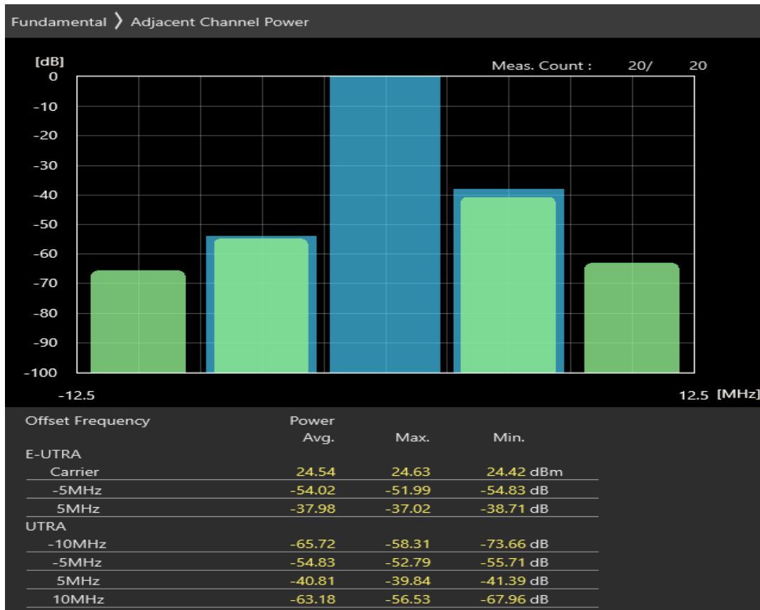
Band20 QPSK BW=5MHz Channel=24300 RB Size=25 Position=#0
