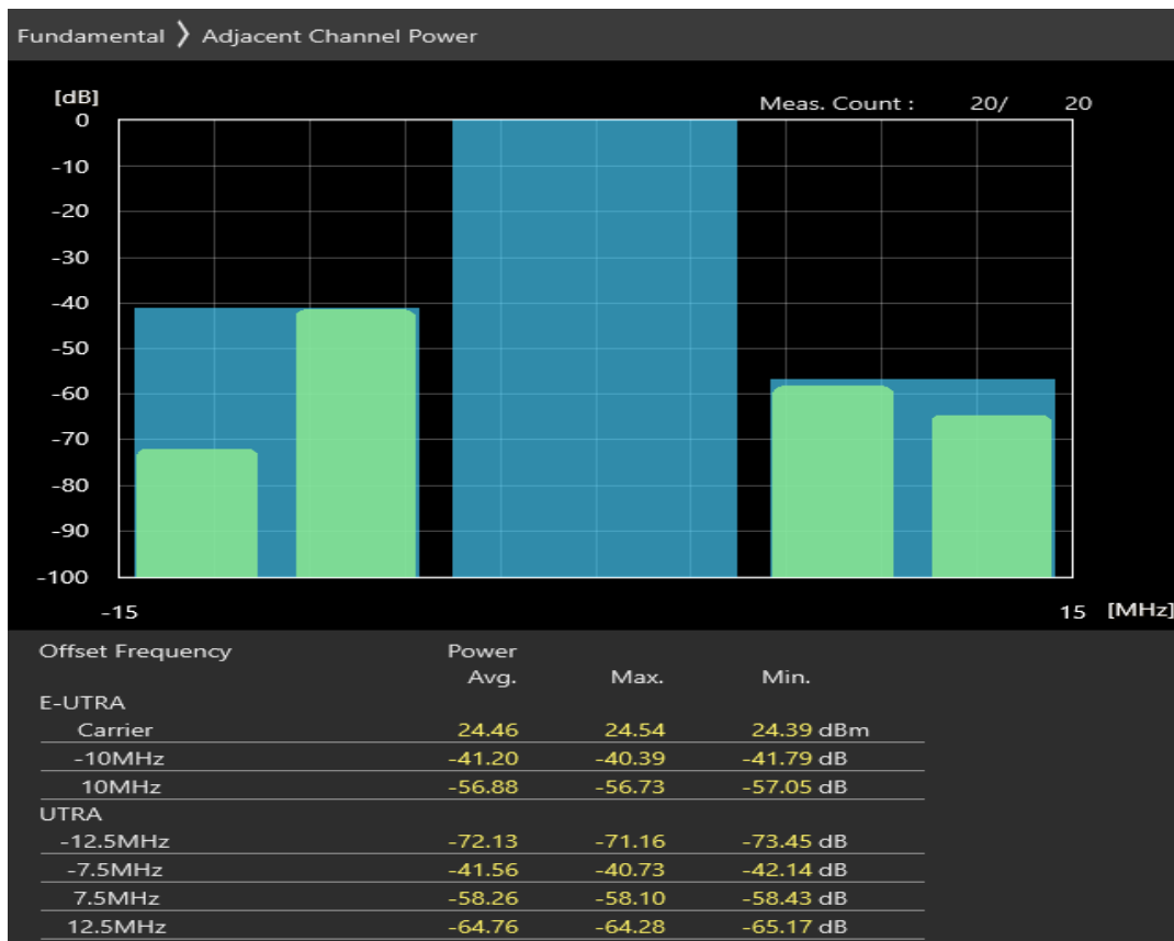
Band20 QPSK BW=10MHz Channel=24200 RB Size=12 Position=#Max
