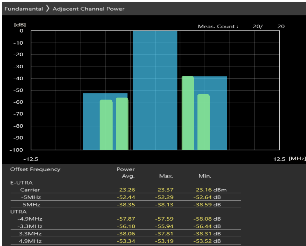
Band38 QPSK BW=5MHz Channel=37775 RB Size=25 Position=#0
