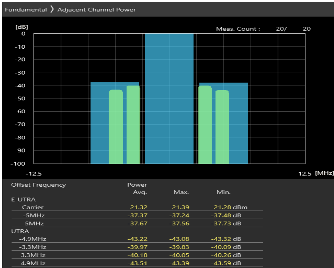
Band38 QPSK BW=5MHz Channel=38225 RB Size=8 Position=#0
