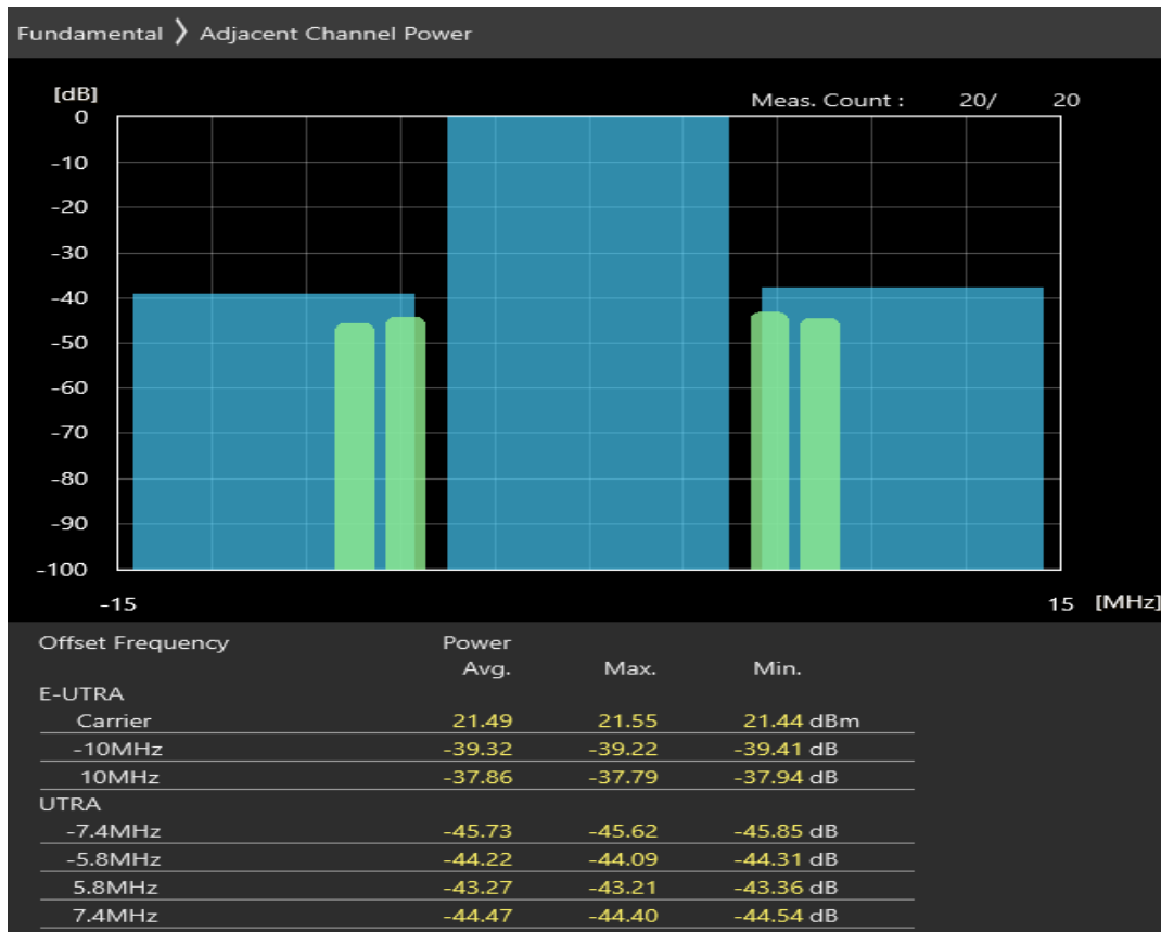
Band38 QPSK BW=10MHz Channel=38000 RB Size=12 Position=#0
