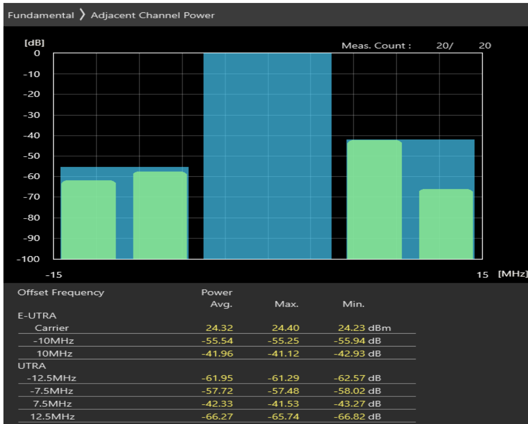
Band20 QPSK BW=10MHz Channel=24400 RB Size=50 Position=#0
