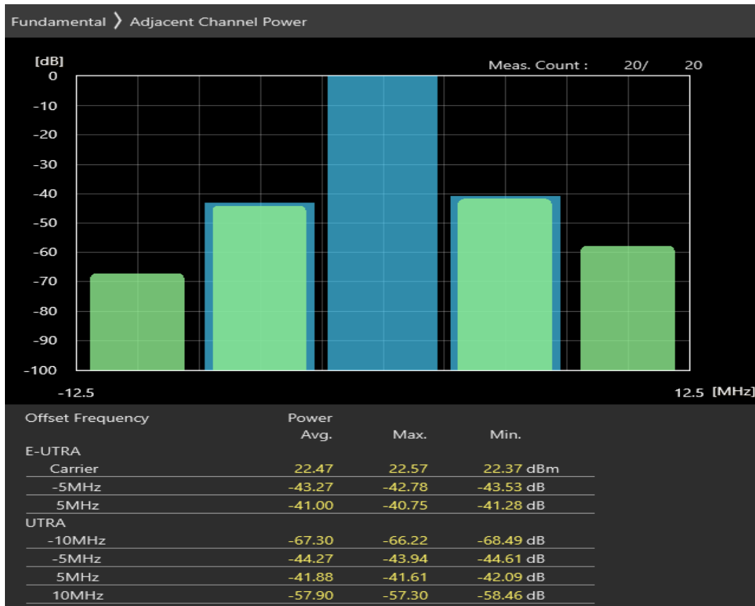
Band20 QPSK BW=5MHz Channel=24300 RB Size=8 Position=#0
