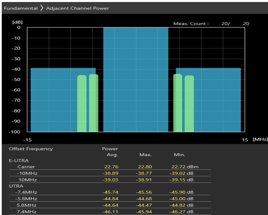
Band38 QAM16 BW=10MHz Channel=38200 RB Size=12 Position=#0
