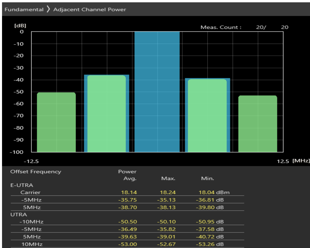
Band1 QAM16 BW=5MHz Channel=18300 RB Size=8 Position=#0
