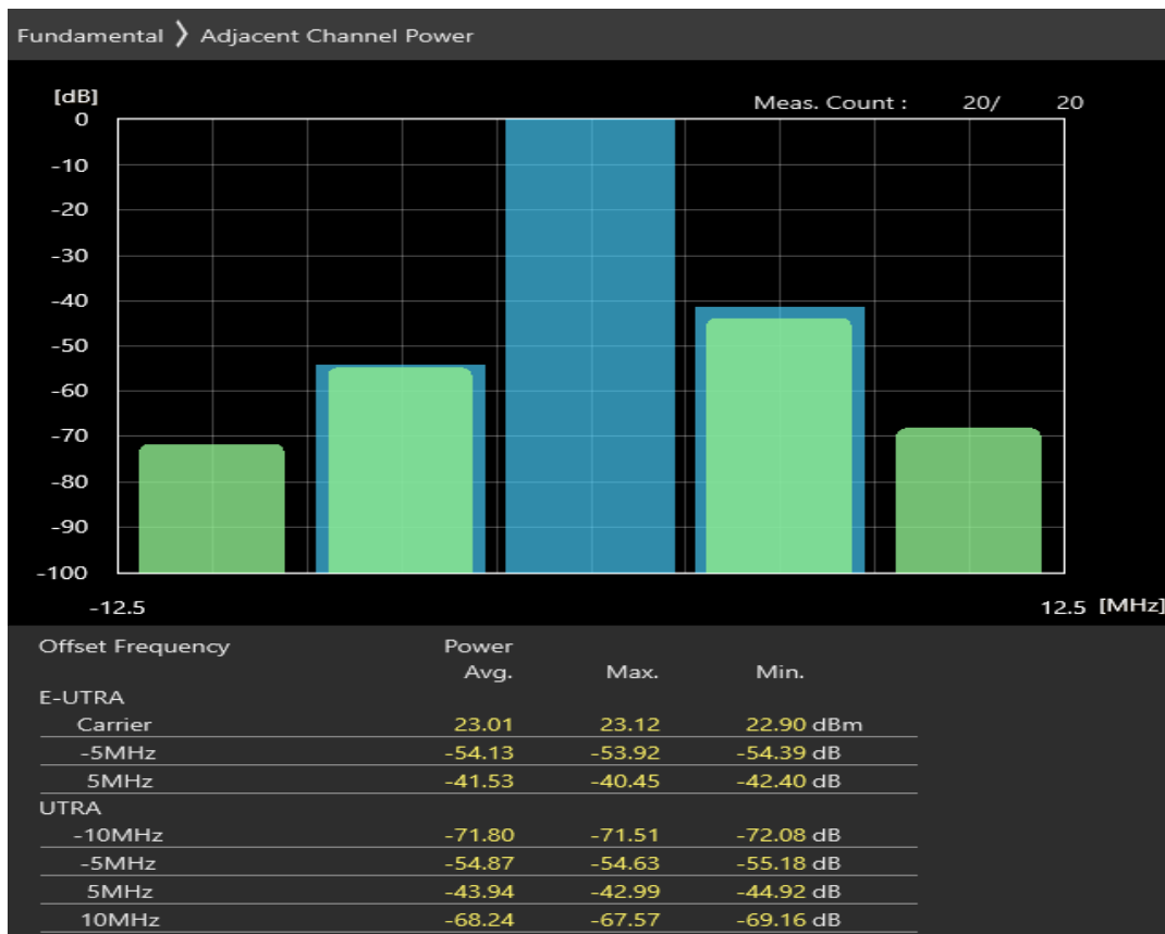
Band8 QAM16 BW=5MHz Channel=21625 RB Size=25 Position=#0
