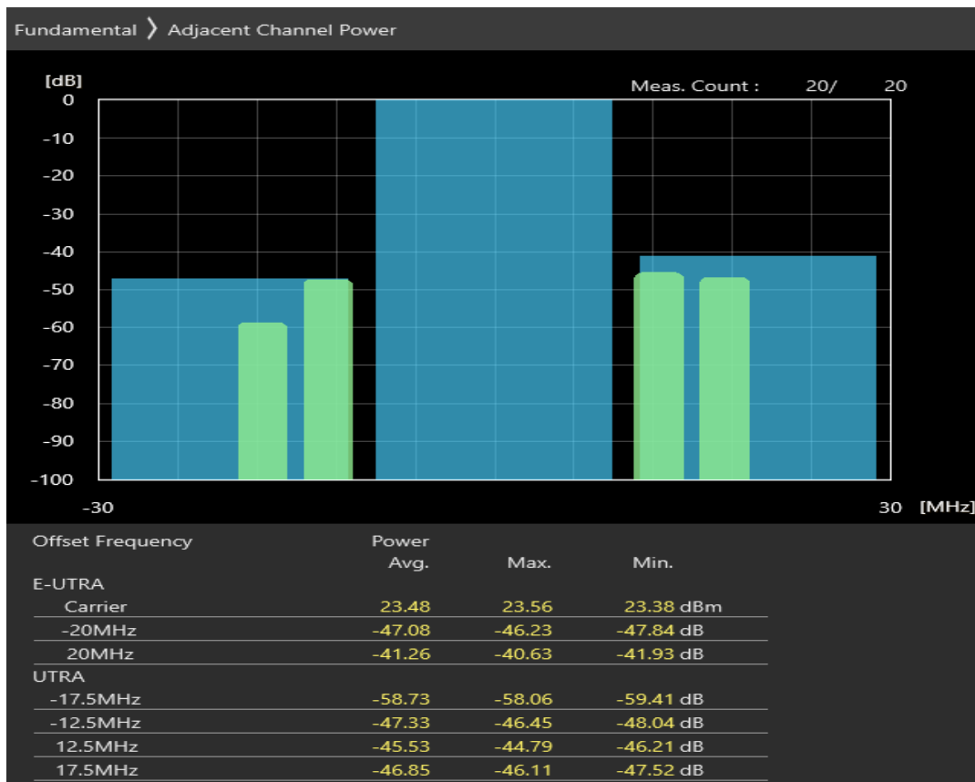
Band20 QAM16 BW=20MHz Channel=24250 RB Size=18 Position=#0
