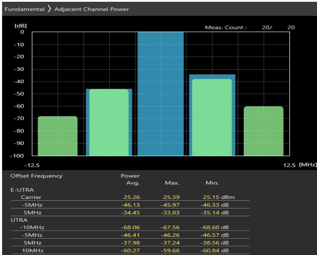
Band7 QPSK BW=5MHz Channel=20775 RB Size=25 Position=#0
