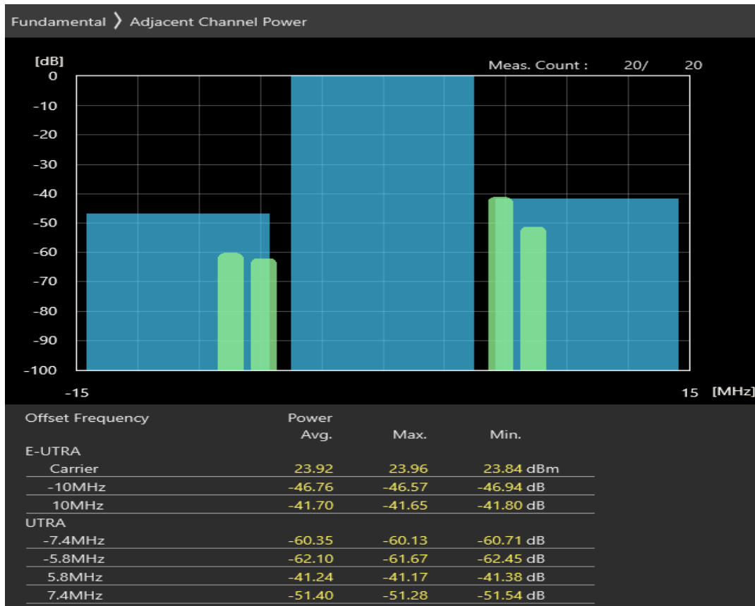
Band40 QPSK BW=10MHz Channel=39150 RB Size=50 Position=#0
