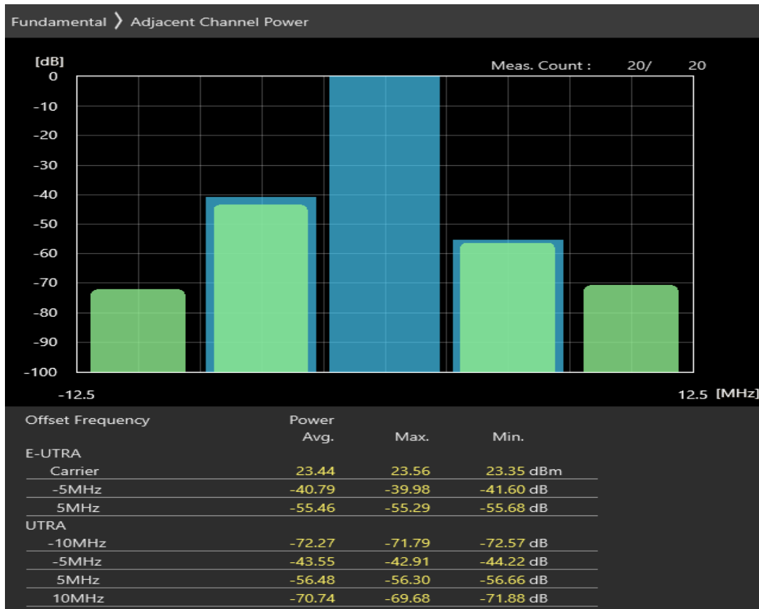
Band20 QAM16 BW=5MHz Channel=24175 RB Size=8 Position=#Max
