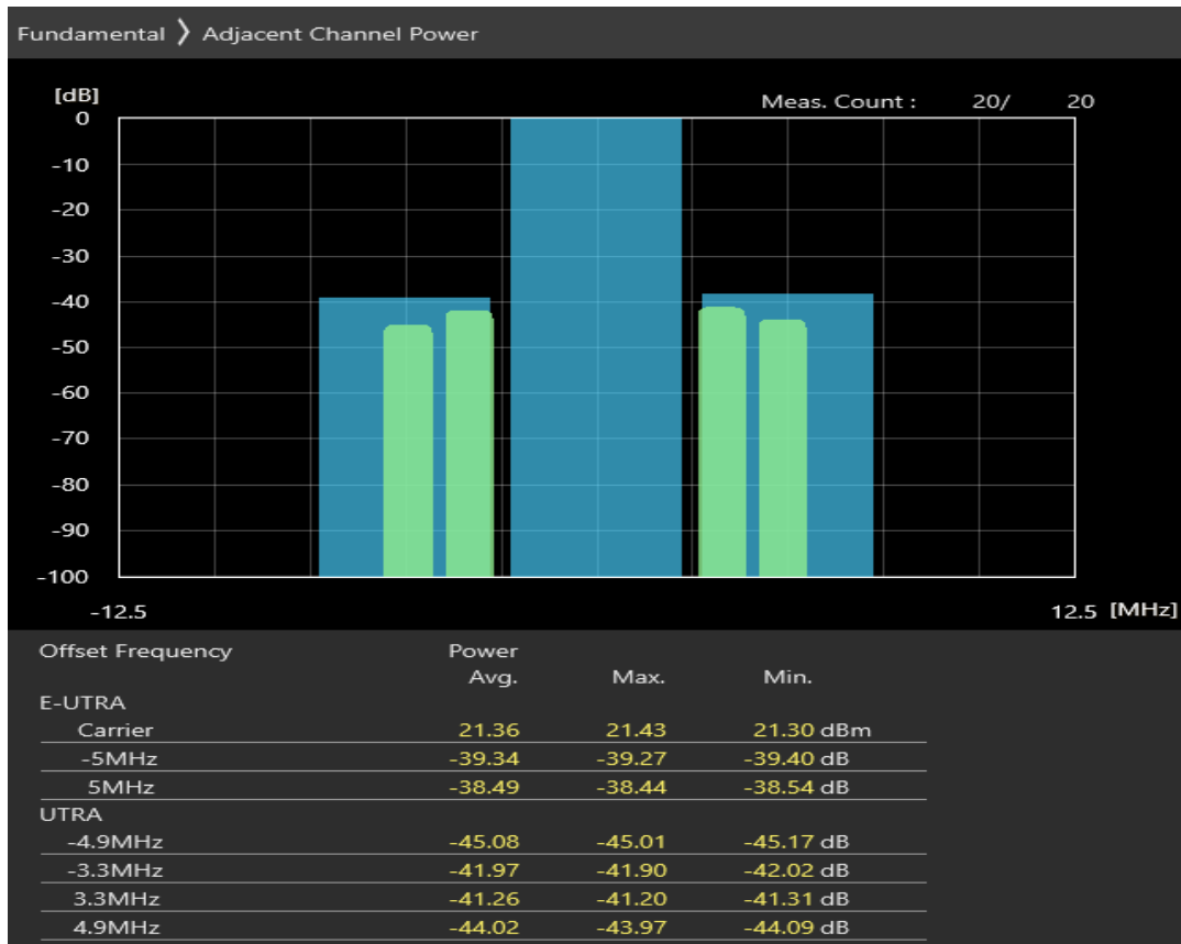
Band38 QPSK BW=5MHz Channel=38000 RB Size=8 Position=#0
