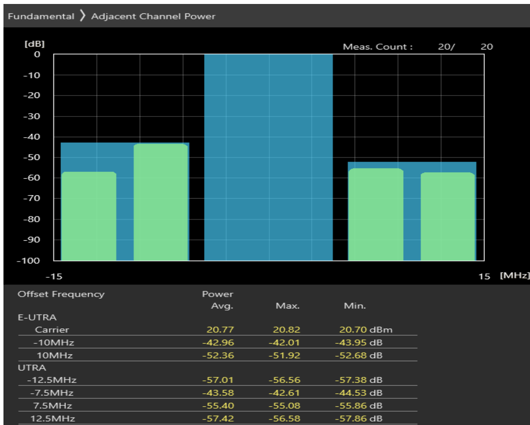
Band1 QPSK BW=10MHz Channel=18050 RB Size=12 Position=#Max
