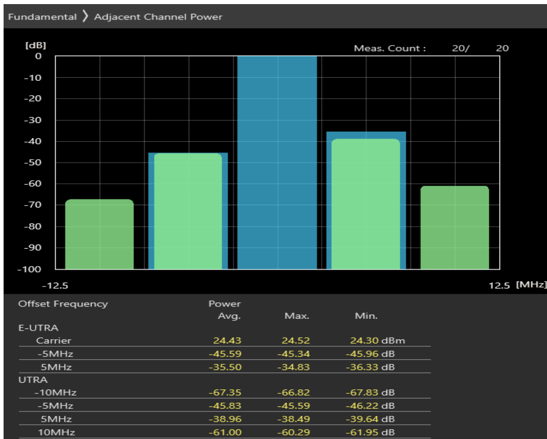
Band7 QAM16 BW=5MHz Channel=21425 RB Size=25 Position=#0
