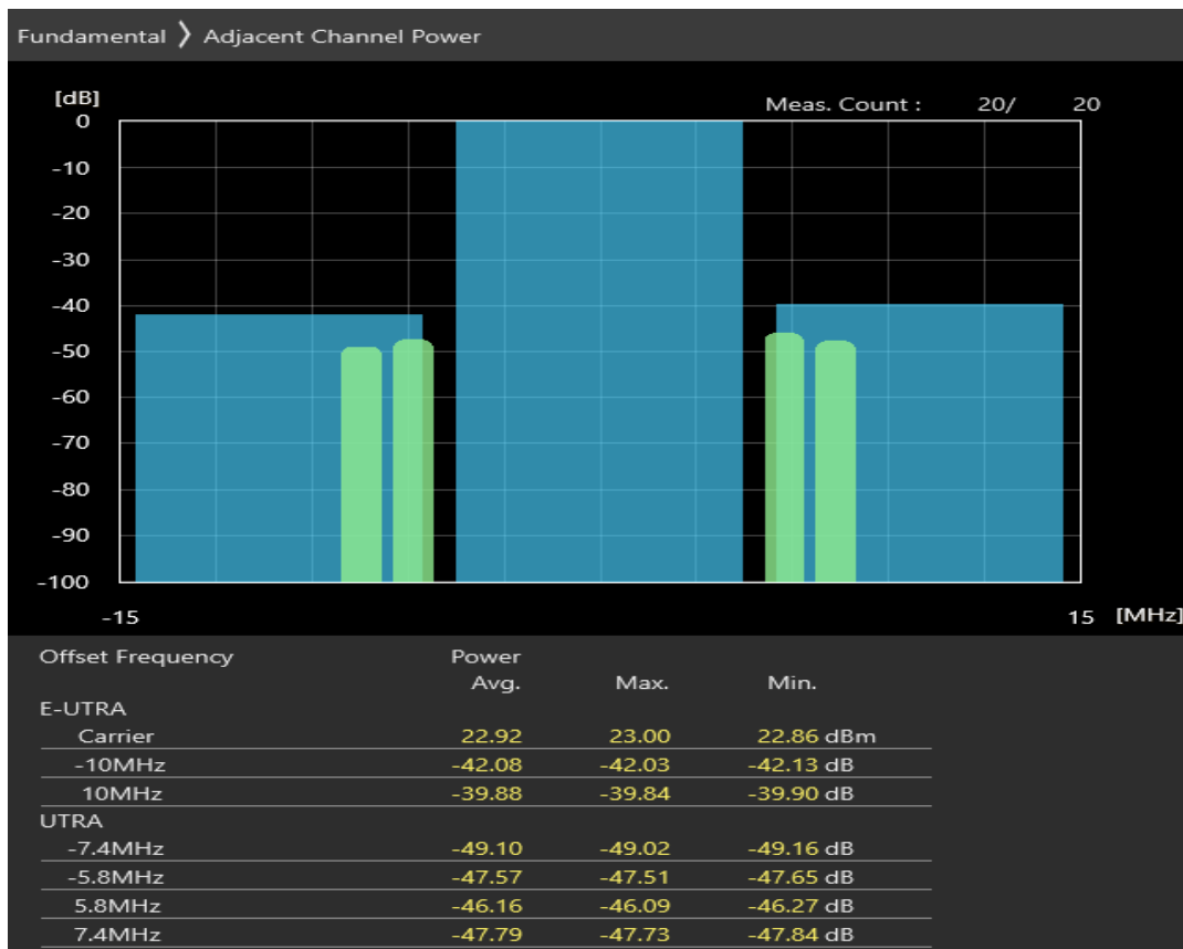
Band40 QAM16 BW=10MHz Channel=39150 RB Size=12 Position=#0
