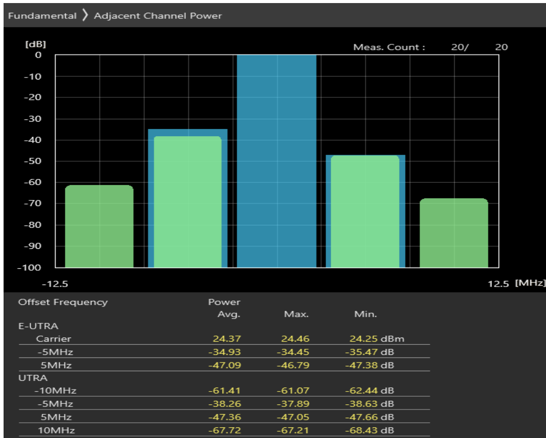
Band7 QAM16 BW=5MHz Channel=21425 RB Size=8 Position=#Max
