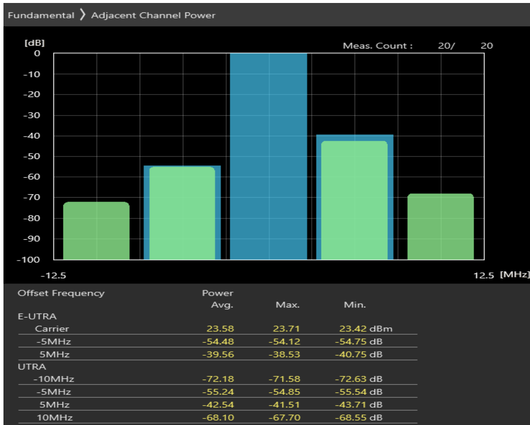
Band20 QAM16 BW=5MHz Channel=24300 RB Size=25 Position=#0
