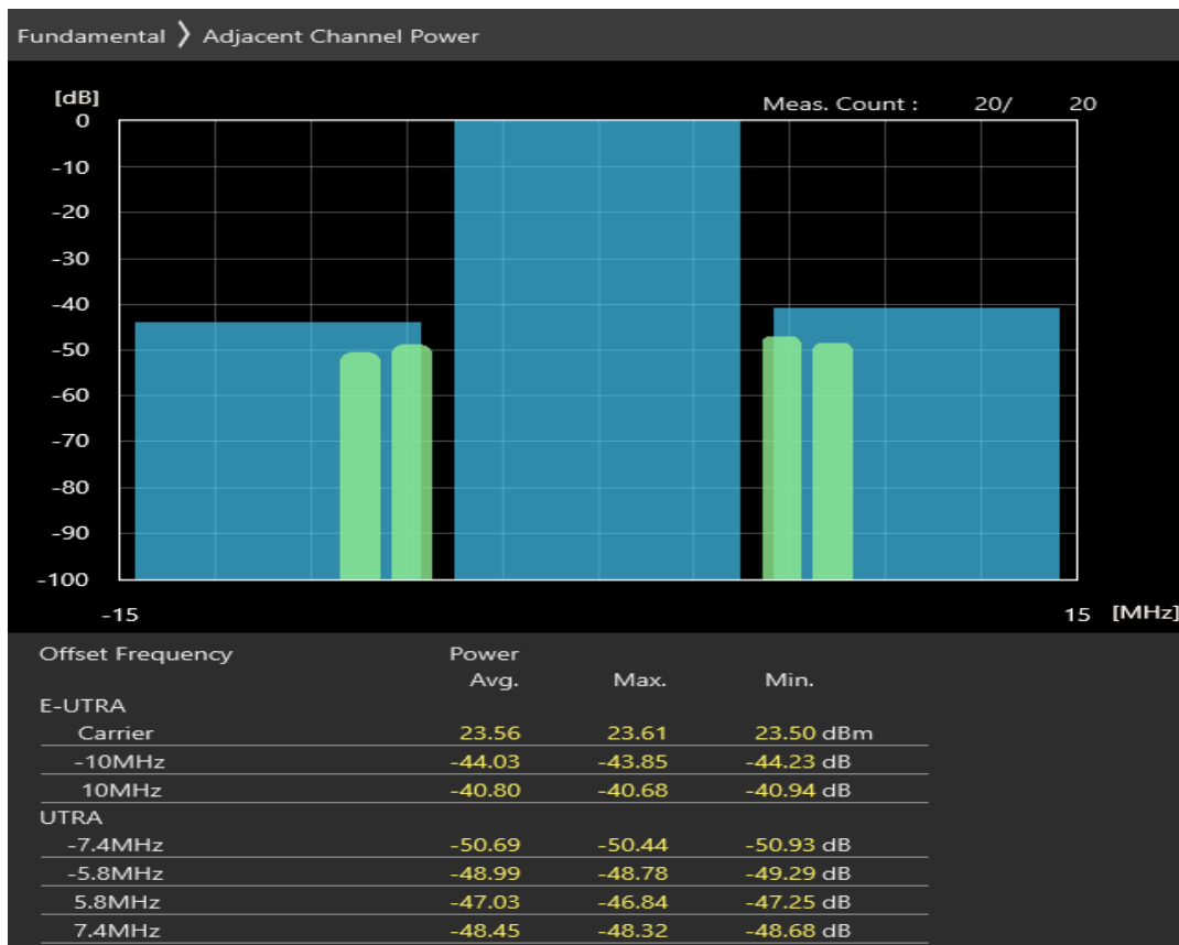
Band40 QAM16 BW=10MHz Channel=38700 RB Size=12 Position=#0
