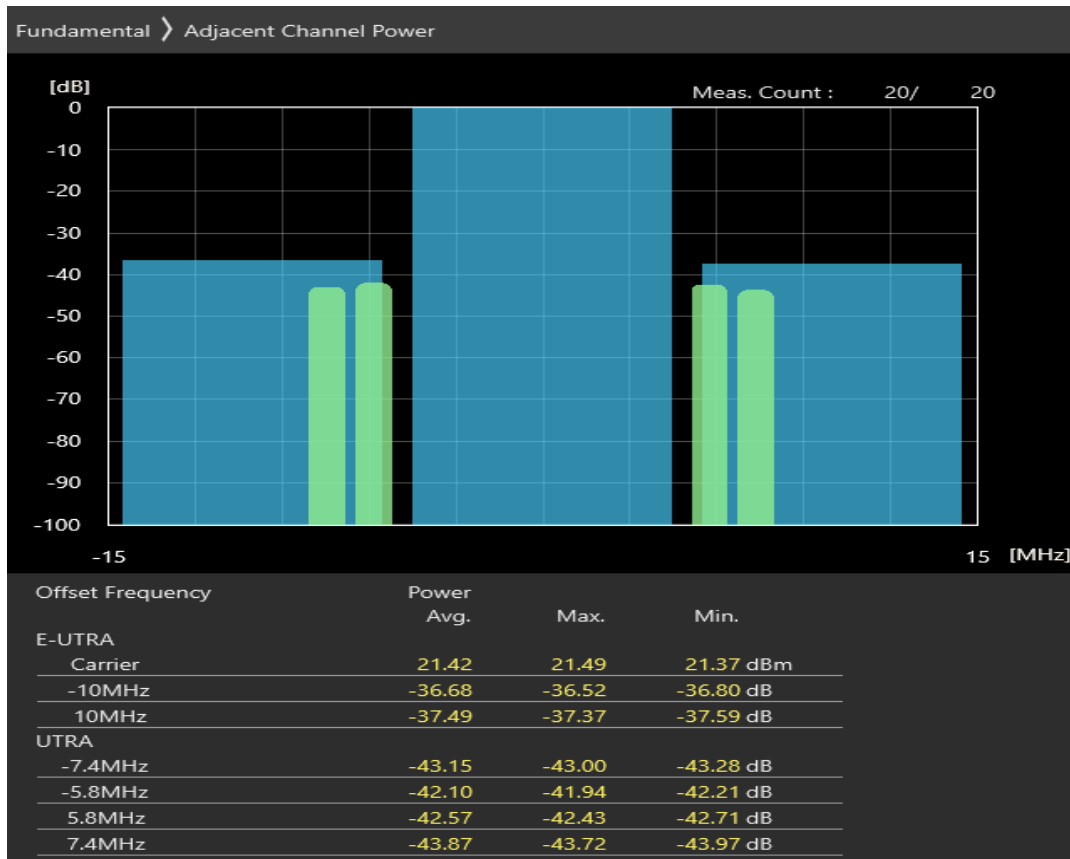
Band38 QPSK BW=10MHz Channel=38200 RB Size=12 Position=#0
