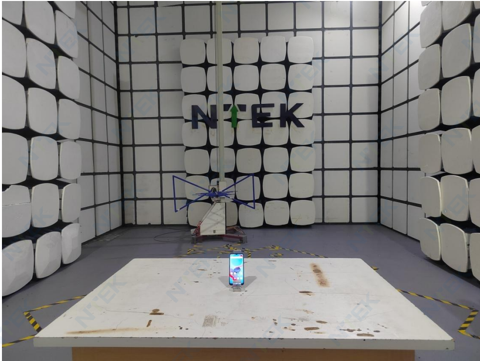
Radiated Measurement Photos(30MHz~1GHz )
