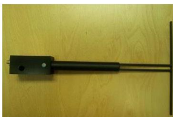
Figure 1 – MVG COMOSAR Validation Dipole
