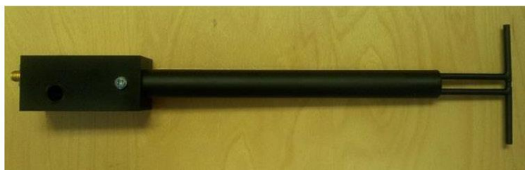
Figure 1 – MVG COMOSAR Validation Dipole
