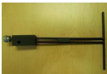
Figure 1 – MVG COMOSAR Validation Dipole
