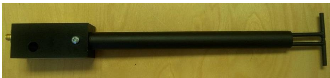
Figure 1 – MVG COMOSAR Validation Dipole
