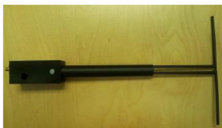
Figure 1 – MVG COMOSAR Validation Dipole
