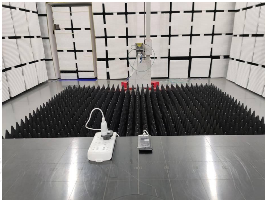
Radiated emission (1 GHz-6 GHz) test view
